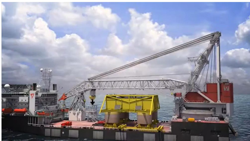
Figure 1.3-2 Subsea template at target location (Braun, 2013)
