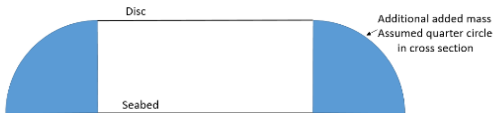
Figure 3.2-3 Representation of added mass of ring of fluid (radius R) outside a
