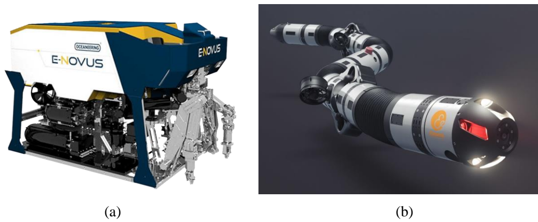
Figure 1.12 (a) Open frame ROV/AUV by Oceaneering, (b) bio-inspired multi-actuated hybrid ROV/AUV Eelume (Eelume AS, 2023).
