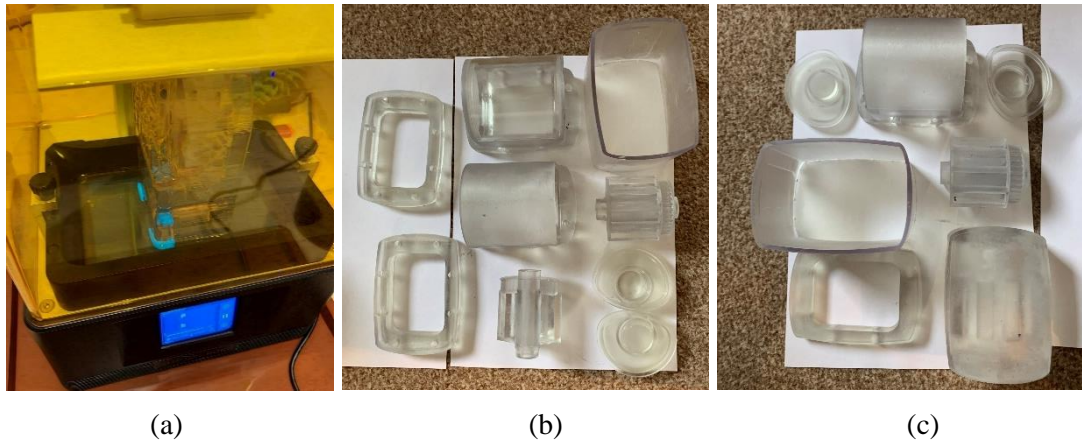
Figure 5.8 (a) SLA 3D printer and structure parts of (b) a head and (c) a body module.
