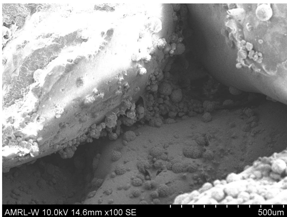
Figure 6.27 SEM images from the bottom portion of a column from Set 6: Coarse sand, NaCl inoculant amendment, submerged treatment strategy, with 9 cycles of 1 day each
