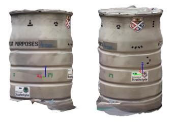
Figure 2.17: Generated 3D model produced from two-vehicle flight footage.
