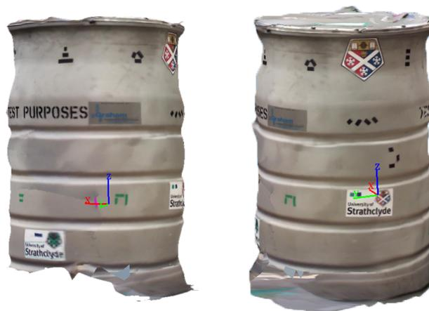
**Figure 2.17:** Generated 3D model produced from two-vehicle flight footage.
