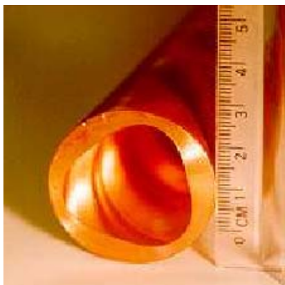
Figure 4.1 Helically corrugated waveguide.
