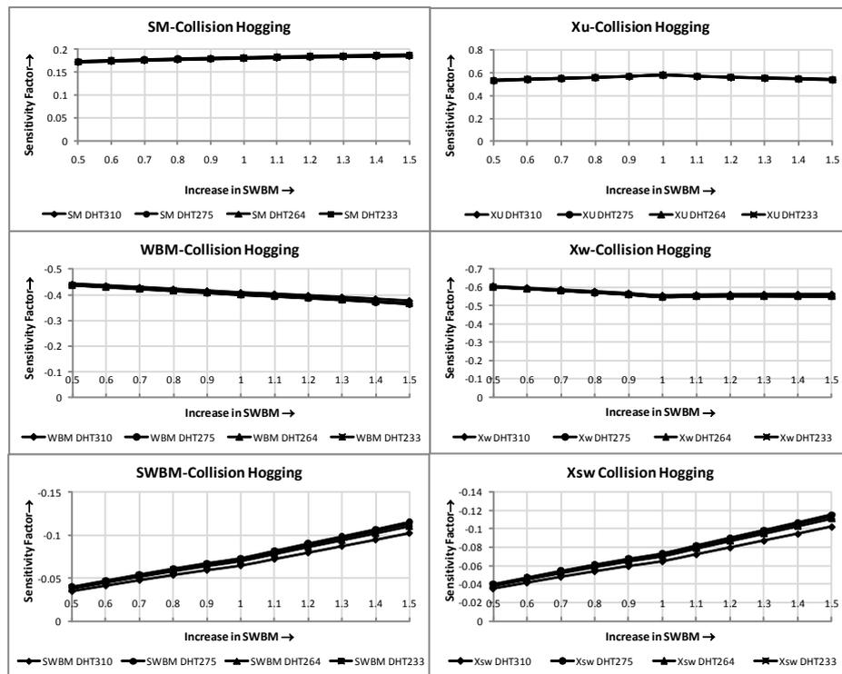
Figure 9-10 Variation of Sensitivity factor ( $\alpha$ ) for SM, WBM, Xu and Xw with increasing SWBM in hogging condition after collision
