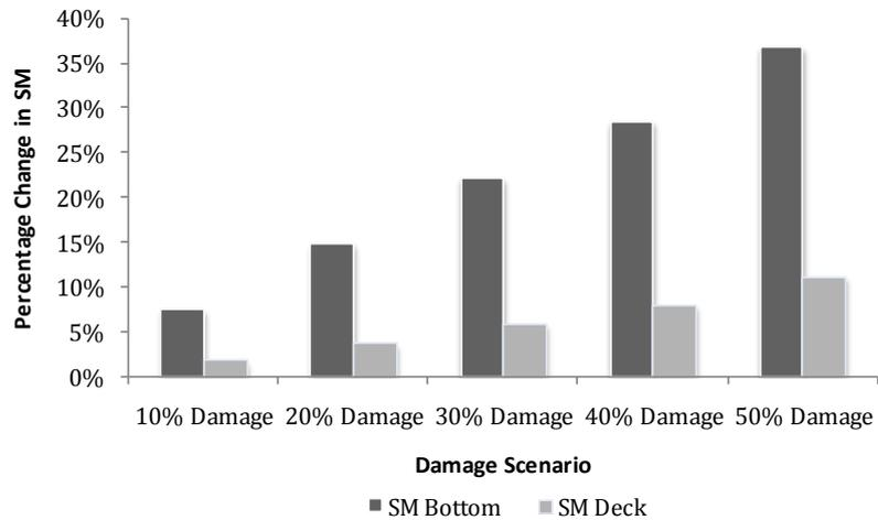
Figure 8-10 Percentage reduction in Section Modulus to deck & bottom after grounding accident
