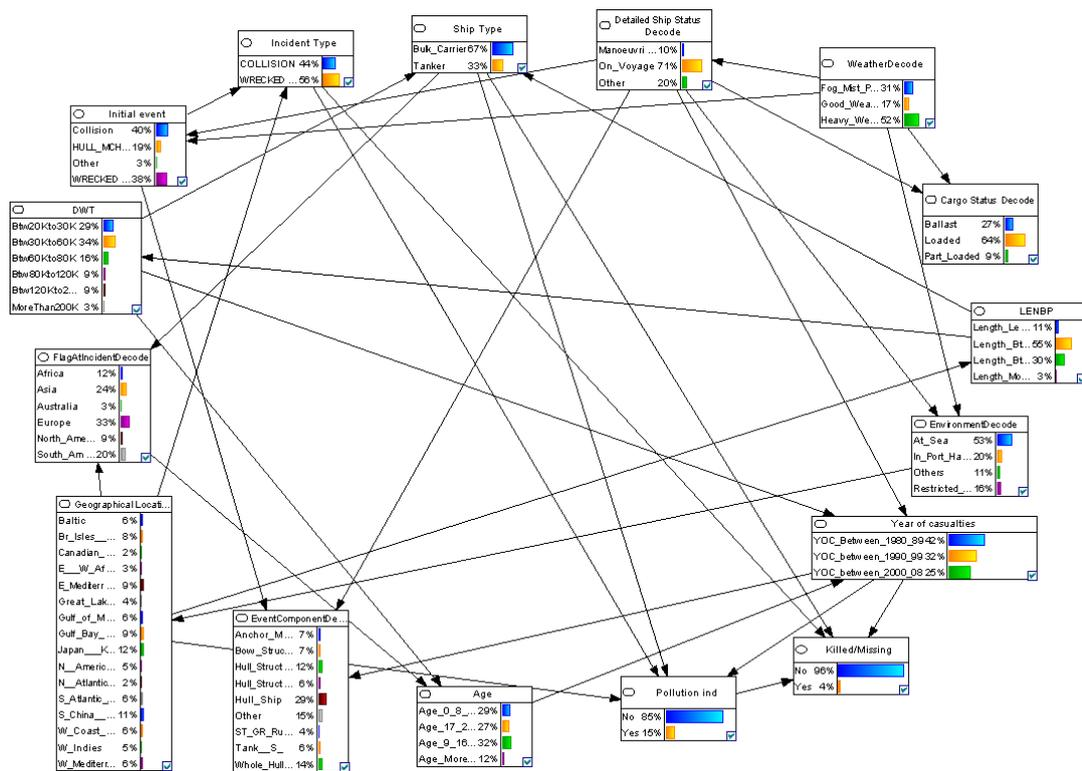
Figure 7-2 Bayesian Model of Damage Database
