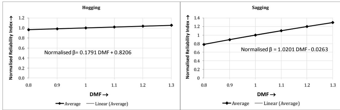
Figure 9-13 DMF versus reliability-Intact condition
