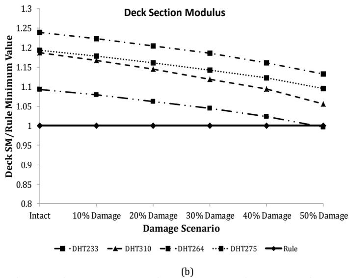
Figure 8-11 Normalised values of Section modulus to bottom and deck after damage
