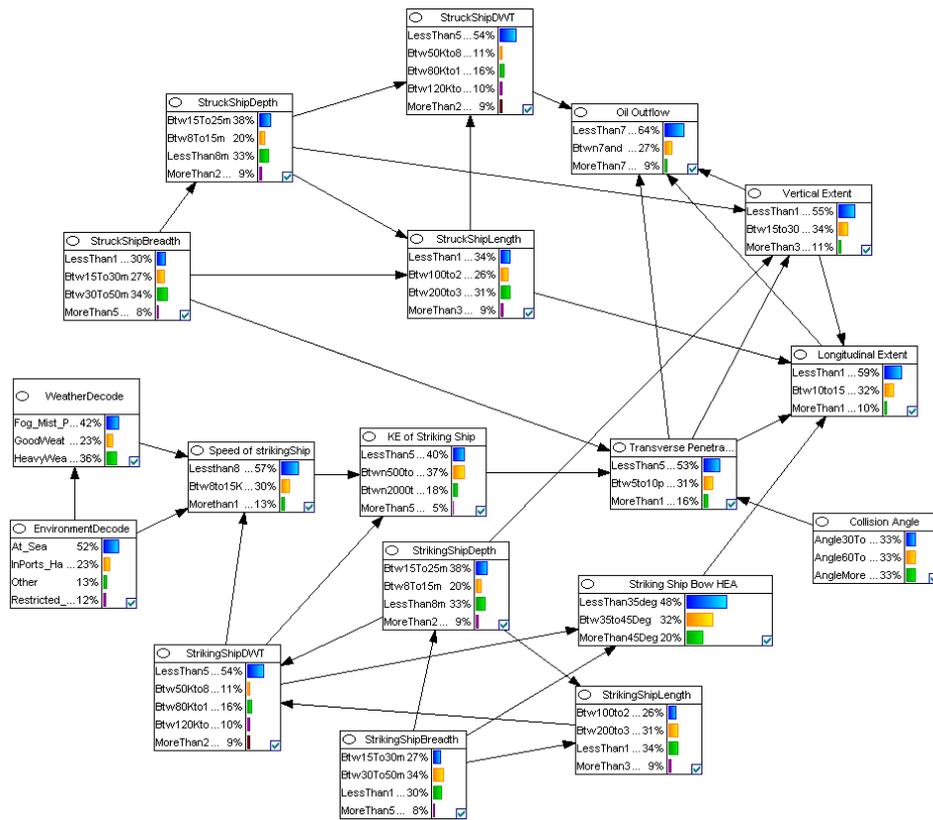
Figure 7-17 BBN Collision Model
