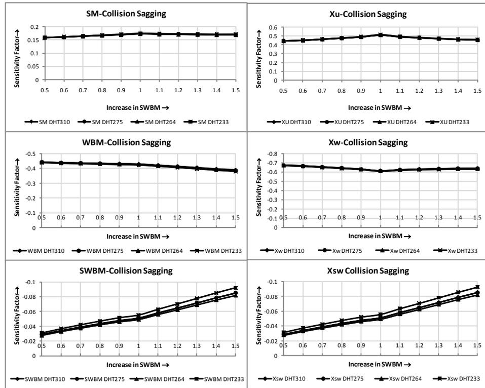
Figure 9-11 Variation of Sensitivity factor ( $\alpha$ ) for SM, WBM, Xu and Xw with increasing SWBM in sagging condition after Collision
