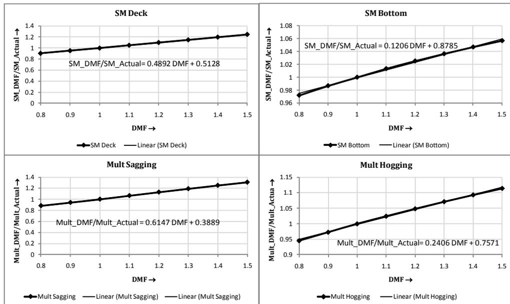
Figure 8-24 DMF versus Section and Ultimate strength
