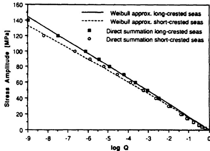
Figure 3-5 Long term distribution of deck stresses resulting from WVBM (Frieze et al., 1991)
