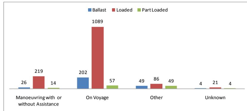
Figure 5-24 Distribution of operating condition of ship and cargo status at the time of accident
