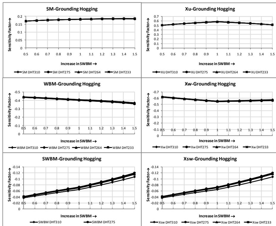
Figure 9-8 Variation of Sensitivity factor ( $\alpha$ ) for SM, WBM, Xu and Xw with increasing SWBM in hogging condition after grounding
