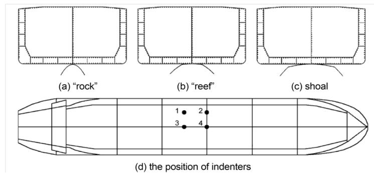
Figure 3-2 Three indenter topologies and position Alsos *et al* (2007)
