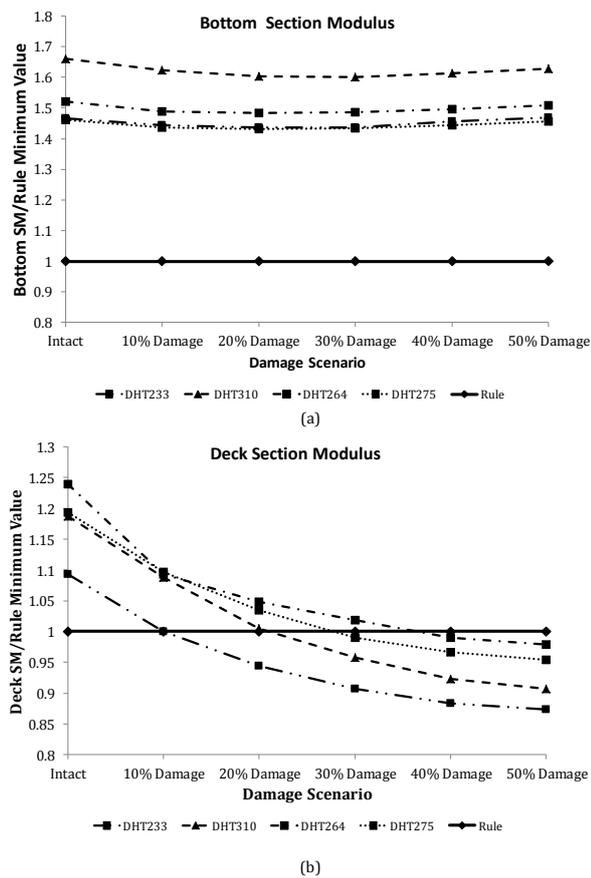
Figure 8-18 Normalised values of Section Modulus after side damage to the (a) Bottom and (b) Deck
