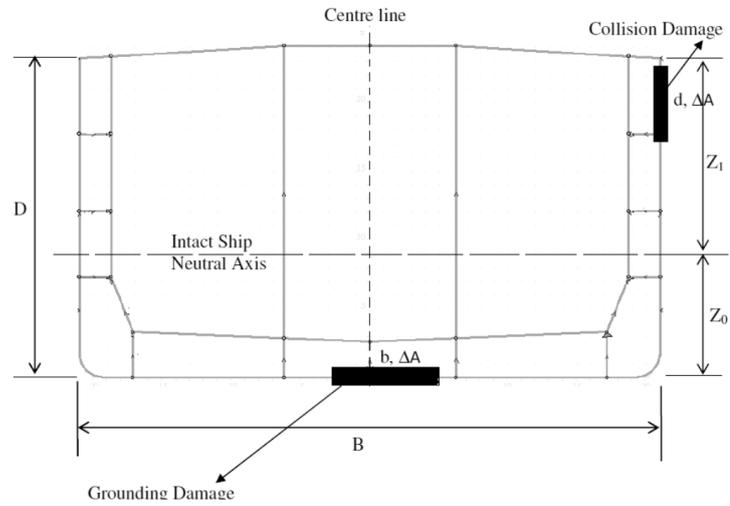
Figure 8-7 Illustration of Damage Extent in ship mid-ship section
