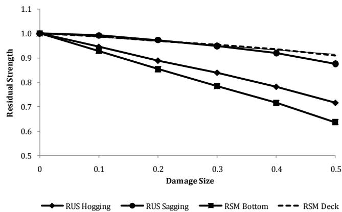
Figure 8-14 Residual Strength of ships with grounding damage
