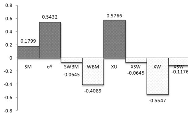
Figure 9-7 Sensitivity factor ( $\alpha$ ) of ships in intact condition
