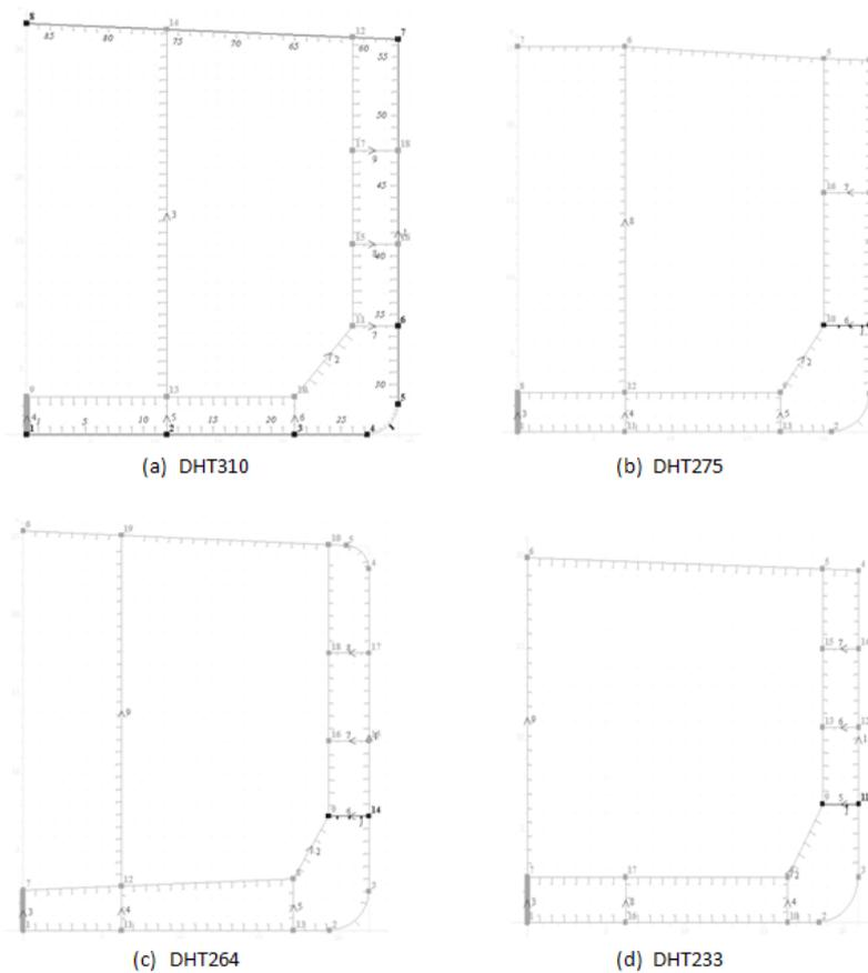
Figure 8-6 Mid-ship cross of sample ships
