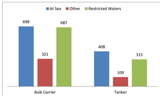
Figure 5-22 Distribution of accidents on different ship types at various locations
