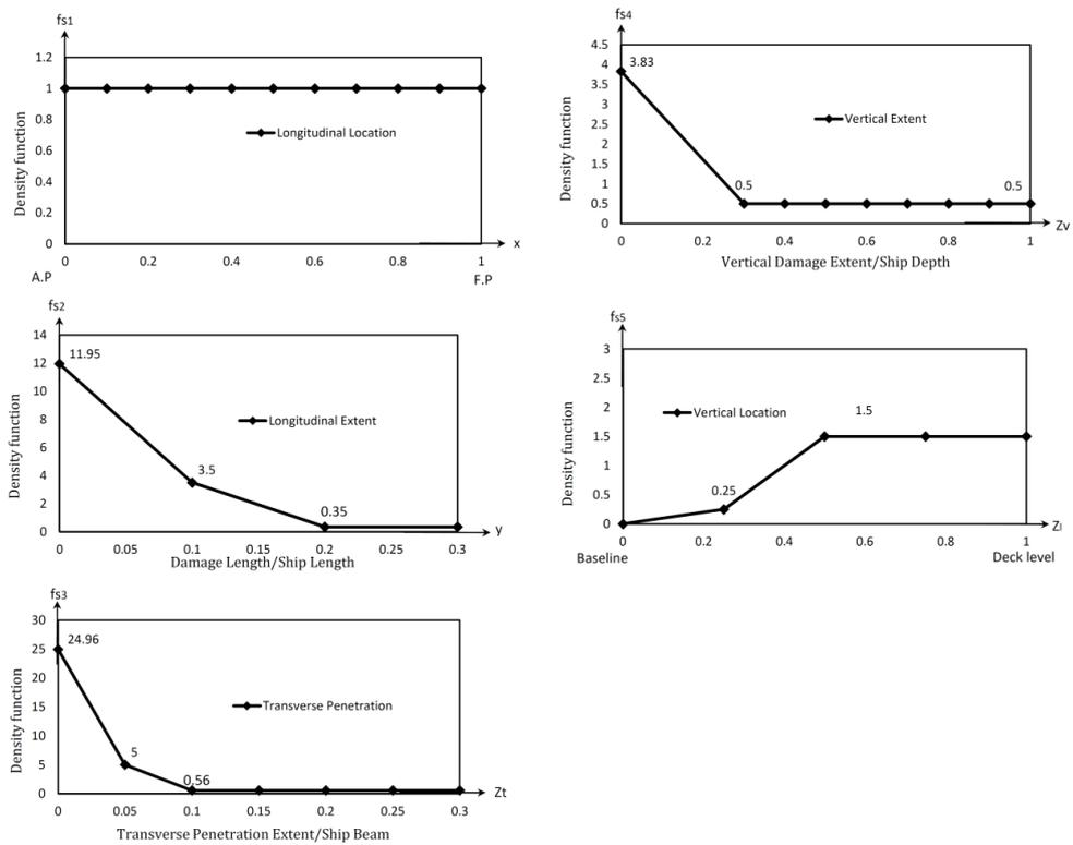
Figure 5-36 Side damage due to collision: density functions  $f_{s1}$ ,  $f_{s2}$ ,  $f_{s3}$ ,  $f_{s4}$  and  $f_{s5}$
