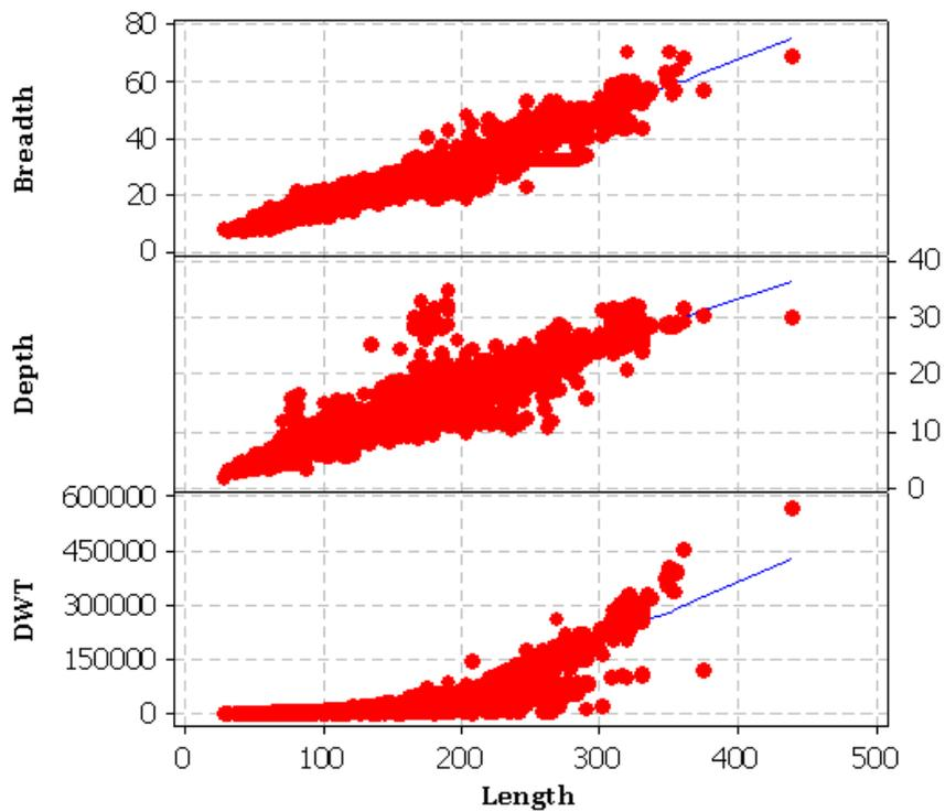
Figure 5-12 Distribution of Length of ships vs. (a) Displacement (b) Depth (c) Breadth
