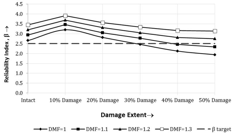
Figure 9-14 Reliability of strengthened section in damaged condition
