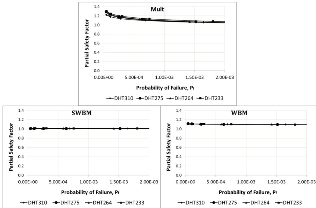
Figure 9-12 Partial safety factor as a function of target reliability level
