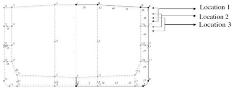
Figure 8-16 Vertical Location of accident
