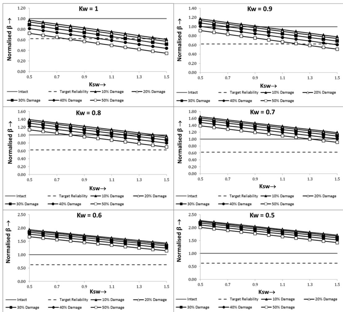
Figure 9-4 Variation of Reliability index under different combinations of  $K_{sw}$  and  $K_w$  in Sagging following a grounding accident.
