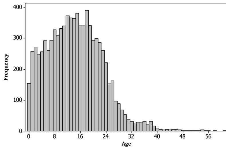
Figure 5-13 Age of ship at the time of accident
