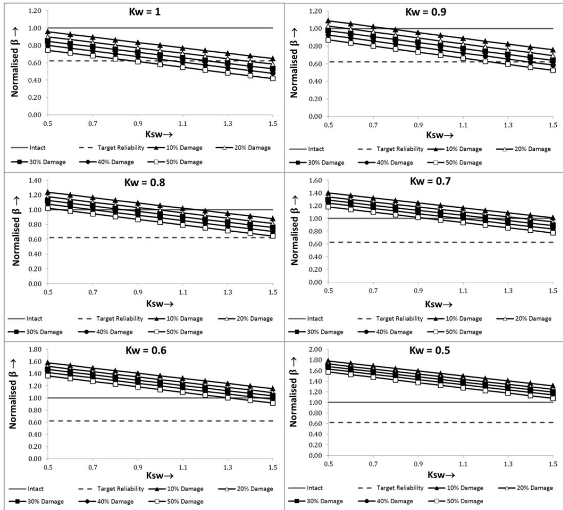
Figure 9-5 Variation of Reliability index under different combinations of  $K_{sw}$  and  $K_w$  in hogging following a collision accident.
