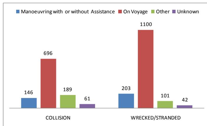
Figure 5-16 Distribution of Ship operating condition at the time of accident
