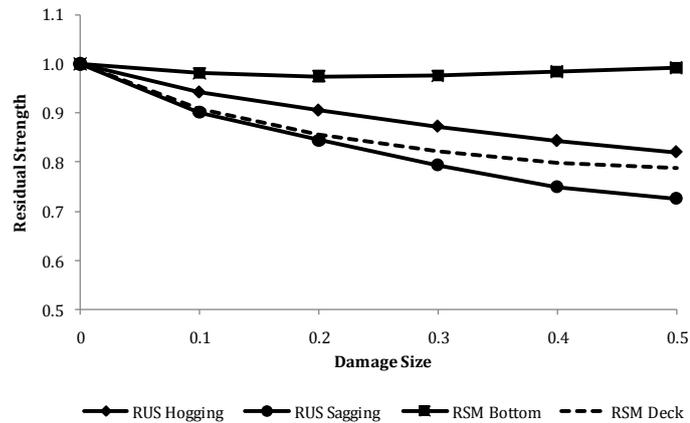
Figure 8-22 Residual Strength of ships with collision damage
