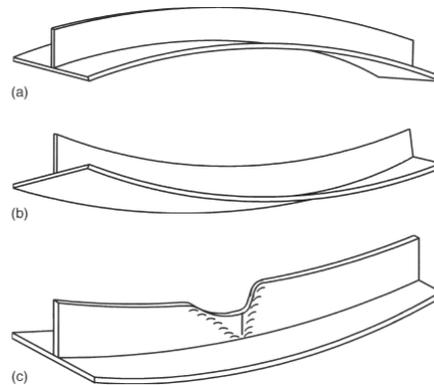
Figure 8-4 Possible collapse modes of stiffened panels under compressive loads. (a) Plate induced collapse; (b) Stiffener induced collapse, (c) Tripping failure
