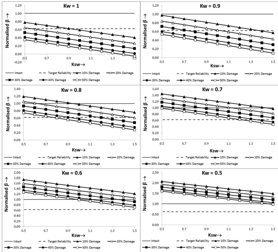
Figure 9-6 Variation of Reliability index under different combinations of Ksw and Kw in sagging following a collision accident.
