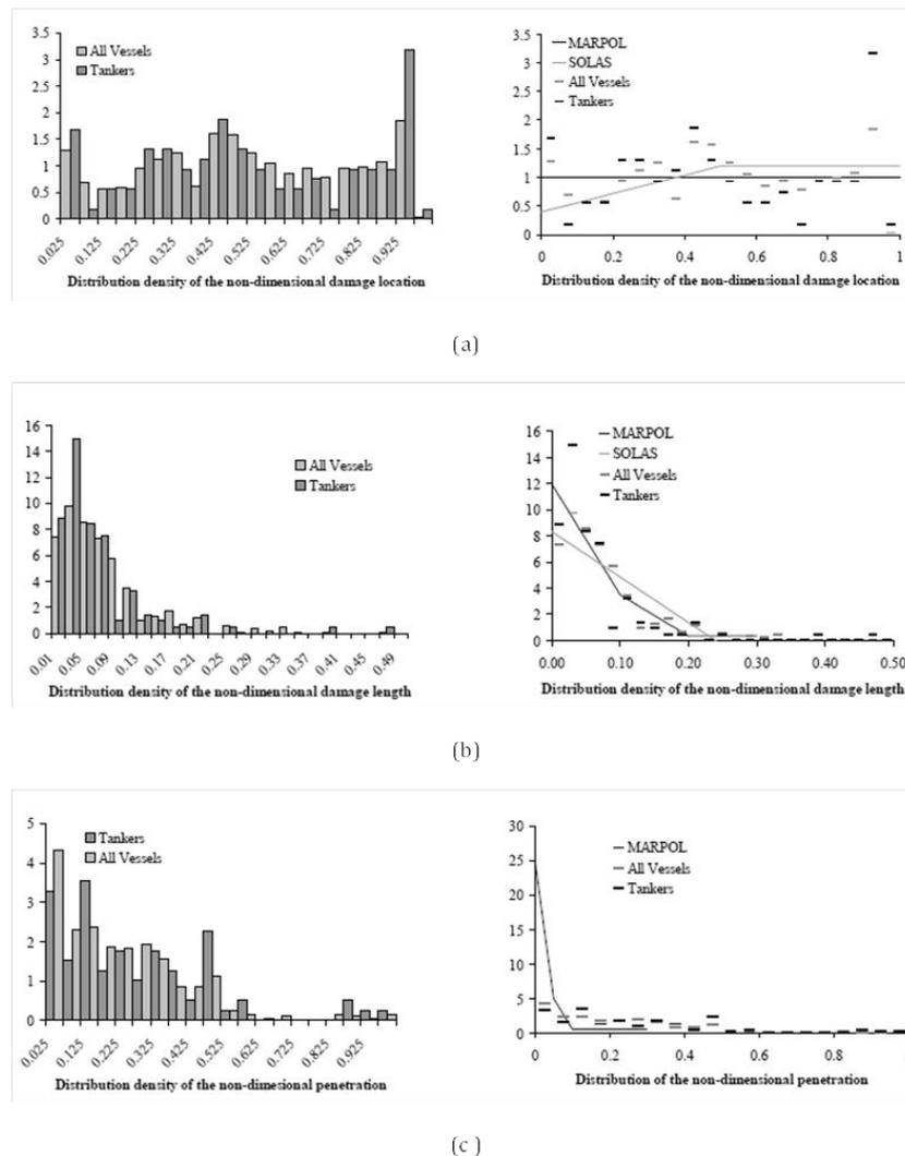
Figure 5-38 The distribution density for (a) the non-dimensional damage location (b) the non-dimensional damage length (c) the non-dimensional damage penetration . Both data and regulation are compared for tankers and all vessels
