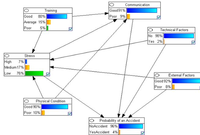
Figure 7-12 Bayesian Network for Cause of Ship Accidents
