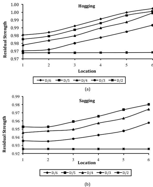
Figure 8-17 Residual Strength after side damage at different locations (a) Hogging (b) Sagging
