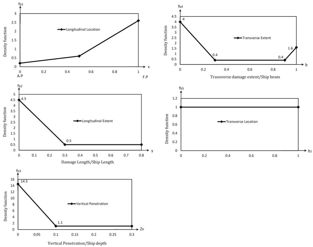
Figure 5-35 Bottom damage due to grounding: density functions  $f_{b1}$ ,  $f_{b2}$ ,  $f_{b3}$ ,  $f_{b4}$  and  $f_{b5}$
