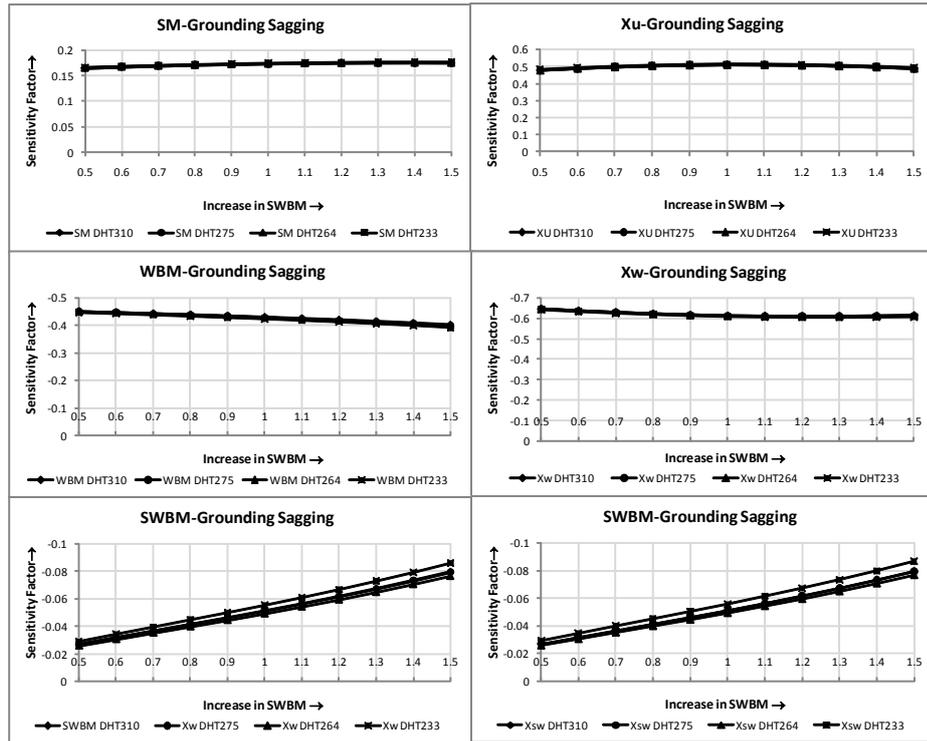
Figure 9-9 Variation of Sensitivity factor ( $\alpha$ ) for SM, WBM, Xu and Xw with increasing SWBM in sagging condition after grounding
