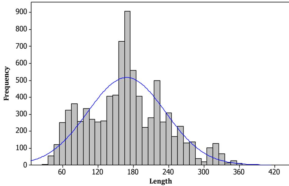
Figure 5-11 Histogram of Length of ship met with accidents
