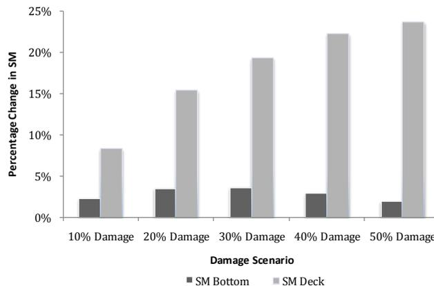
Figure 8-19 Percentage reduction in Section Modulus to deck & bottom after collision accident
