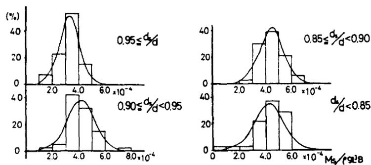
Figure 3-3 Distribution of still water bending moment of container ships (Mano et al., 1977)
