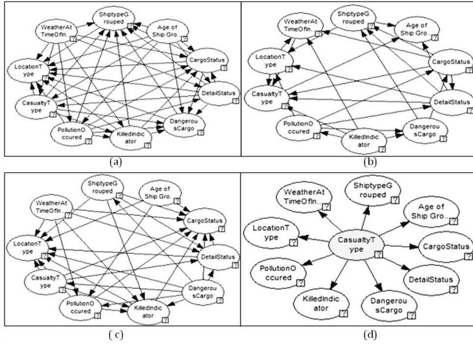
Figure 6-2 Structure of Probabilistic Network Model Using (a) PC Method (b) Greedy Search (c) Essential Search (d) Naïve Classifier
