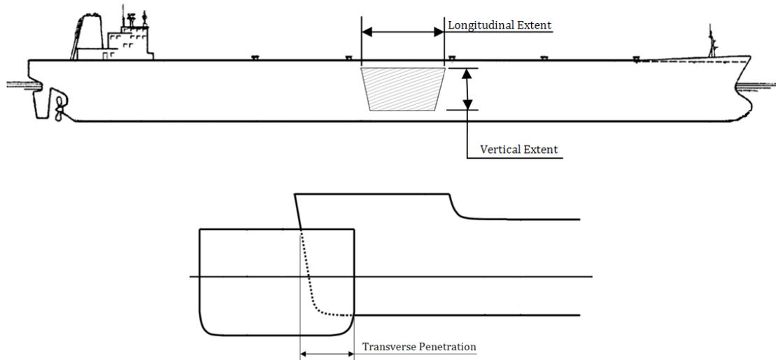
Figure 7-15 Description of Damage Extent in collision
