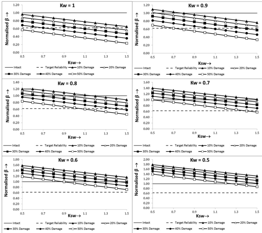
Figure 9-3 Variation of Reliability index under different combinations of  $K_{sw}$  and  $K_w$  in hogging following a grounding accident.
