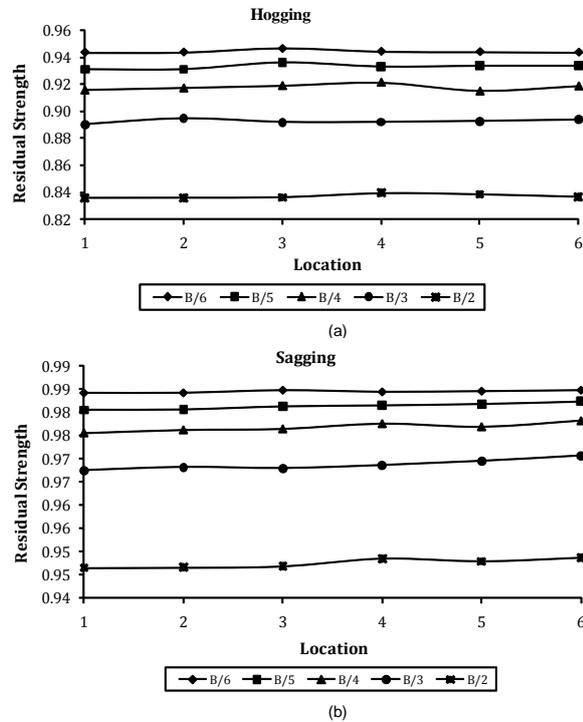
Figure 8-9 Residual Strength after bottom damage at different locations (a) Hogging (b) Sagging
