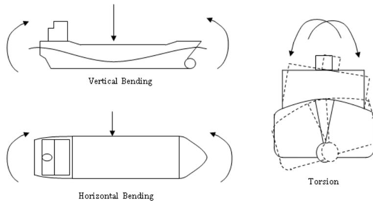
Figure 8-1 Types of Hull Bending
