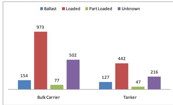
Figure 5-21 Distribution of Cargo statuses of ships at the time of accident
