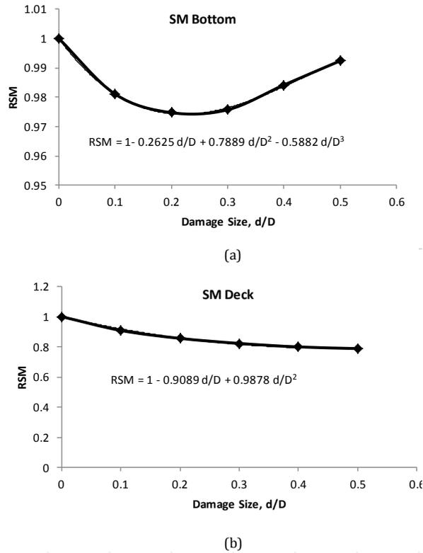
Figure 8-20 RSM formula for (a) loss in SM of Bottom (b) loss in SM of Deck
