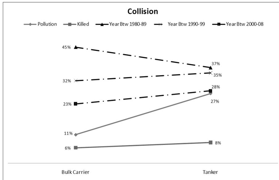
Figure 7-4 The variations of probability of Pollution, Killed, Year of Accident given Ship Type
