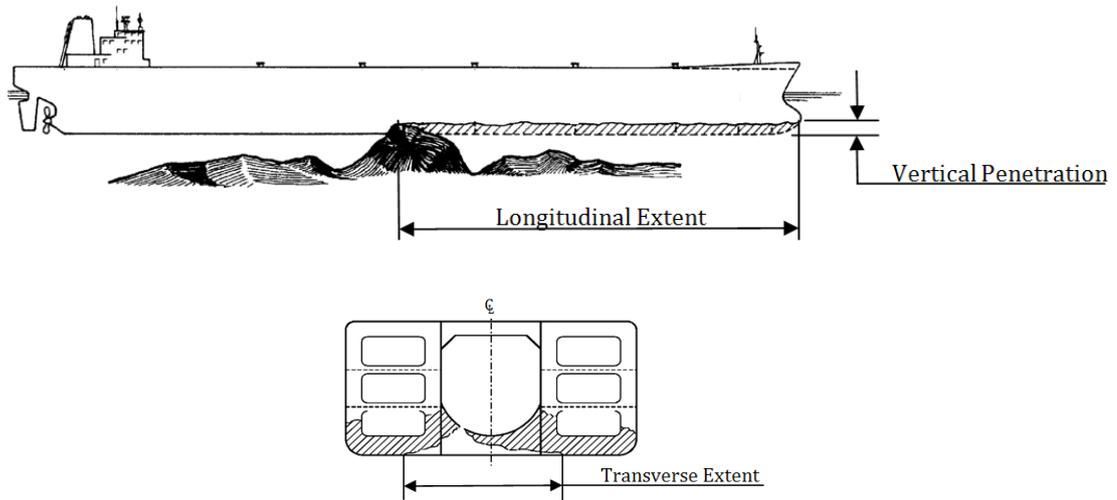
Figure 7-14 Description of Damage Extent in grounding
