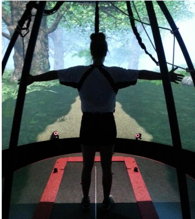
Figure 10. Photograph of subject during calibration, prior to initiation of walking. The forest walk projection can be observed along with split belt and safety harness set up.
