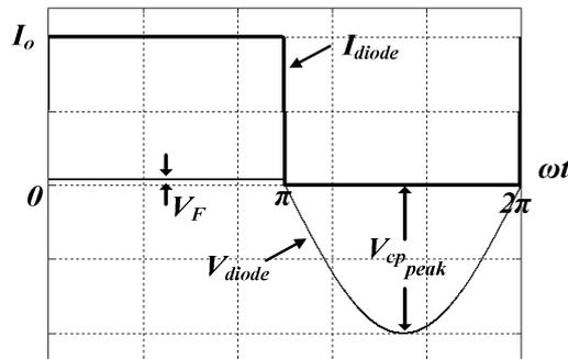
Fig. 3.10: SPRC rectifier diode voltage/current waveforms
