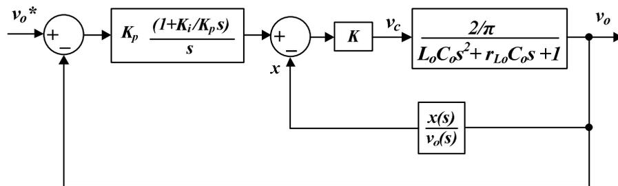
Fig. 4.26: Generalized transfer function block diagram for the multi-loop control system
