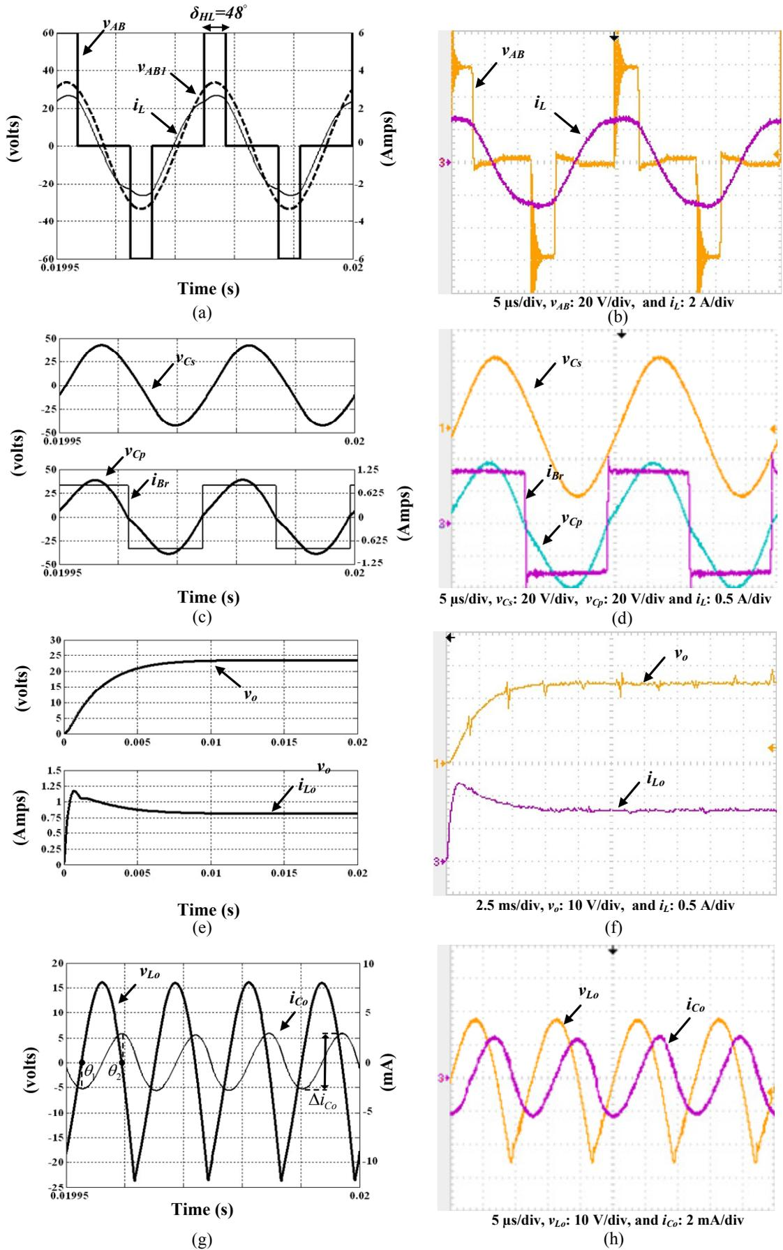
Fig. 3.22: Half-load operation results (a),(c),(e)&(g) Simulation, and (b),(d),(f)&(h) Experimental.
