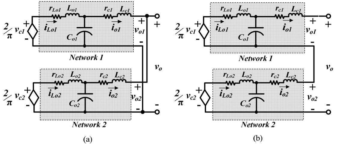
Fig. 6.5: Equivalent control circuit diagrams for (a) ISOP and (b) ISOS systems.
