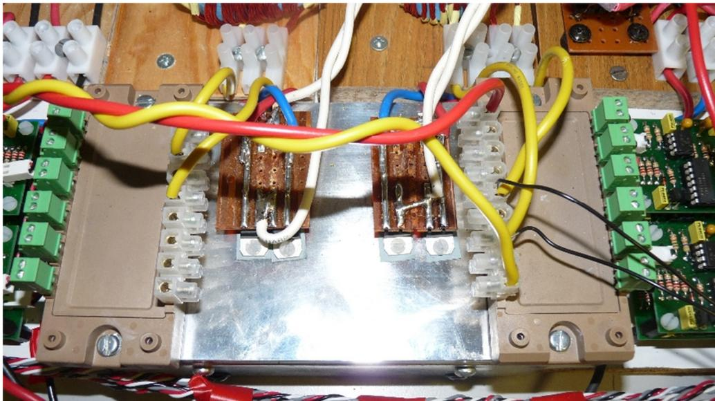
Fig. A.11: Module power inverters mounted on heat sink
