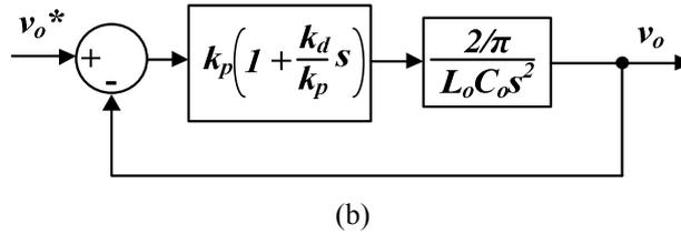
Fig. 5.3: Closed-loop system with Lyapunov controller
