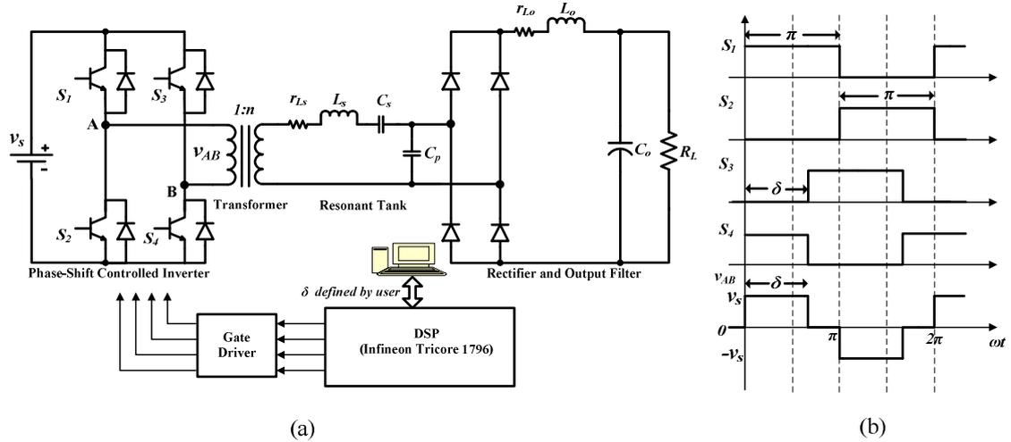
Fig. 3.20: Experimental prototype (a) circuit diagram and (b) inverter phase control gating pattern.
