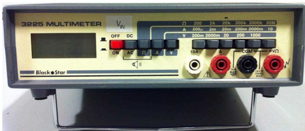
Fig. A.19: Multimeter for circuit current and voltage monitoring
