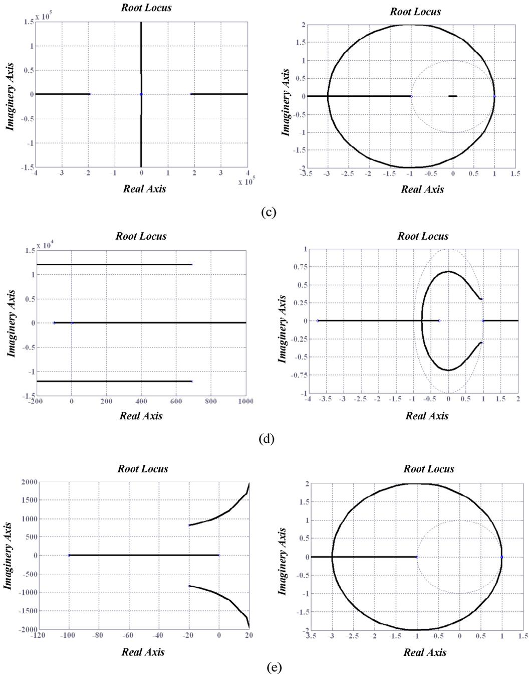
Fig. 4.28: Root loci of multi-loop control system with the inner control loop state variable being (a)  $i_{Ld}$ , (b)  $i_{Lq}$ , (c)  $v_{Csd}$ , (d)  $v_{Csq}$ , and (e)  $v_{Cpd}$ .
