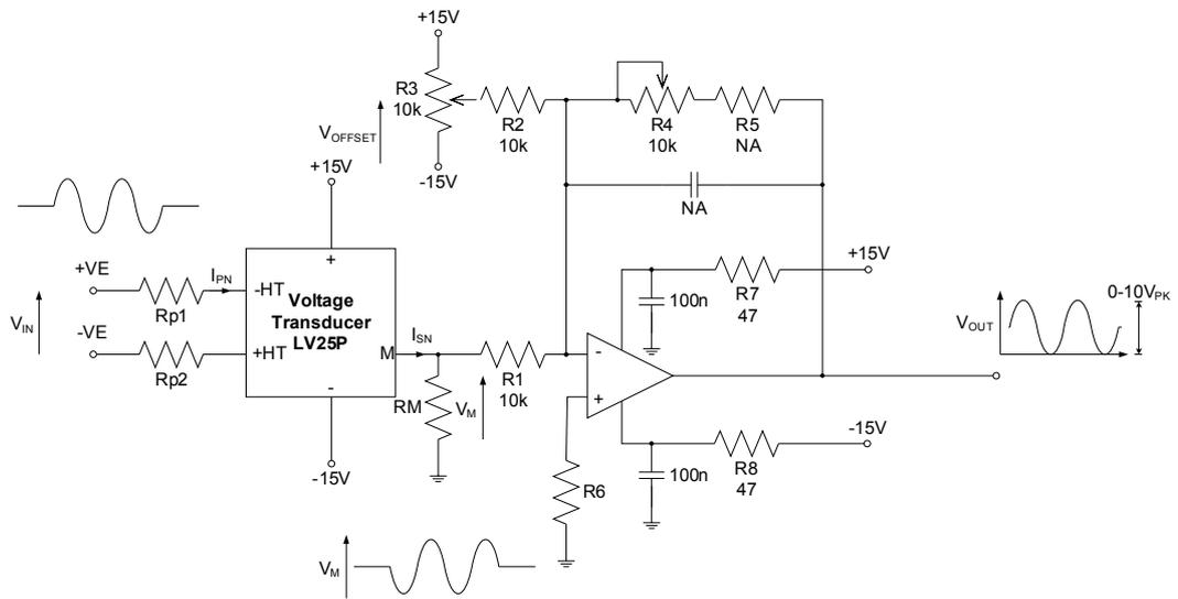
Fig. A.6: Voltage transducer circuit diagram
