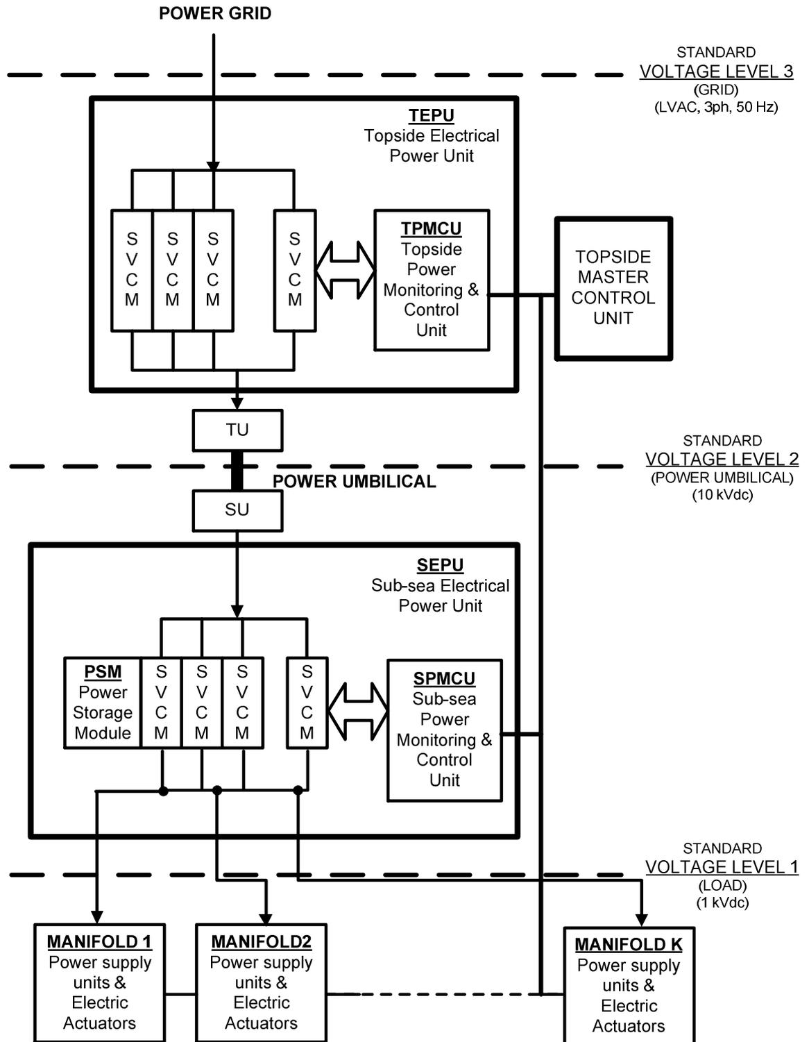
Fig. 1.7: Layout of the fully modular power distribution system architecture for subsea applications.
