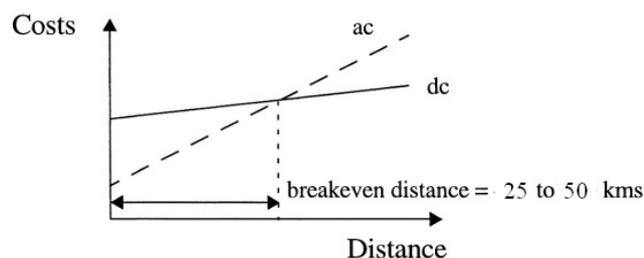
Fig. 1.2: Cost comparison for subsea cables operating with ac versus dc transmission.
