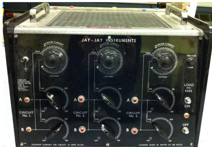
Fig. A.16: Resistive load
