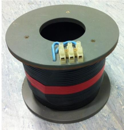
Fig. A.15: Cable impedance emulator
