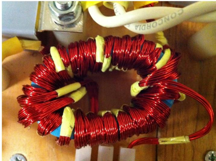
Fig. A.12: Nano-crystalline core transformer
