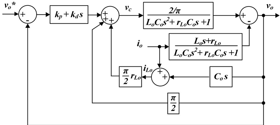
Fig. 5.9: Closed-loop system structure with Lyapunov controller.
