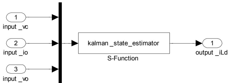
Fig. C.1: Kalman filter state estimator as an s-function in Simulink
