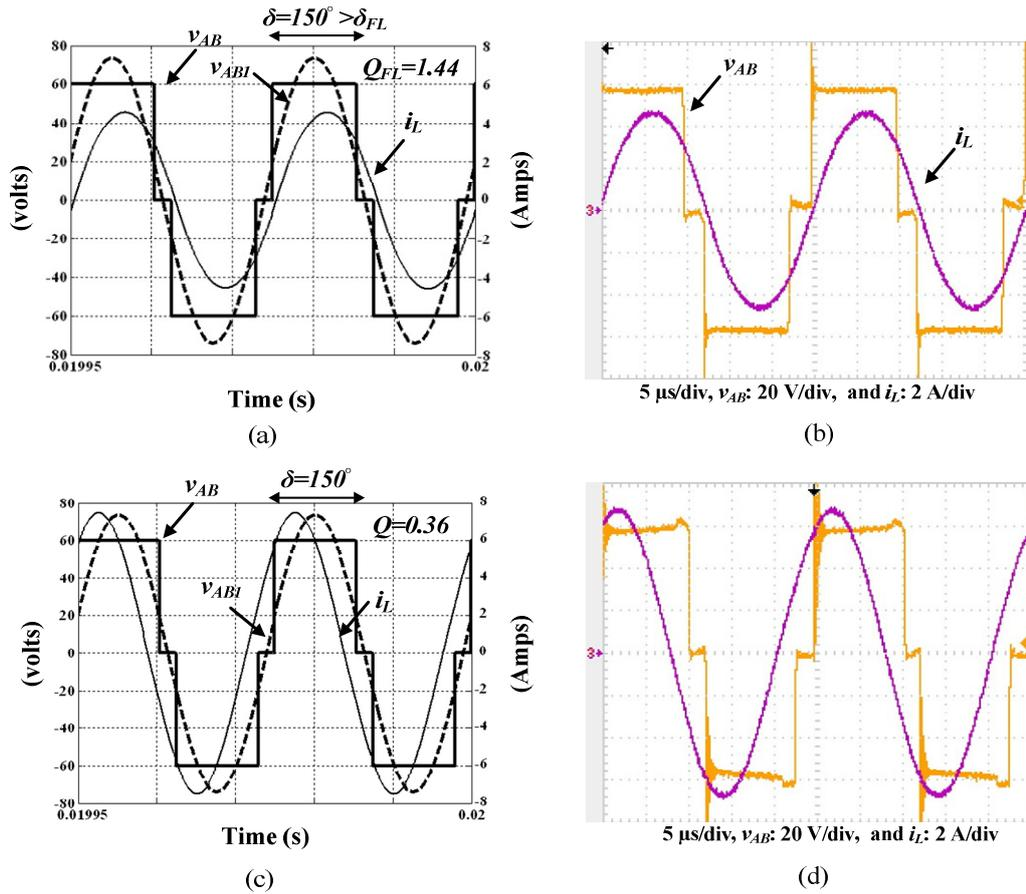
Fig. 3.23: Mode 1 and mode 3 operation results (a)&(c) Simulation, and (b)&(d) Experimental.
