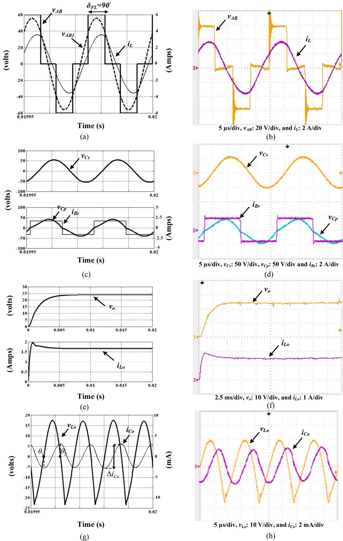
Fig. 3.21: Full-load operation results (a),(c),(e)&(g) Simulation, and (b),(d),(f)&(h) Experimental.
