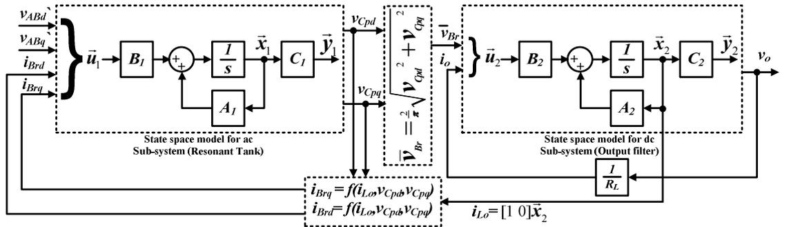
Fig. 4.5: Non-linear combined system model for the SPRC.
