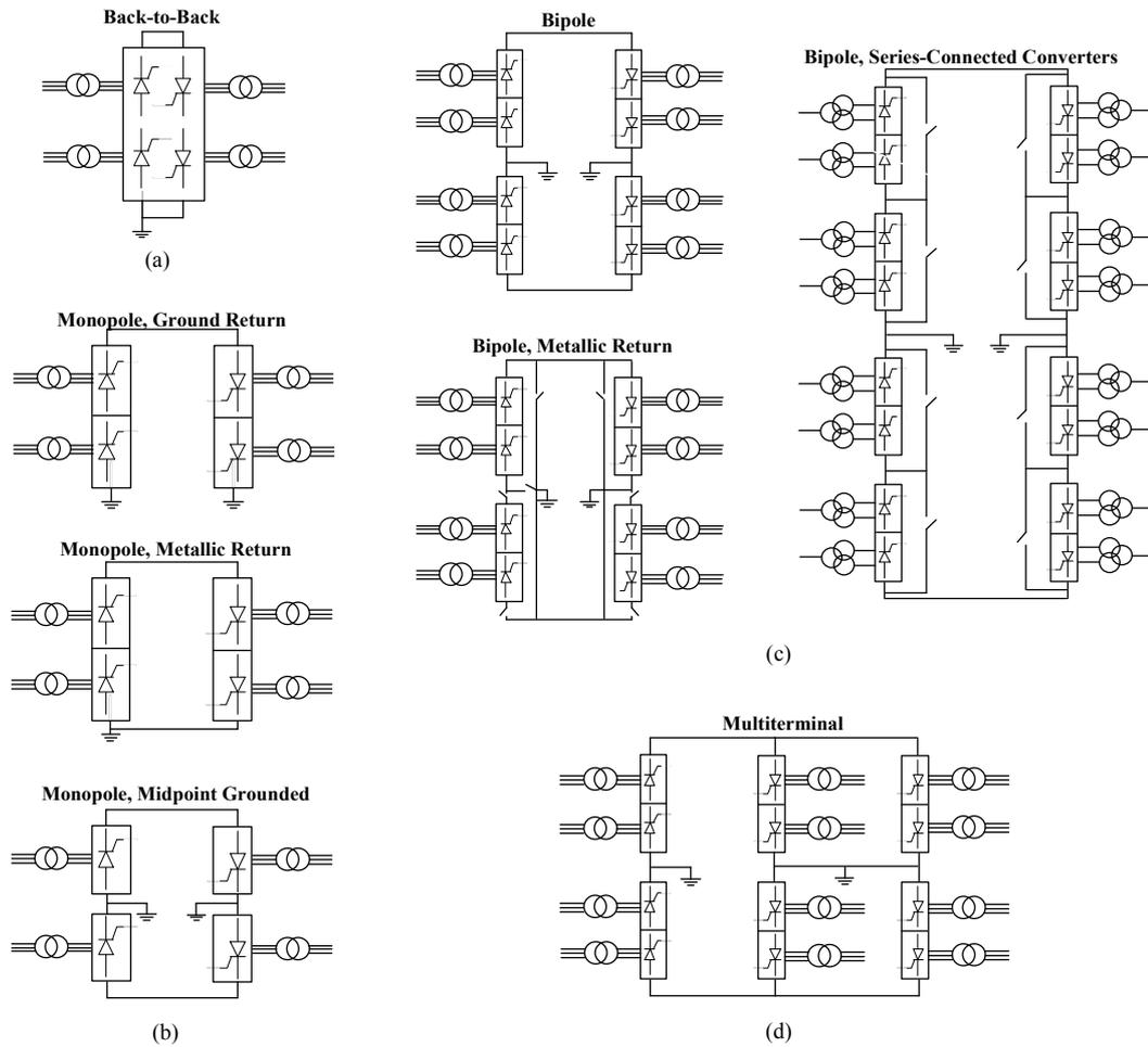
Fig. 1.4: CSC-HVDC system configurations and operating modes: (a) back-to-back, (b) monopolar, (c) bipolar, and (d) multi-terminal.
