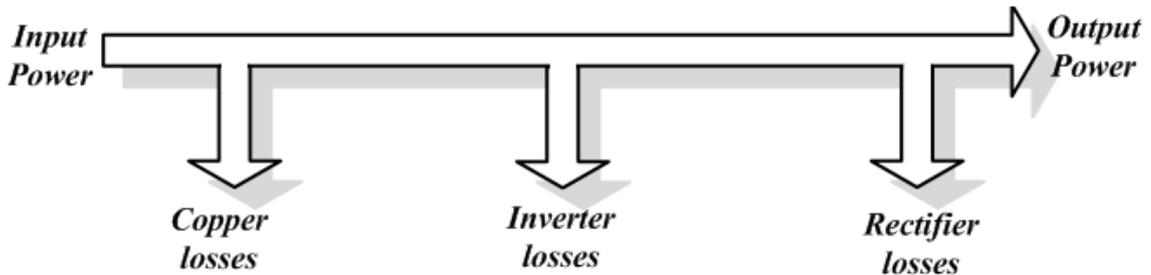
Fig. 3.8: Power flow diagram for a SPRC
