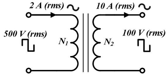
Fig. 3.13: Nano-crystalline core transformer full-load ratings
