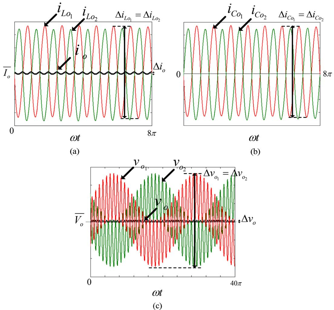
Fig. 3.19: Results for two interleaved SPRC output filters in ISOS connection (a) module inductor currents and output (load) current, (b) capacitor currents, (c) module output voltages and total load voltage.
