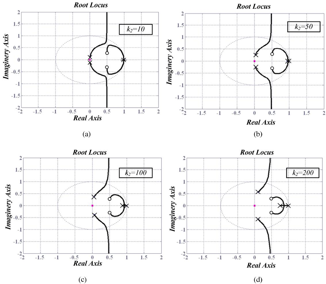
Fig. 5.22: Root loci for system with predictive controller (a)  $k_2=10$ , (b)  $k_2=50$ , (c)  $k_2=100$ , and (d)  $k_2=200$ .
