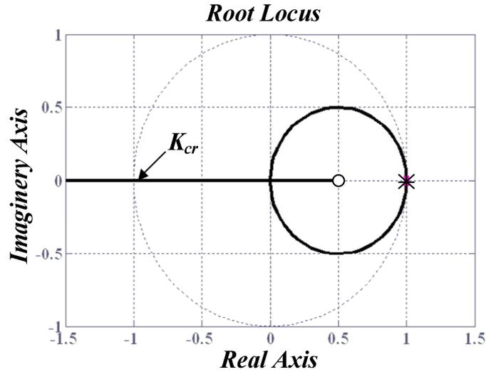
Fig. 5.6: Root locus for discretized system with Lyapunov controller.
