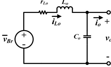
Fig. 4.4: Equivalent circuit diagram for the dc sub-system.
