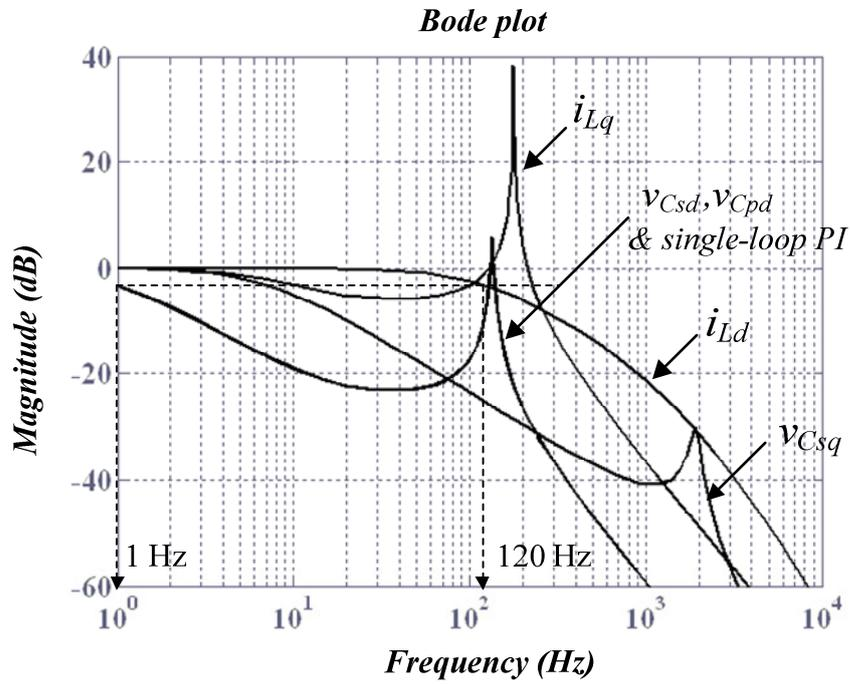
Fig. 4.29: Bode plot illustrating closed-loop bandwidth with the different state variables used for the inner control loop
