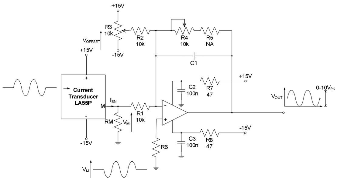
Fig. A.5: Current transducer circuit diagram
