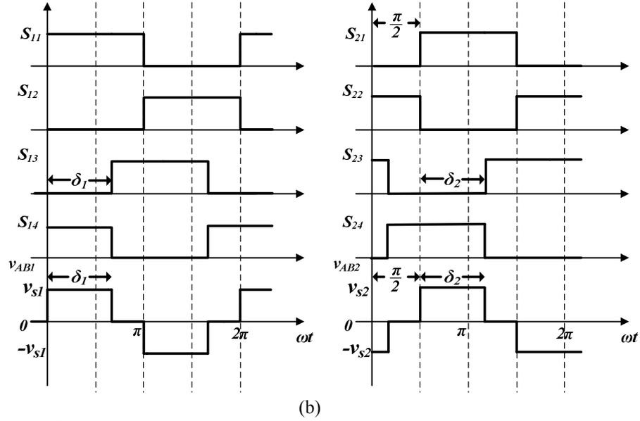
Fig. 6.6: Two-module ISOP connected phase-controlled SPRC (a) circuit diagram and (b) interleaved modules inverter gating patterns.
