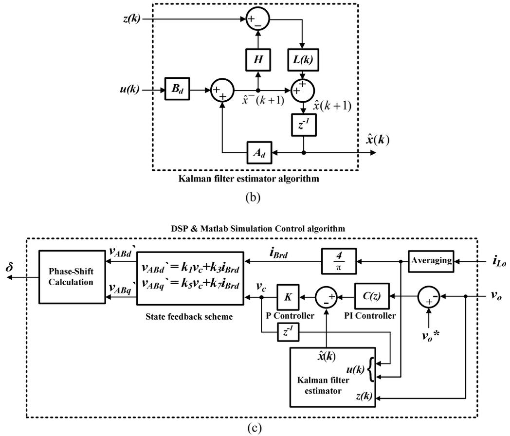
Fig. 4.25: Closed-loop sensorless multi-loop control scheme (a) Circuit diagram, (b) Kalman filter estimator, and (c) Control algorithm.
