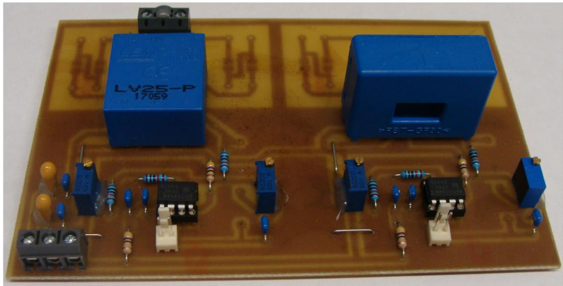
Fig. A.7: Voltage (left) and current (right) transducer circuit boards.
