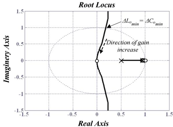
Fig. 5.25: Root locus for system with circuit parameter change.
