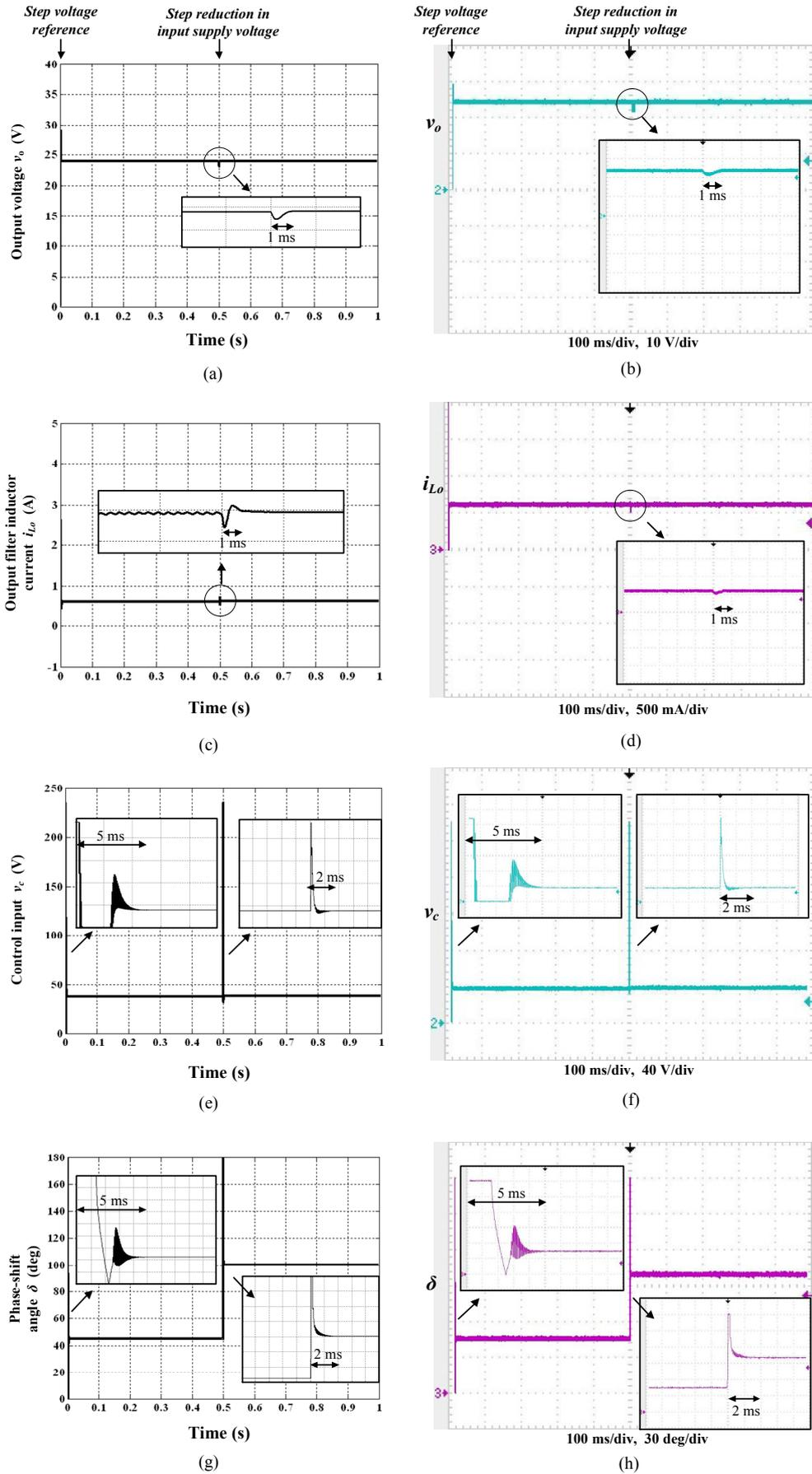
Fig. 5.8: Closed-loop operation results with step input voltage disturbance using the proposed Lyapunov controller (a), (c), (e) and (g) simulation, and (b), (d), (f) and (h) experimental.
