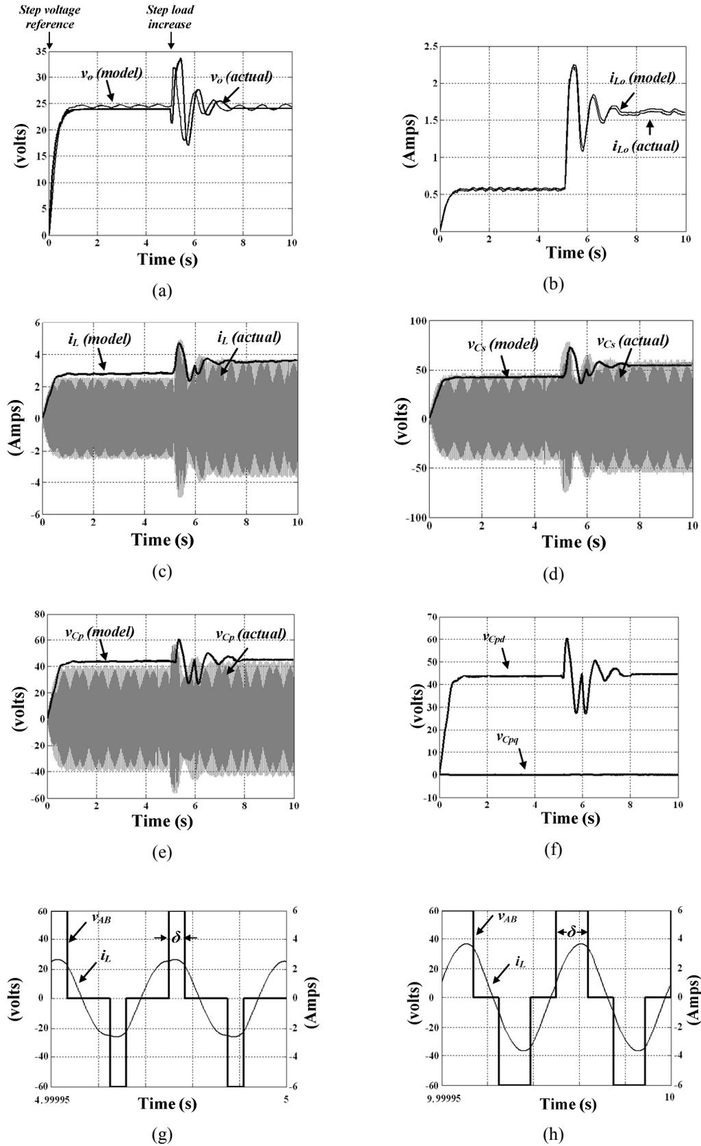
Fig. 4.20: Matlab simulations comparing actual switching and proposed large-signal model (full-load applied at  $t=5.0s$ ), (a) output voltage, (b) output filter inductor current, (c) resonant inductor current, (d) series resonant capacitor voltage, (e) parallel resonant capacitor voltage, (f)  $dq$  equivalent resonant tank parallel capacitor voltages, (g) inverter output voltage at part-load, and (h) inverter output voltage at full-load.
