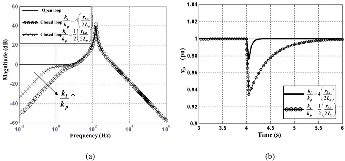
Fig. 4.16: (a) Bode plots for open- and closed-loop converter output impedance, and (b) effect of changing  $k_i/k_p$  on closed-loop response to a step load change.
