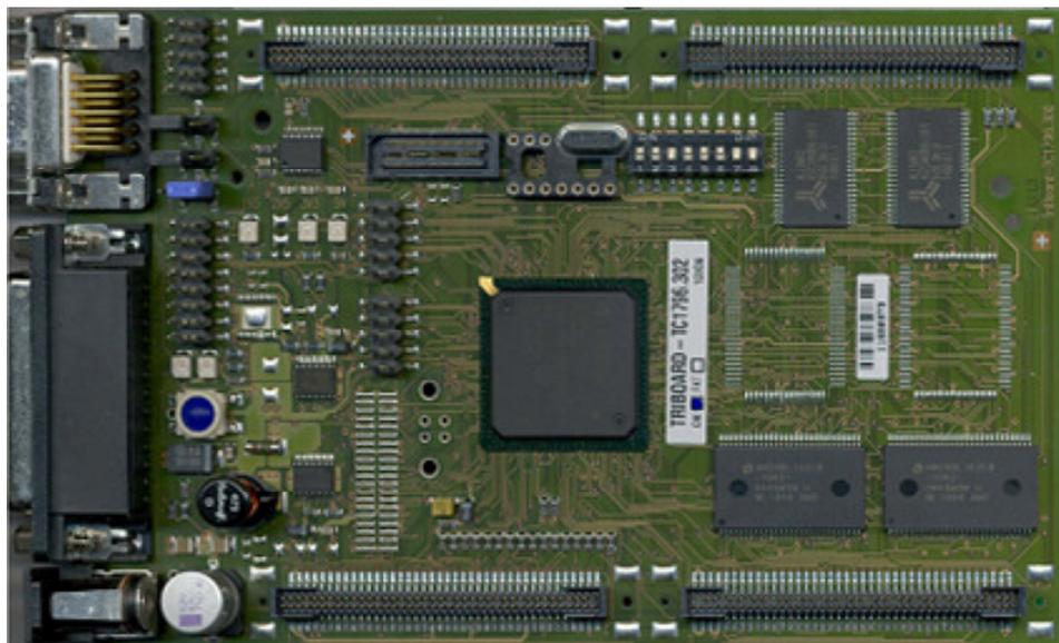
Fig. A.2: Infineon Tricore TC1796 DSP
