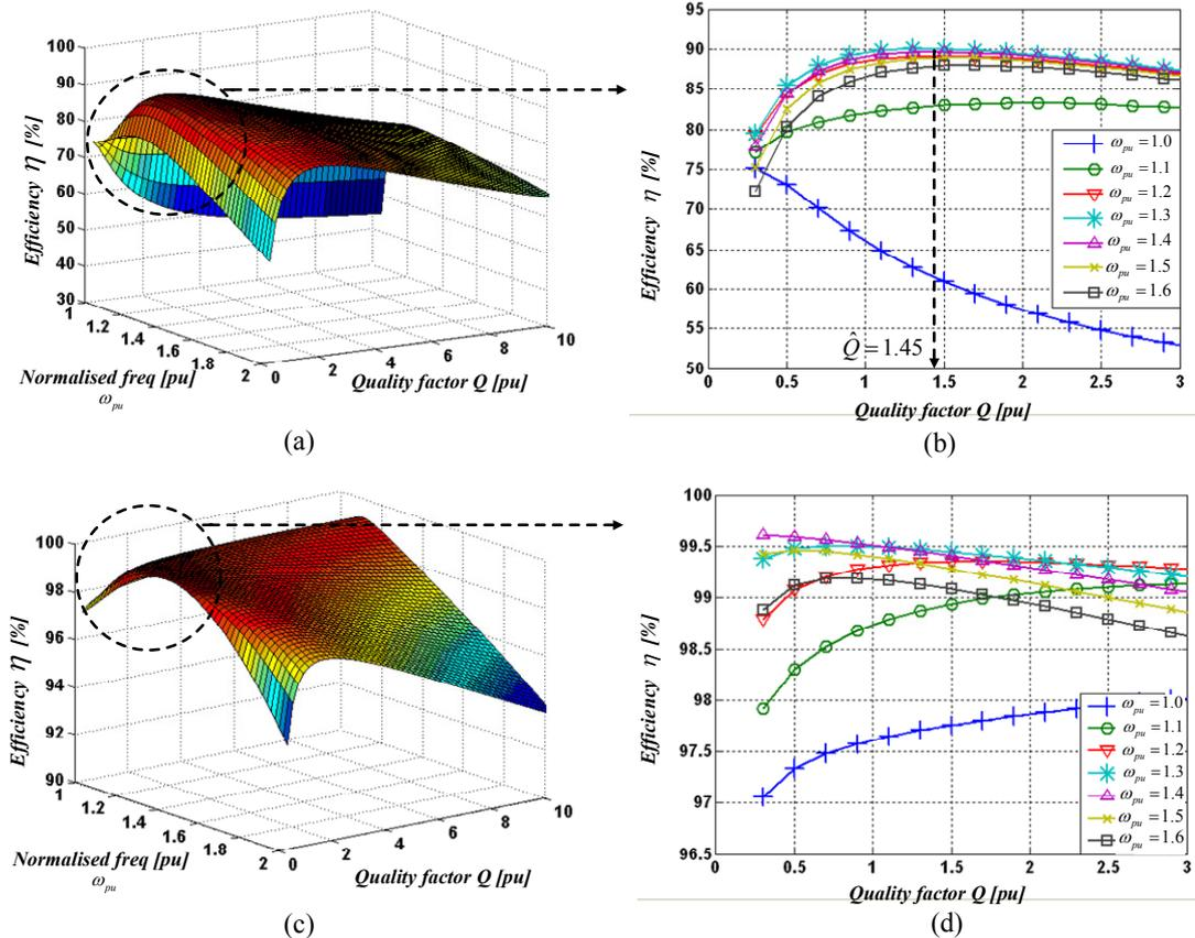
Fig. 3.11: Phase-controlled SPRC efficiency plots (a) 3D view (b) focus on global maximum at selected frequencies (c) 3D view of efficiency considering inverter & rectifier losses only (d) global maximum.
