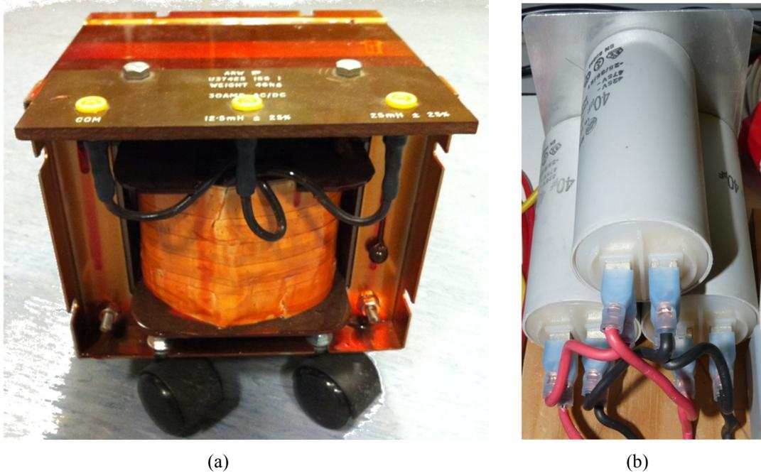
Fig. A.14: Output LC filter (a) inductance, and (b) capacitance
