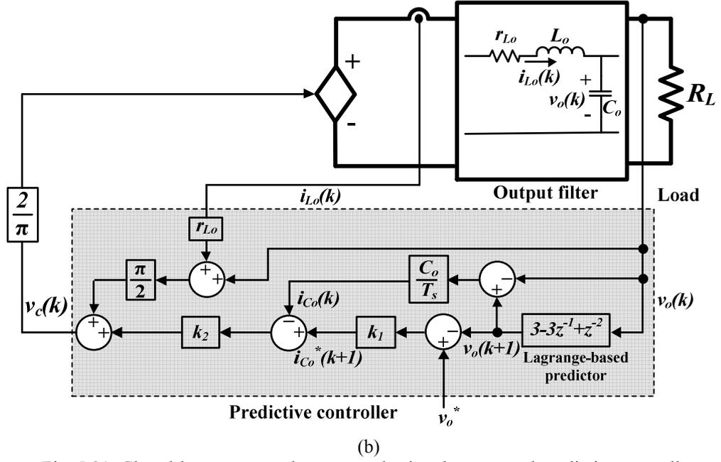
Fig. 5.21: Closed-loop output voltage control using the proposed predictive controller (a) full structure and (b) reduced equivalent model.
