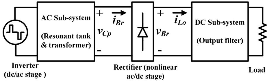
Fig. 4.2: Conversion stages and sub-systems in a typical resonant converter.
