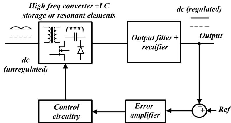
Fig. 2.2: Functional block diagram of dc/dc converters.
