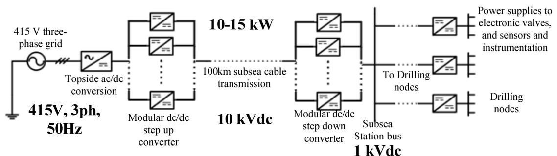
Fig. 1.8: Single line diagram of the subsea power distribution project with modular dc/dc converters.
