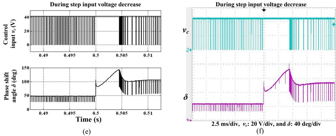
Fig. 5.19: Closed-loop operation results with step input voltage disturbance using the proposed sliding mode controller (a),(c) and (e) simulation, and (b),(d) and (f) experimental.
