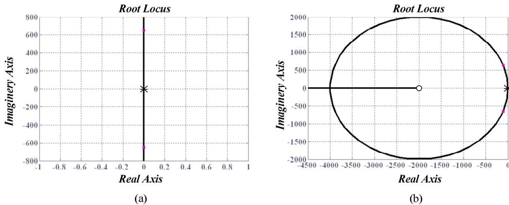
Fig. 5.4: Root loci for system with feedforward loop of Lyapunov controller
