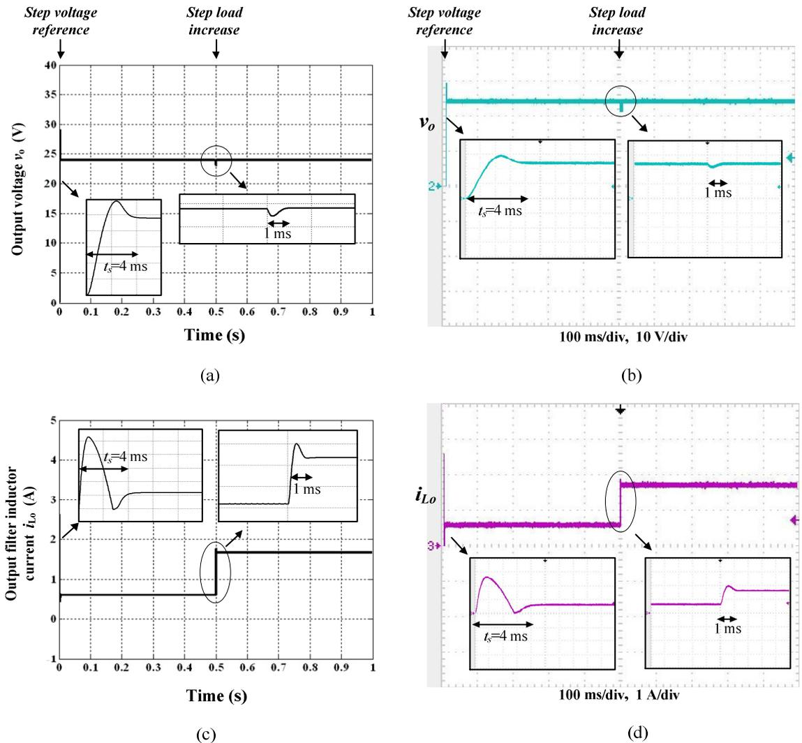
Fig. 5.7: Closed-loop operation results with step load disturbance using the proposed Lyapunov controller (a) and (c) simulation, and (b) and (d) experimental.
