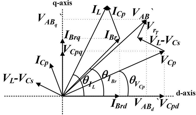
Fig. 4.6: Steady-state phasor diagram of the ac sub-system.
