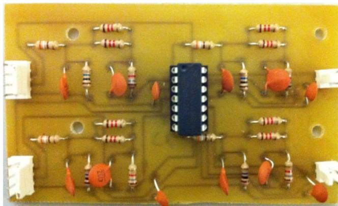
Fig. A.17: Low pass filter circuit for DSP analogue output
