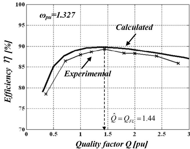
Fig. 3.24: Comparison between converter calculated and experimental efficiency results.
