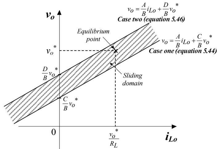
Fig. 5.15: Graphical representation of sliding domain.
