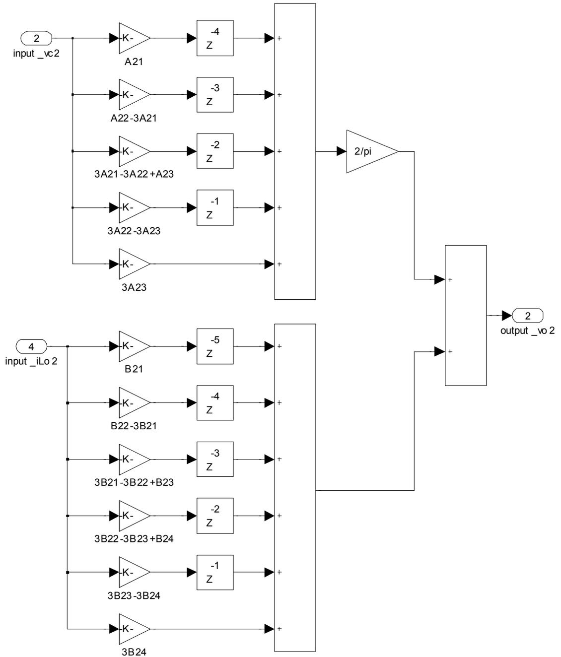
Fig. C.2: Simulink block diagram of load voltage estimation algorithm
