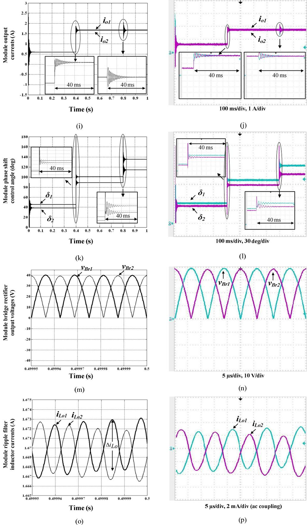
Fig. 6.7: Results for the ISOP connected phase-controlled SPRC (a),(c),(e), (g), (i), (k), (m) and (o) simulation, and (b),(d),(f), (h), (j), (l), (n) and (p) experimental.
