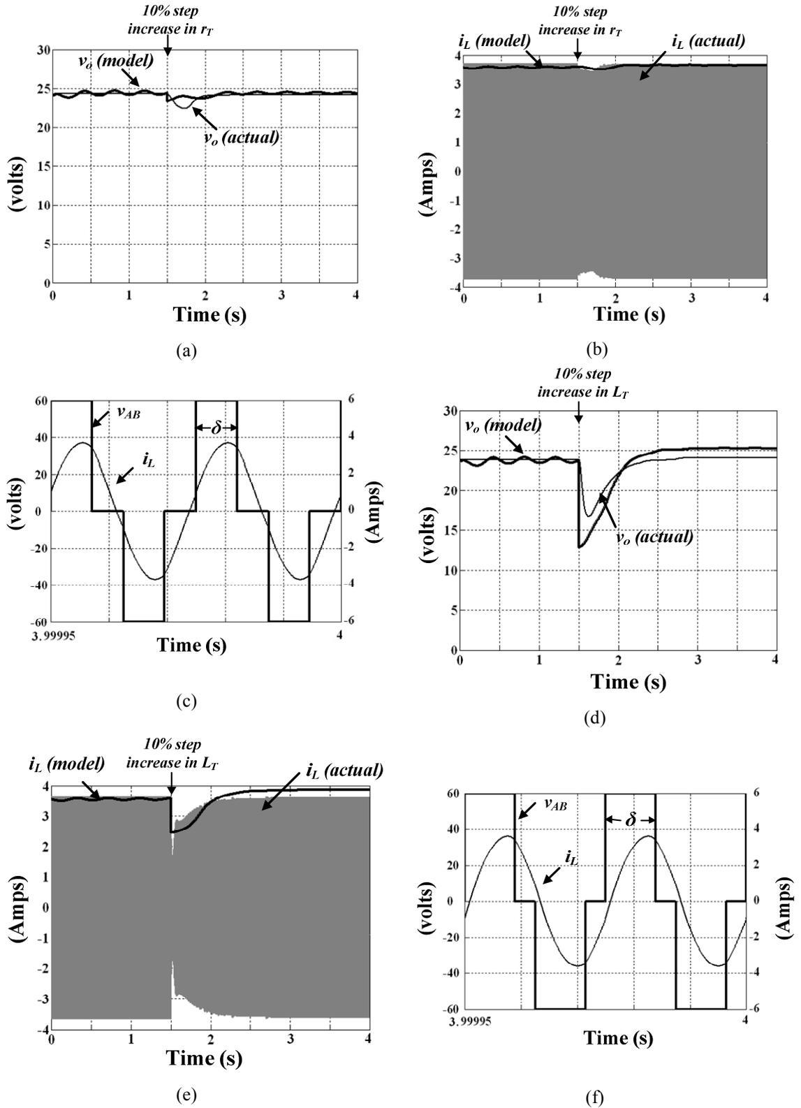
Fig. 4.22: Results for robustness analysis comparing the actual converter operating at  $Q_{FL}$  with the proposed model, in response to a +10% step change (at  $t=1.5$ s) in the value of: (a)-(c)  $r_T$  and (d)-(f)  $L_T$ .
