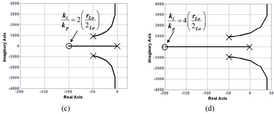
Fig. 4.12: Root loci for the open-loop transfer function  $C(s)G_I(s)$
