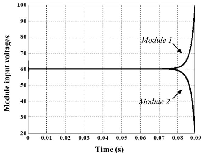
Fig. 6.3: Diverging module input voltages in an ISOP connected system with OCS and no IVS control.
