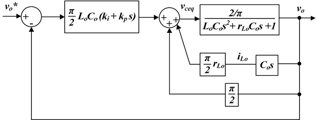
Fig. 5.16: Equivalent control closed-loop structure for the proposed SMC.
