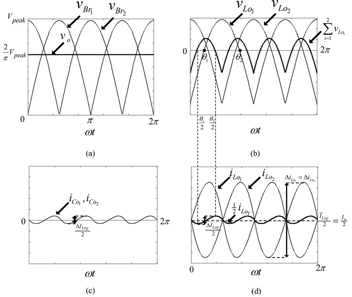
Fig. 3.18: Results for two interleaved SPRC output filters in ISOP connection (a) bridge rectifier output voltages and converter output voltage, (b) inductor voltages, (c) capacitor currents, (d) inductor currents
