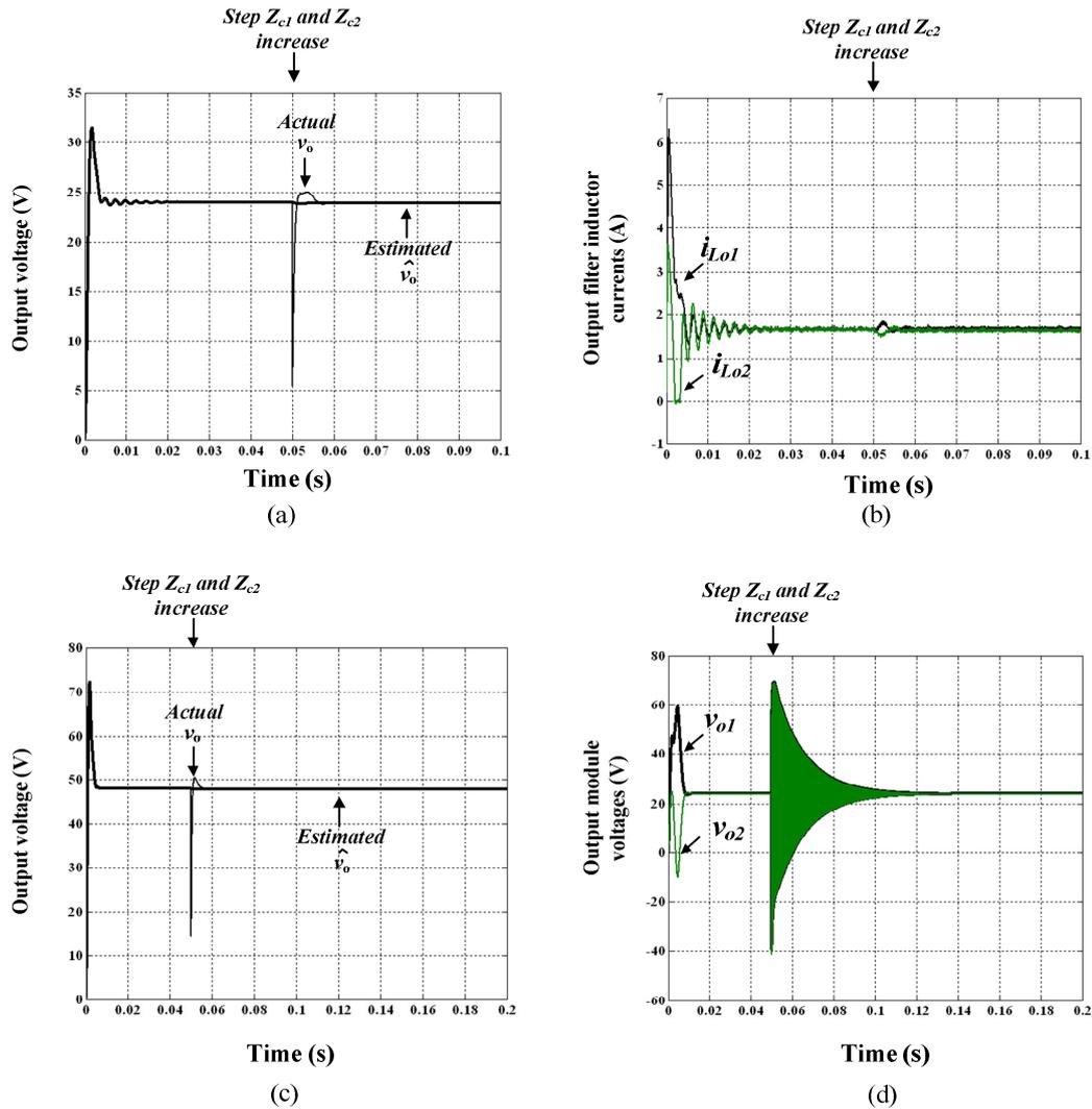
Fig. 6.10: Load voltage estimator sensitivity to varying cable impedance (a) and (b) ISOP system, and (c) and (d) ISOS system.
