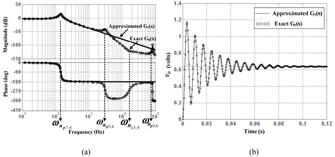
Fig. 4.10: Comparison between approximate and exact control-to-output voltage transfer function (a) Bode plot, and (b) step response.
