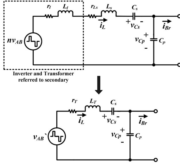
Fig. 4.3: Equivalent circuit diagrams for the ac sub-system.
