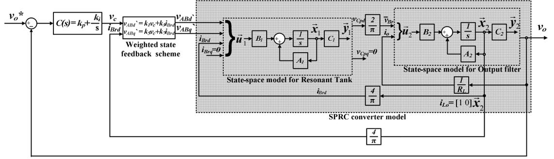
Fig. 4.17: Closed-loop SPRC output voltage control using the proposed linearization scheme.
