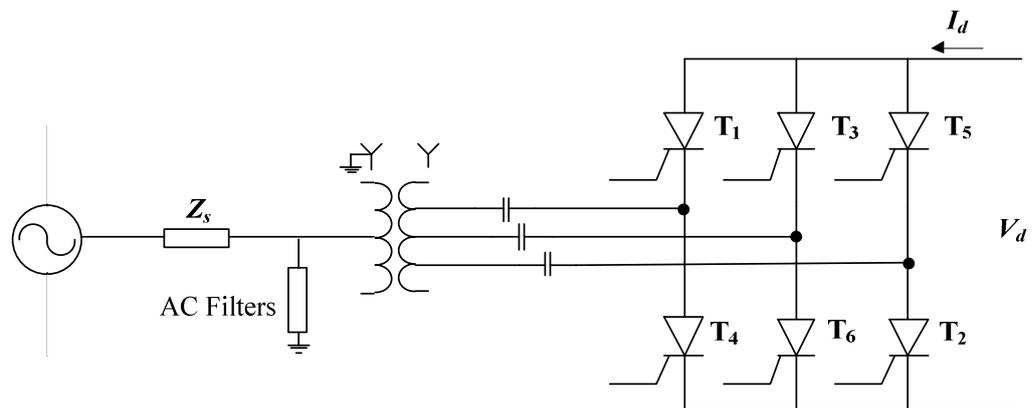
Fig. 1.5: Typical CCC configuration.
