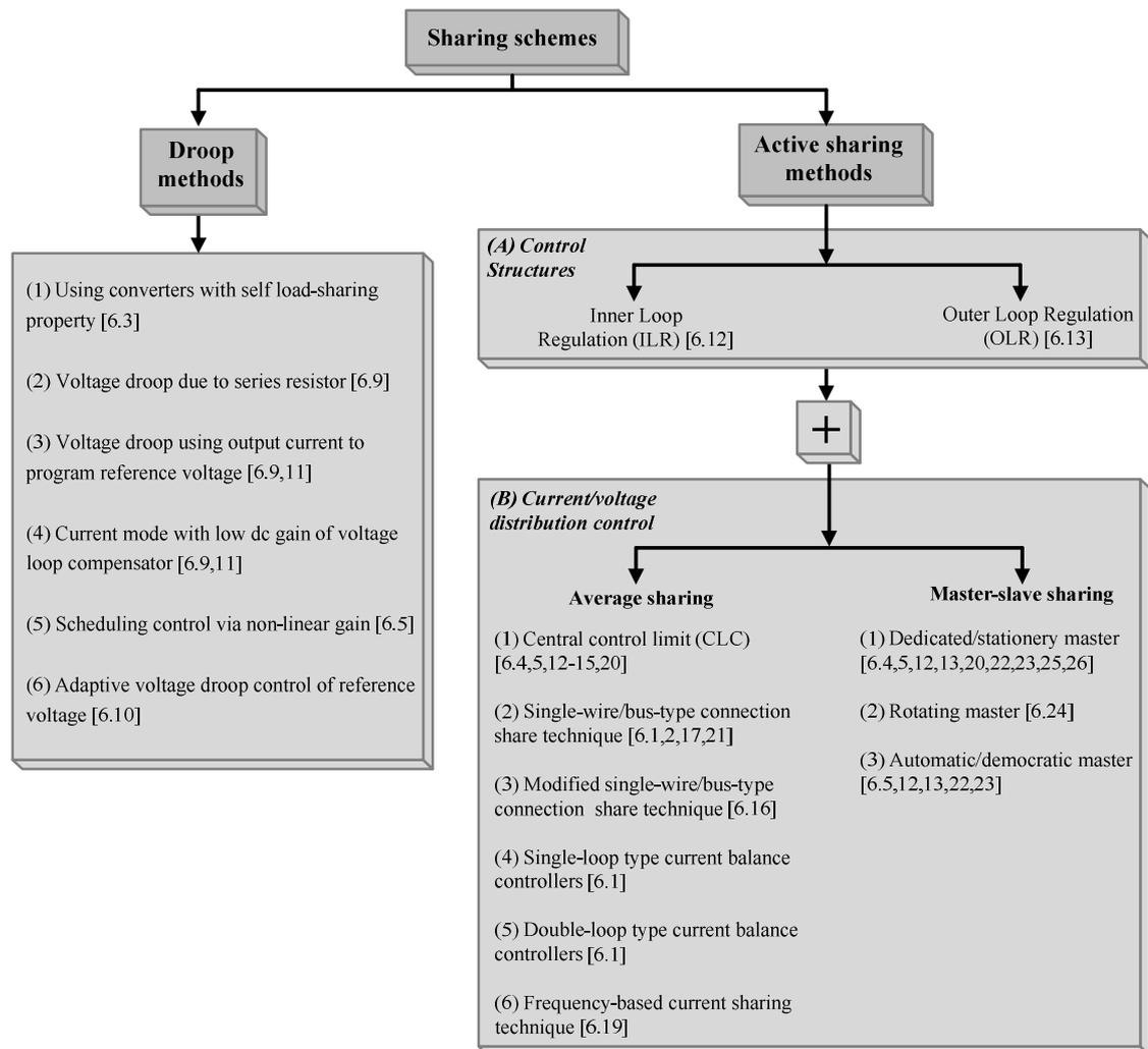
Fig. 6.1: Classification of sharing schemes for series-parallel dc/dc converters
