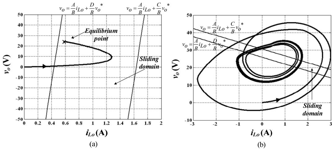
Fig. 5.17: Typical closed-loop behaviour at start-up (a) stable response, and (b) unstable oscillatory response.
