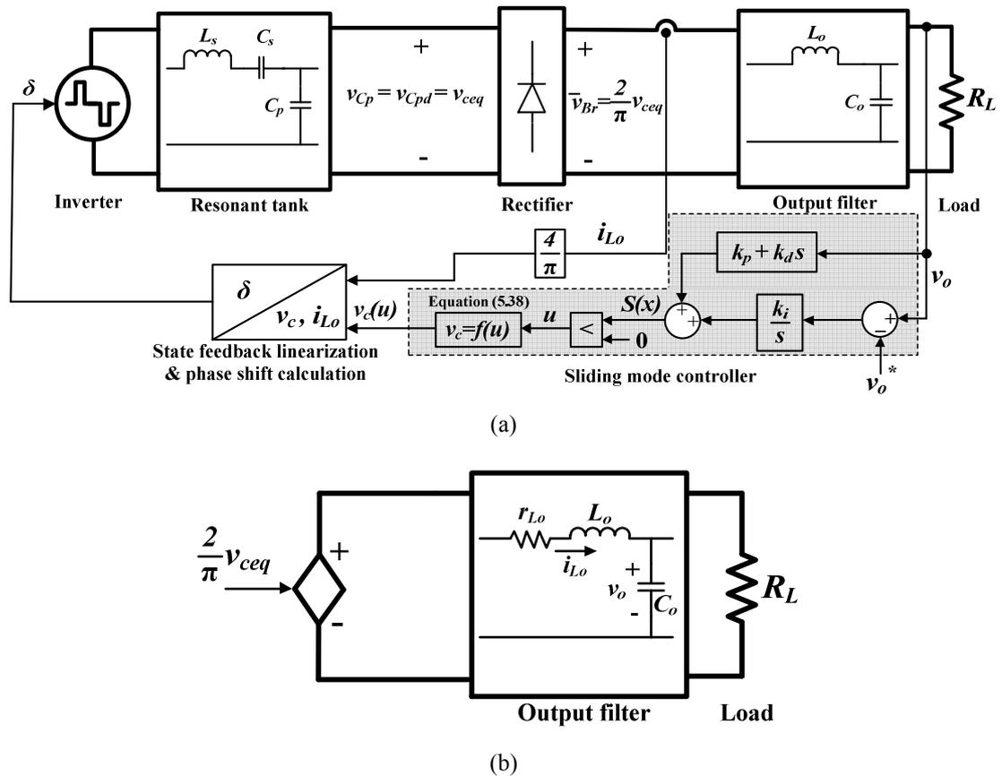
Fig. 5.14: Closed-loop output voltage control using the proposed sliding mode controller (a) full structure, and (b) reduced equivalent model using the equivalent control input  $v_{ceq}$ .
