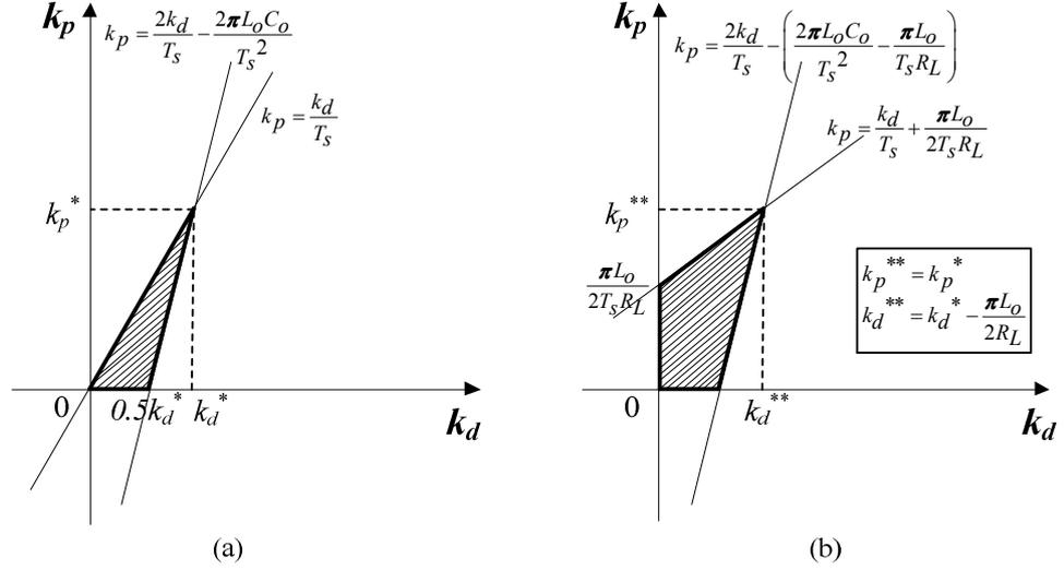
Fig. 5.5:  $k_p$ - $k_d$  map for closed-loop output voltage control stability margins (a) at no load and (b) with load.
