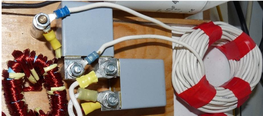
Fig. A.13: LCC resonant tank
