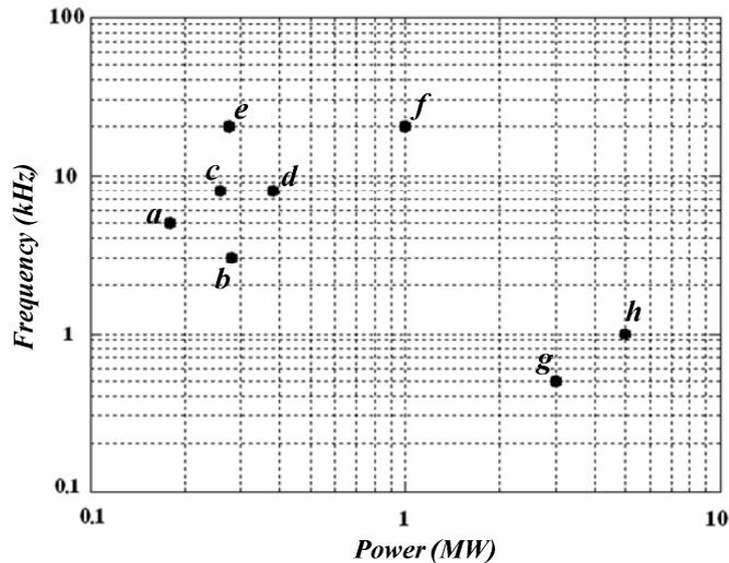
Fig. 2.6: Frequency vs. power map with different high-power dc/dc converter research efforts: (a) Alstom (15kV to 3.6kV) [2.54], (b) Uniflex (3.3kV to 3.3kV) [2.55], (c) ABB (15kV to 2.8kV) [2.56], (d) Bombardier (15kV to 3.6kV) [2.57], (e) Freedom NCSU (24kV to 0.75kV) [2.58], (f) ETH Zurich (12kV to 1.2kV) [2.59], (g) KTH (33kV to 3kV) [2.60], and (h) E. ON RWTH (5kV to 5kV).
