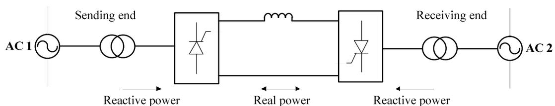
Fig. 1.3: HVDC system based on CSC technology with thyristors.
