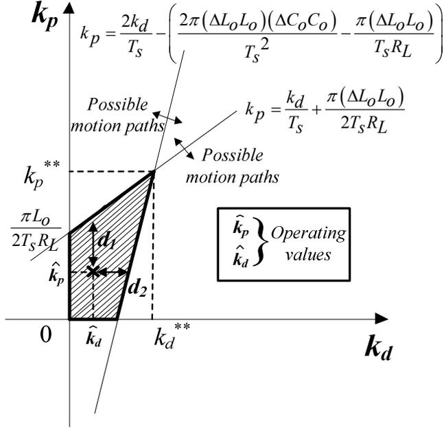
Fig. 5.11: Closed-loop stability margins for system parameter variation.
