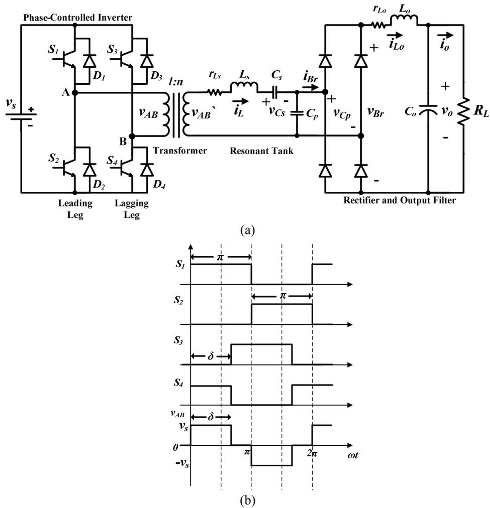
Fig. 3.1: Series-parallel resonant converter
