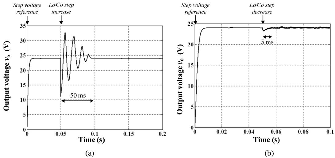
Fig. 5.20: Output voltage step response applying step changes in  $L_o$  and  $C_o$
