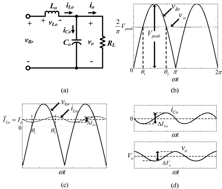
Fig. 3.16: SPRC output filter (a) circuit diagram, (b) bridge rectifier output voltage and converter output voltage, (c) inductor voltage and current and (d) capacitor voltage and current
