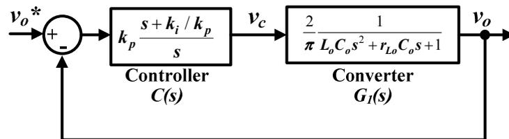
Fig. 4.11: Closed-loop structure for output voltage control.
