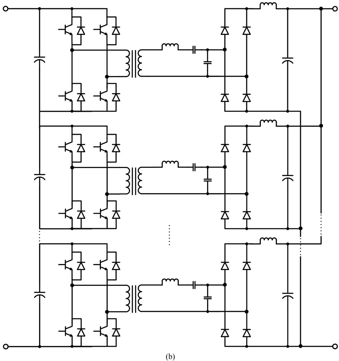
Fig. 2.7: Phase-controlled SPRC selected for the *All-Electric* subsea project (a) IPOS connection for voltage step up substation, and (b) ISOP connection for voltage step down substation.
