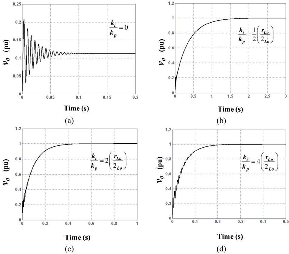
Fig. 4.13: Closed-loop step response for output voltage control loop
