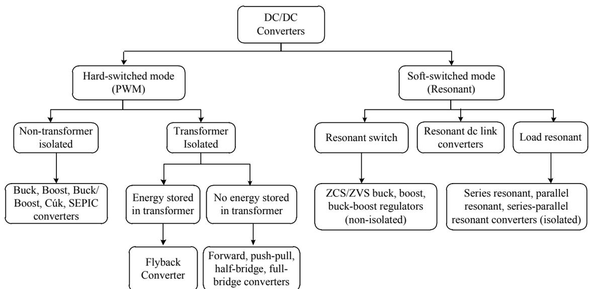
Fig. 2.1: General tree classification of dc/dc converters.
