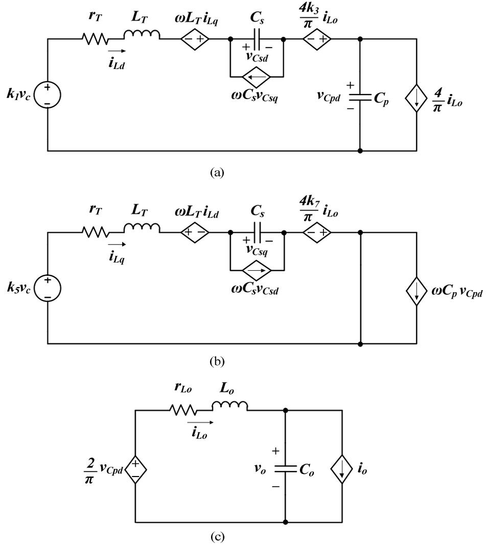
Fig. 4.27: Linearized model equivalent circuits (a)  $d$ -axis, (b)  $q$ -axis, and (c) output filter.
