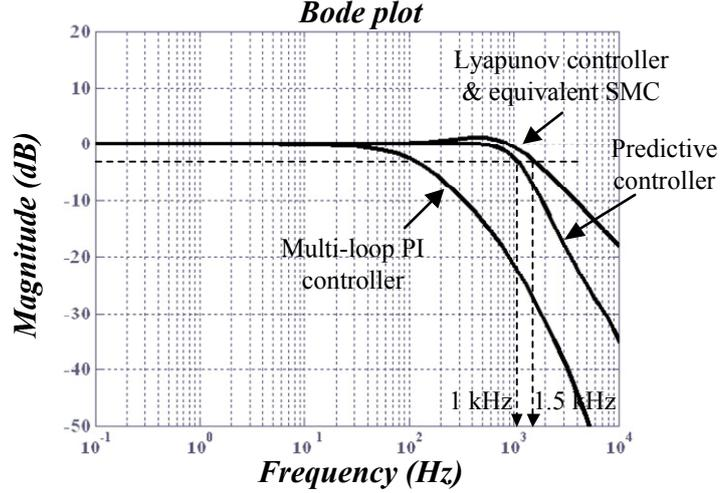
Fig. 5.24: Comparison of closed-loop bandwidth.
