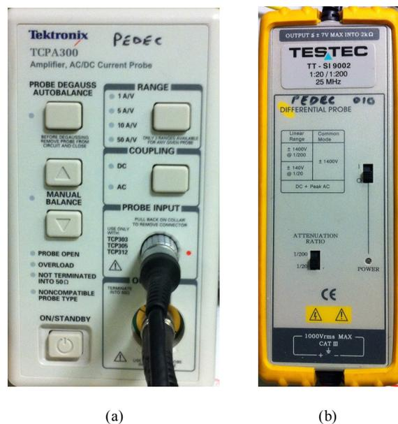
Fig. A.20: Test probes (a) current, and (b) voltage.
