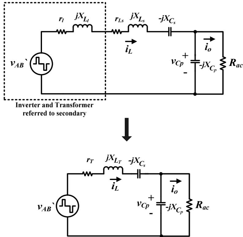
Fig. 3.2: AC equivalent circuit of the series-parallel resonant converter ( $r_T=r_l+r_{Ls}$  and  $X_{LT}=X_{Ll}+X_{Ls}$ )
