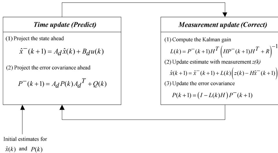
Fig. 4.24: Kalman filter recursive algorithm
