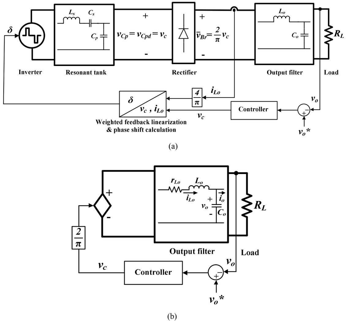
Fig. 5.1: Closed-loop output voltage control configuration using the linearization scheme
