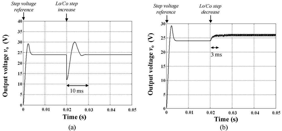
Fig. 5.12: Output voltage step response applying step changes in  $L_o$  and  $C_o$
