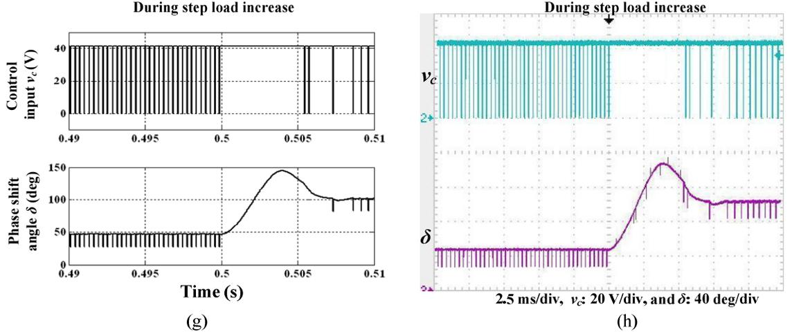
Fig. 5.18: Closed-loop operation results with step load disturbance using the proposed sliding mode controller (a),(c),(e) and (g) simulation, and (b),(d),(f) and (h) experimental.
