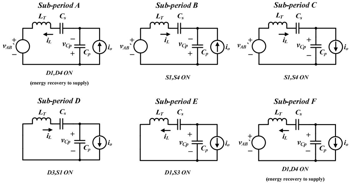
Fig. 3.5: Equivalent ac circuits for the positive half-cycle sub-periods
