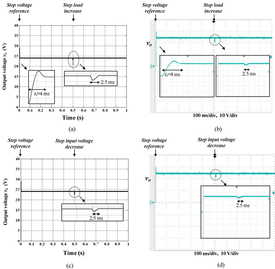
Fig. 5.23: Closed-loop output voltage results with step load and step input voltage disturbances using the proposed predictive controller (a) and (c) simulation, and (b) and (d) experimental.
