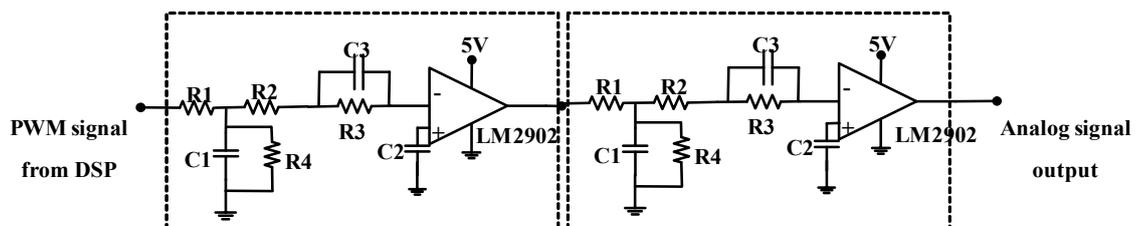
Fig. A.18: Circuit diagram for Low pass filter circuit for DSP analogue output
