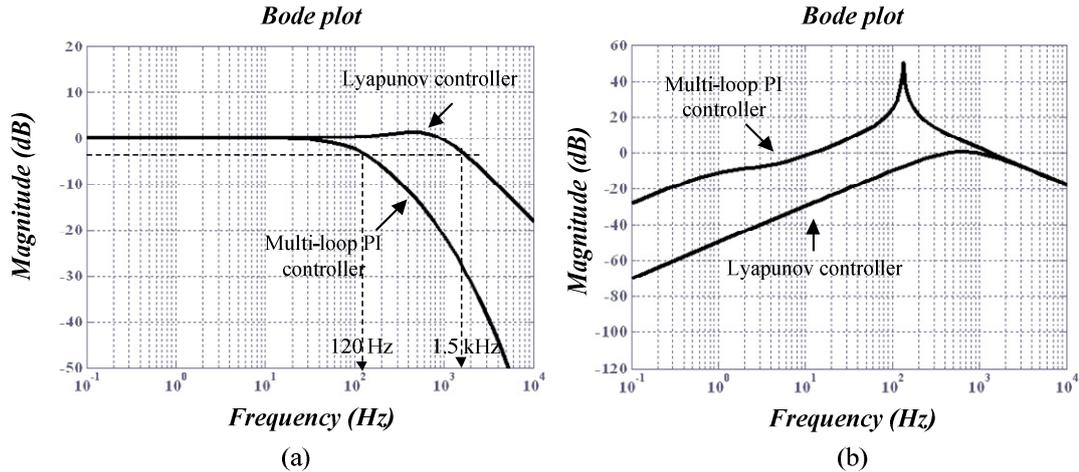
Fig. 5.10: Bode plots comparing the proposed Lyapunov controller and the multi-loop PI controller (a) closed-loop bandwidth and (b) closed-loop output impedance.
