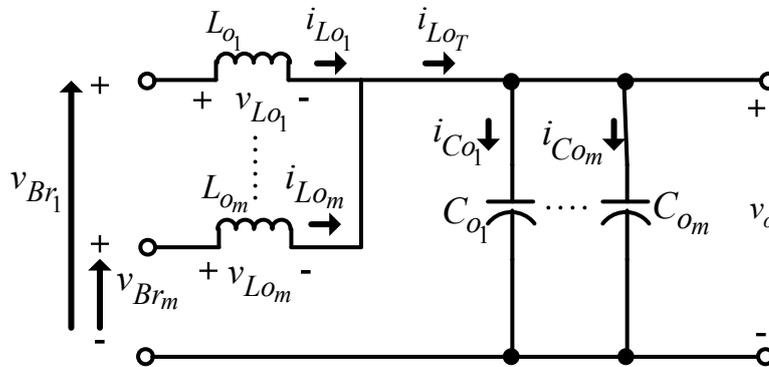
Fig. 3.17: Config#1 for ISOP connection
