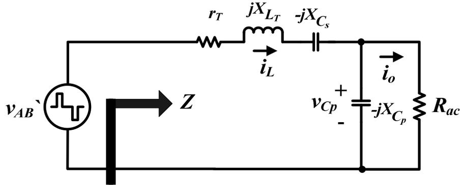
Fig. 3.4: Input impedance  $Z$  of resonant circuit
