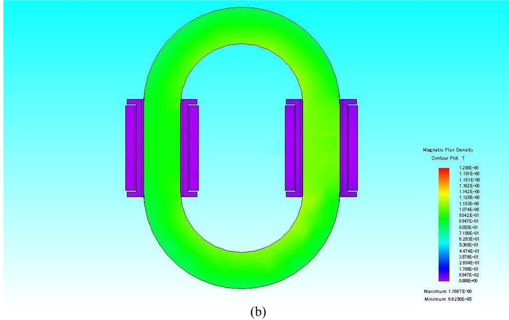
Fig. 3.15: (a) Converter circuit diagram using JMAG-Designer circuit simulator and (b) Maximum operating core flux density
