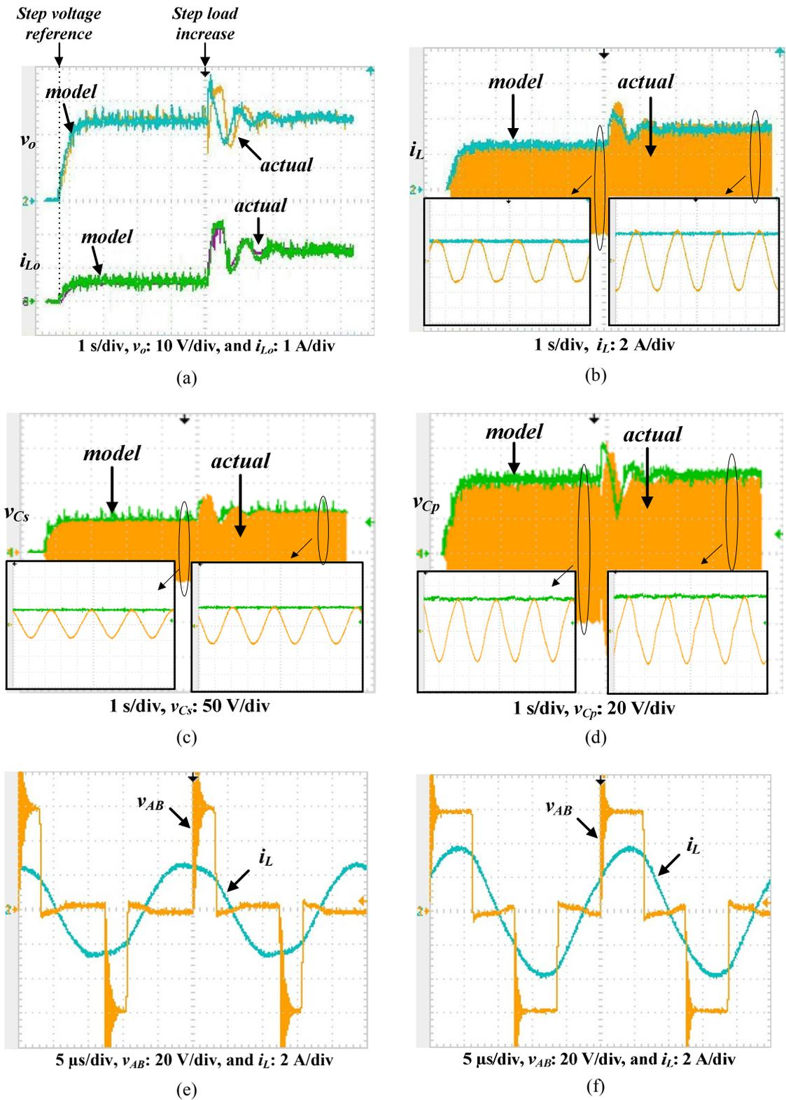
Fig. 4.21: Experimental results comparing measurements from the actual converter and the proposed large-signal model, (a) output voltage and output filter inductor current, (b) resonant tank inductor current, (c) resonant tank series capacitor voltage, (d) resonant tank parallel capacitor voltage, (e) inverter output voltage at part-load (f) inverter output voltage at full-load.
