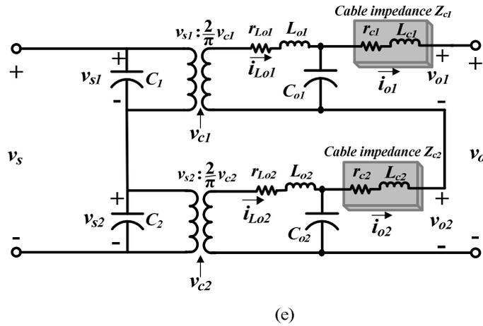
Fig. 6.4: Proposed two-module phase-controlled SPRC (a) ISOP connection, (b) ISOS connection, (c) common control structure for both connections, (d) reduced equivalent control circuit for ISOP connection, and (e) reduced equivalent control circuit for ISOS connection.
