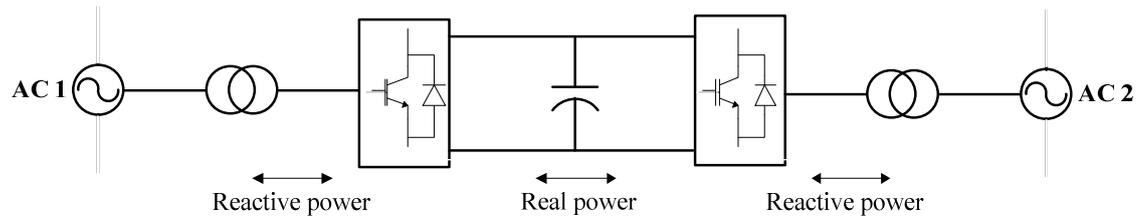
Fig. 1.6: HVDC system based on VSC technology using IGBTs.
