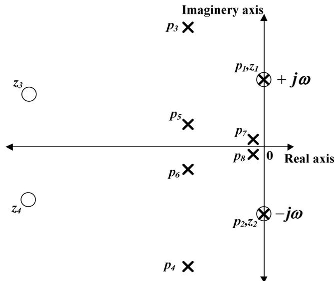
Fig. 4.9: Pole-zero map for actual control-to-output voltage transfer function  $G_I(s)$  in complex  $s$ -plane.
