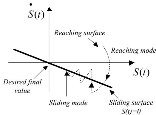
Fig. 5.13: Concept of sliding mode control.
