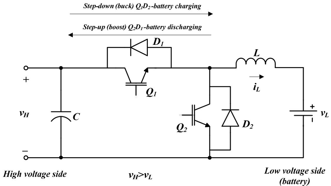
Fig. 2.4: A buck converter with two-quadrant bi-directional power flow.
