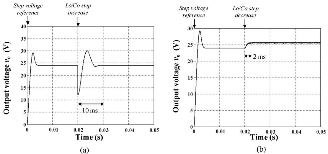
Fig. 5.26: Output voltage step response applying step changes in  $L_o$  and  $C_o$
