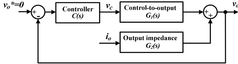
Fig. 4.15: Control structure to obtain the closed-loop output impedance
