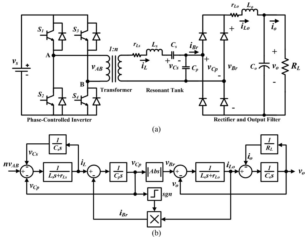
Fig. 4.1: (a) Circuit diagram for the SPRC and (b) non-linear model representation of the SPRC.
