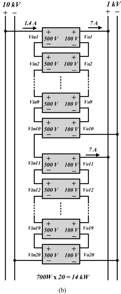
Fig. 3.12: (a) Proposed SPRC, full-load operating values (b) 20 modules connected in ISOS/OP to achieve the 14 kW, 10kVdc/1 kVdc step down load side converter
