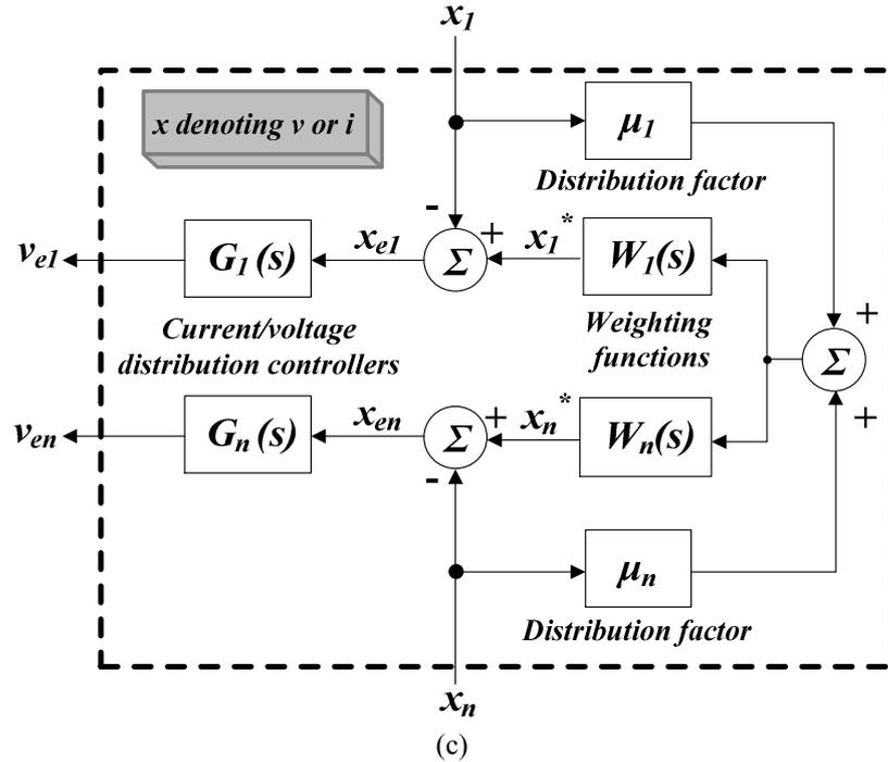
Fig. 6.2: (a) Inner loop regulation (ILR) control structure, (b) outer loop regulation (OLR) control structure and (c) current/voltage distribution control
