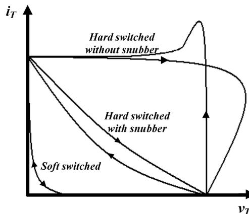
Fig. 2.3: Comparison of switching conditions in hard and soft switched transistors.
