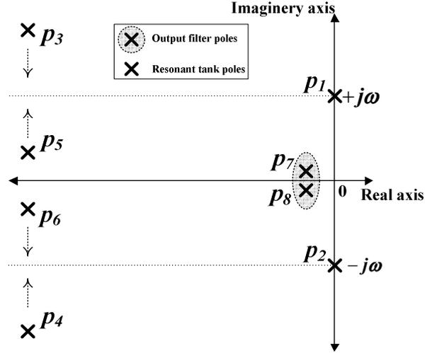
Fig. 4.8: Complex  $s$ -plane showing poles of the linearized resonant converter model.
