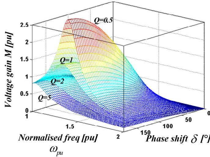
Fig. 3.3: Converter voltage gain  $M$
