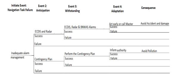
Figure 7-5 Poor alarm management ETA
