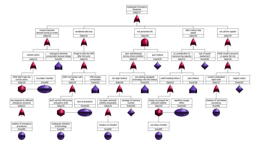
Figure 11-4 Inadequate Emergency Response FTA
