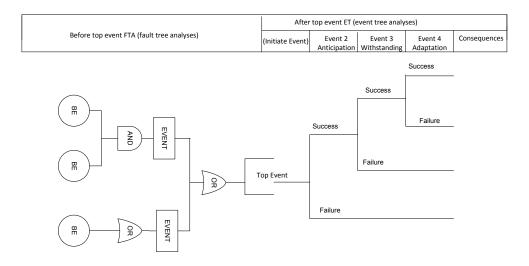
Figure 4-7 Bow-tie Illustration include FTA and ETA
