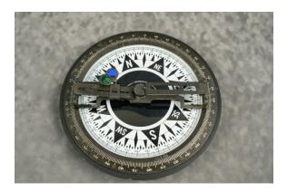
Figure 11-25 Navigation compass (from http://www.lighthouselens.com)
