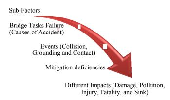
Figure 4-5 Failure escalation of bridge operation
