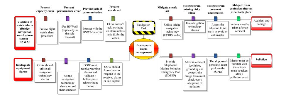
Figure 11-15 Inadequate alarm management Bow-tie
