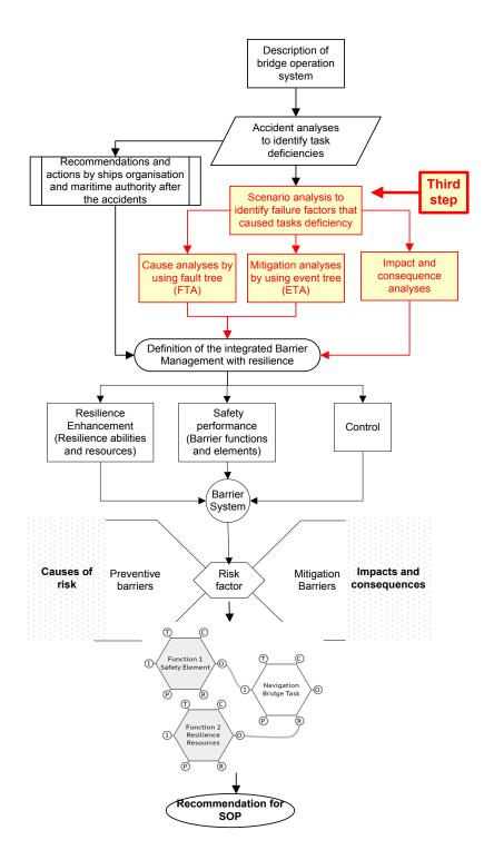
Figure 4-6 indicate the third step of the resilient safety system framework
