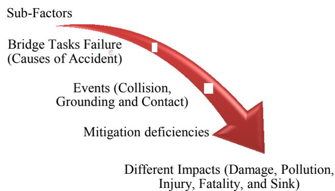
**Figure 4-5 Failure escalation of bridge operation**
