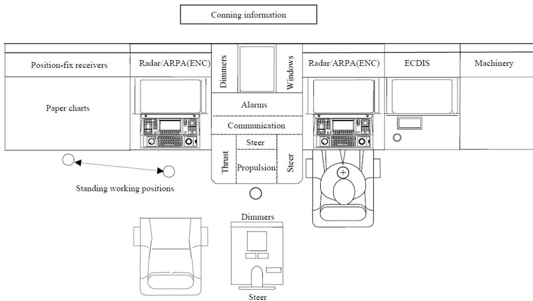
**Figure 5-7 Example of principles for location of main equipment in a centre console (IACS, 1992)**
