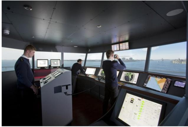
Figure 8-2 Photo of TRANSAS 360° full mission Navigation bridge simulator
