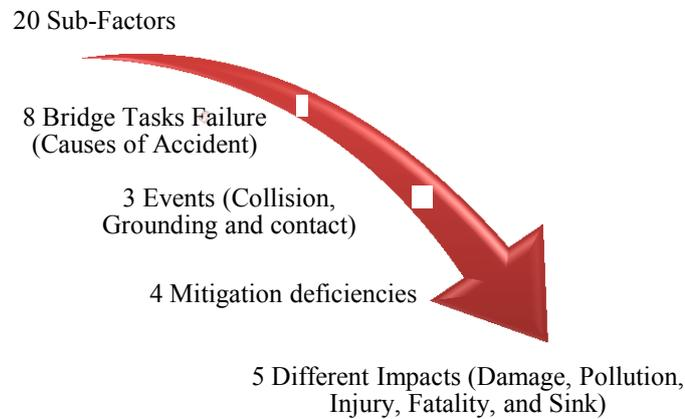
**Figure 6-1 Failure escalation of bridge operation**
