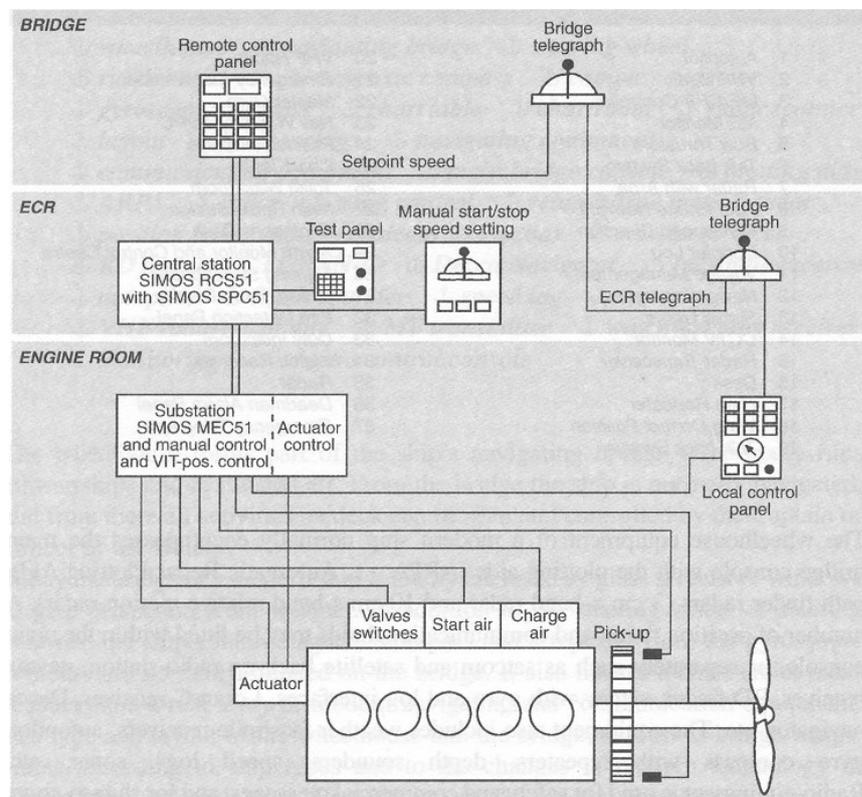
**Figure 5-6 Engine control system from the bridge (University.of.Rijeka, 2013).**
