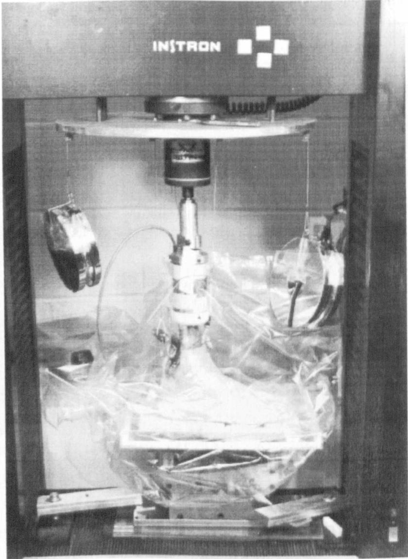
Figure 4.2 A foot specimen mounted in the Instron® test machine. Muscle forces were simulated using static weights applied to tendons with wire traces.
