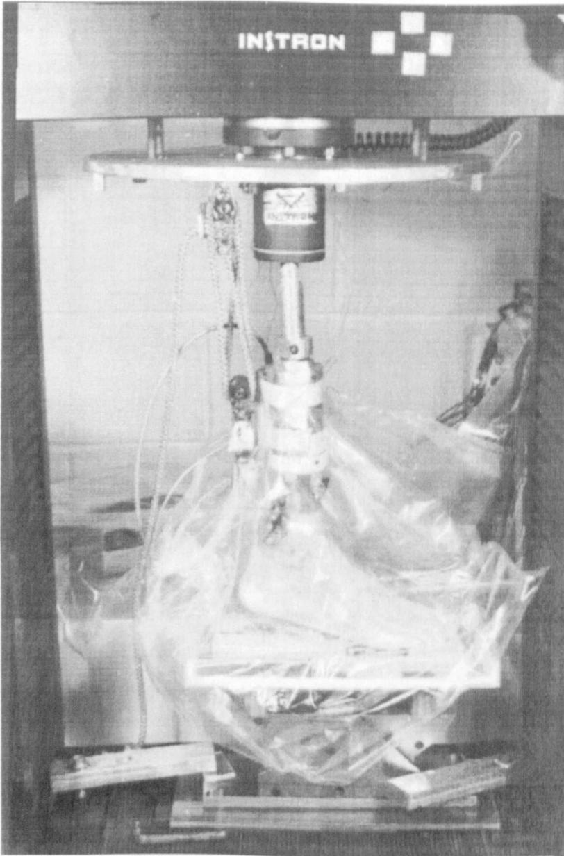
Figure 4.3 Foot mounted in the Instron® during the gait experiments. The foot is shown in the toe-off position with the pulley system attached to the Achilles tendon
