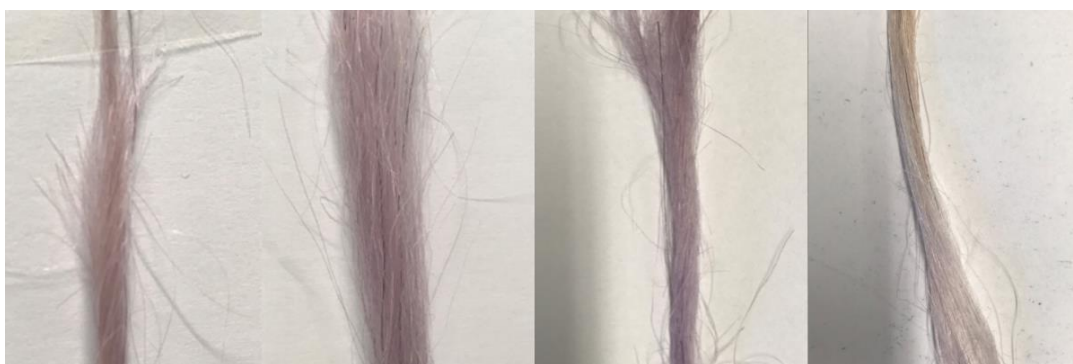
Figure 5.13: Hairs dyed with ALZ, ALZ-PYR, ALZ-ACR and ALZ-PHN respectively after 30 minutes of dyeing, followed by 30 minutes of washing in hot soapy water at 50 °C.
