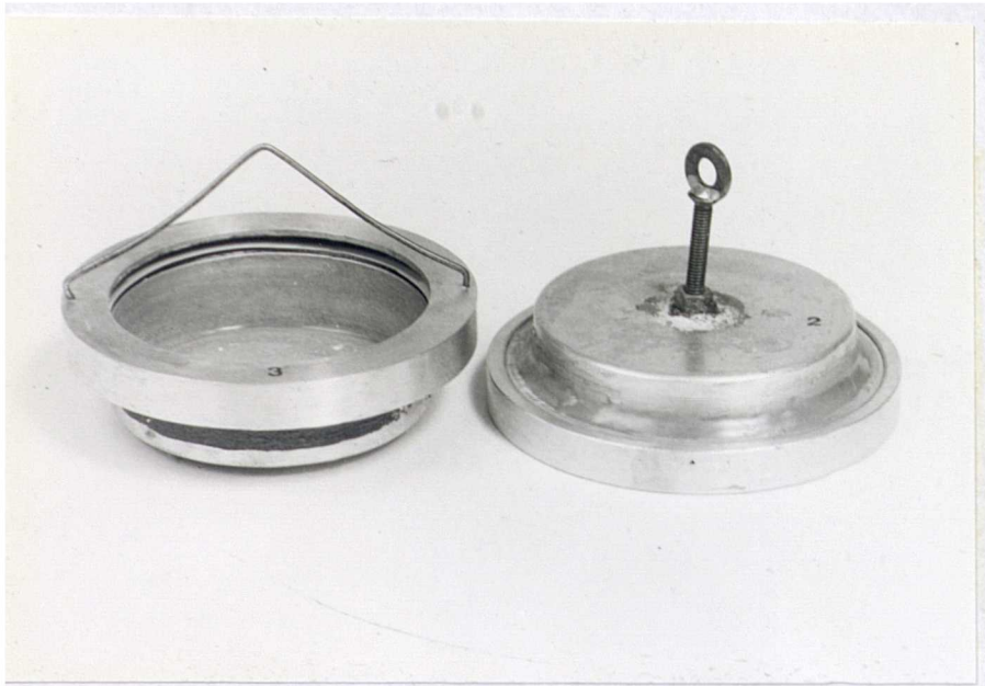
Figure 8.10a The test cell used in the experiments to determine the water vapour transmission rate of silicone gel.
