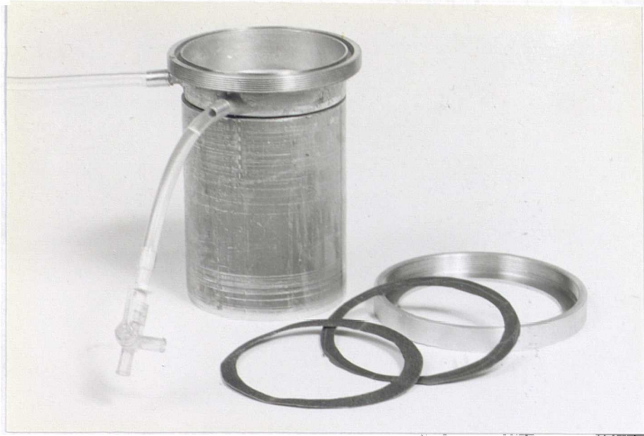
Figure 8.4 The test cell used in experiments to determine the conformability of silicone gel.
