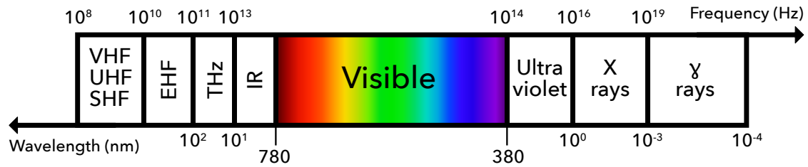
Figure 1.6: Electromagnetic spectrum in logarithmic scale for frequency and wavelength. The visible range is enlarged and is not to scale.
