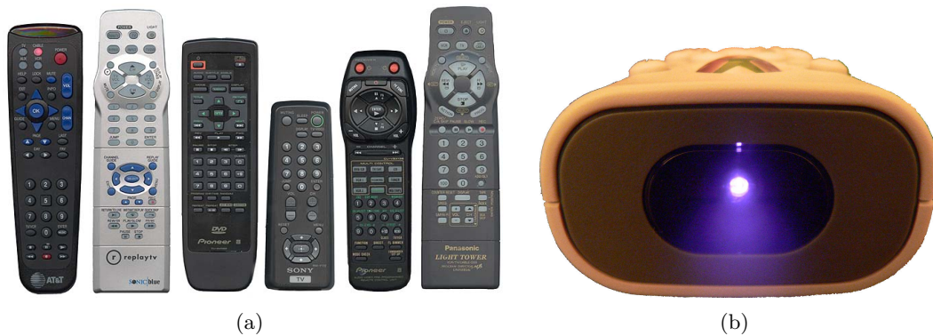
Figure 1.3: Examples of IrDA transmitting devices, (a) domestic remote controls and (b) emission from a remote control detected by an image sensor. From Wikimedia with free licence.
