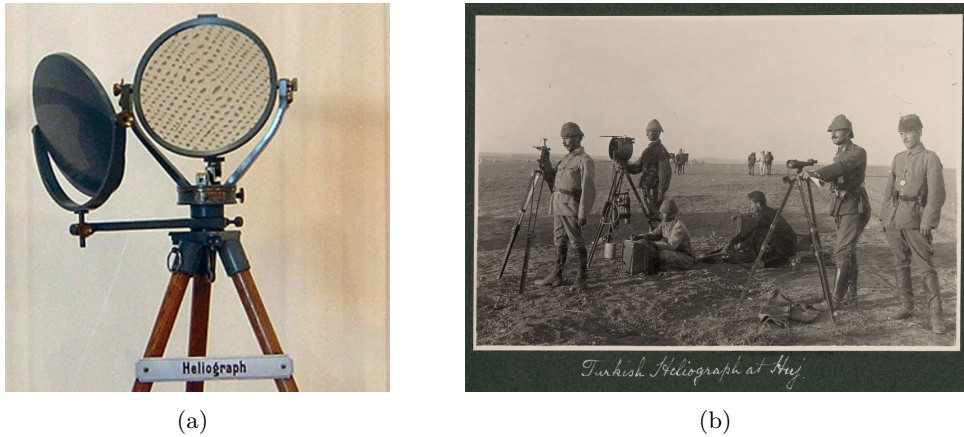
Figure 1.2: Examples of heliographs: (a) German built system and (b) Ottoman heliograph crew at Huj during World War I, 1917. From Wikimedia with free licence.
