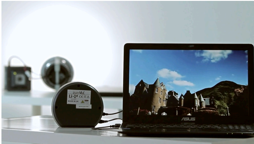
Figure 1.9: First LiFi commercial system by the UK company pureLiFi, the Li-1 st , a full-duplex VLC system. A video is being communicated wirelessly over free-space between source and detector using reflected light. Picture taken from [4].
