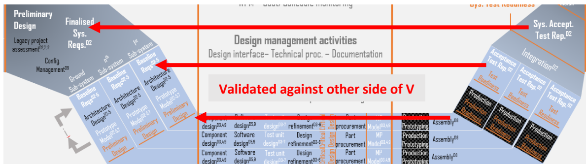
Figure 7-6 – Cross-referencing requirements when validating
