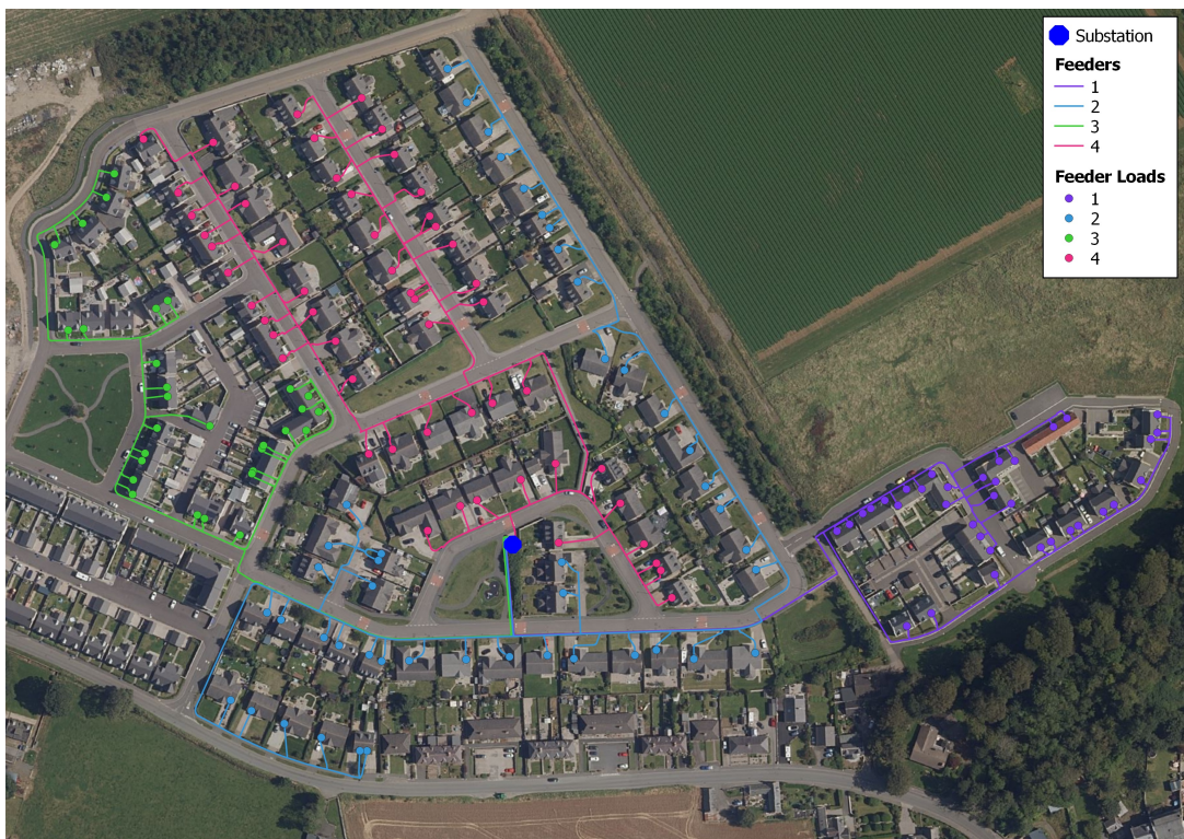
Figure 5.11. Satellite visualisation of the LV distribution network under study using Bing Aerial showing which households are connected to which of the four network feeders in the area that are connected to the substation shown. Copyright statement: © 2023 Microsoft, Microsoft product screen shot(s) reprinted with permission from Microsoft Corporation.
