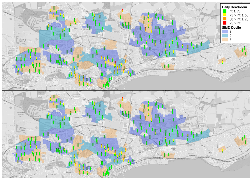
Figure 3.17. Comparison of the generalised and localised approaches in more socially deprived areas (SIMD deciles 1, 2 and 3) at 100% HP penetration. (top) Generalised. (bottom) Localised.
