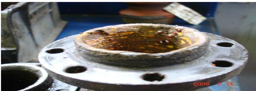
Fig. 1.3: Erosion-corrosion of a joint.
