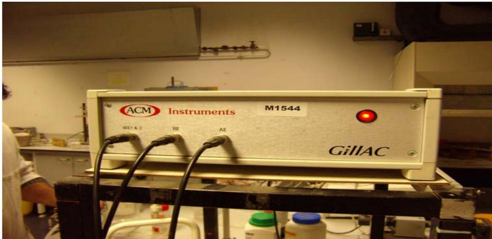
Fig. 2.9: Electrochemical interface with three electrodes ACM (Gillac).
