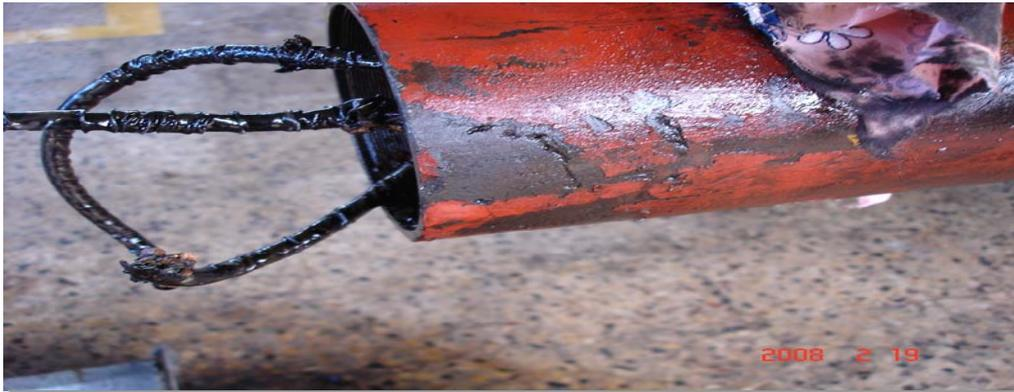
Fig. 1.1: ESP destroyed by erosion–corrosion.
