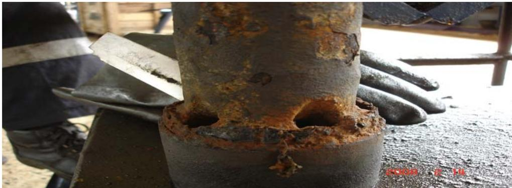
Fig. 1.2: Erosion-corrosion of carbon steel tubing.
