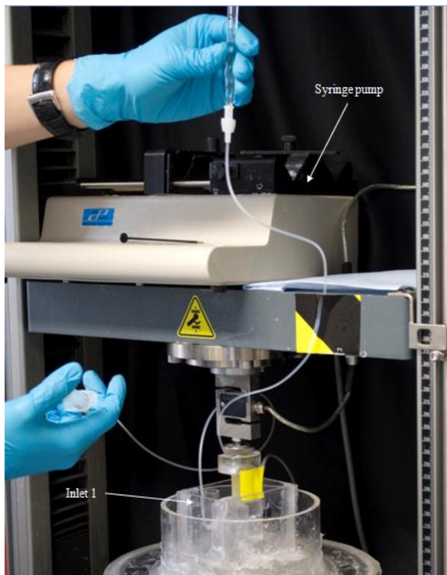
Figure 3.4 Filling the upper chamber with solution, and venting air out through syringe.
