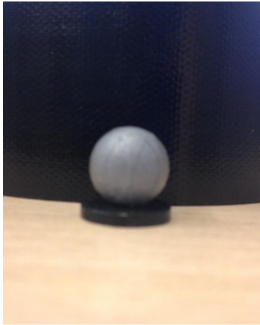
Figure 7 14mm reflective marker
