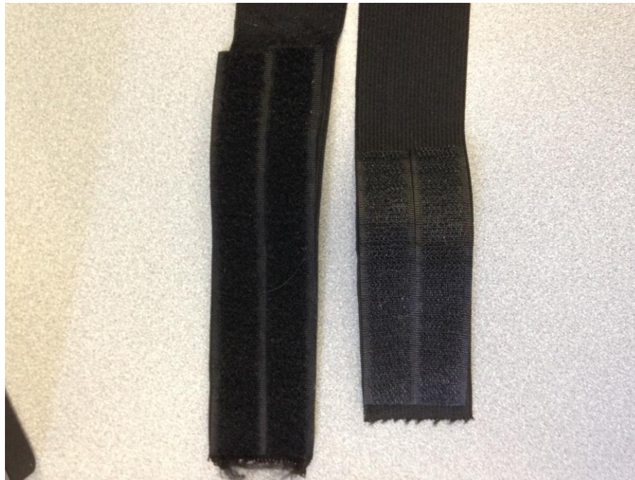
Figure 4 Assembly of elastic and velcro used to attach cluster to participants
