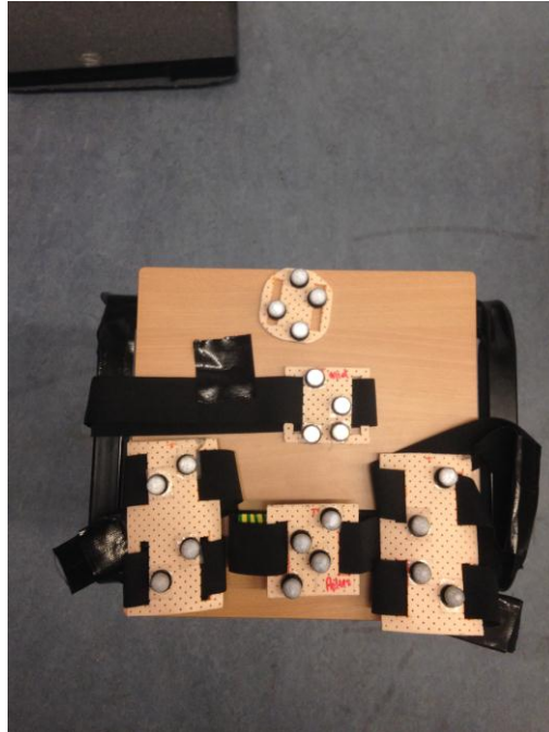
Figure 10 Configuration of clusters used in the bench test
