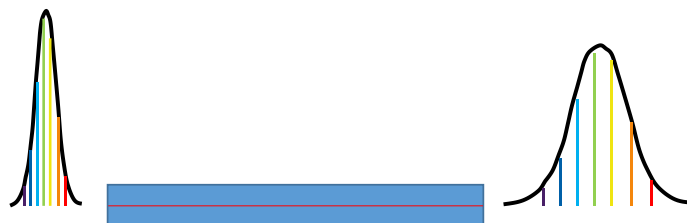
Fig. 3.1: Optical pulse broadening.
