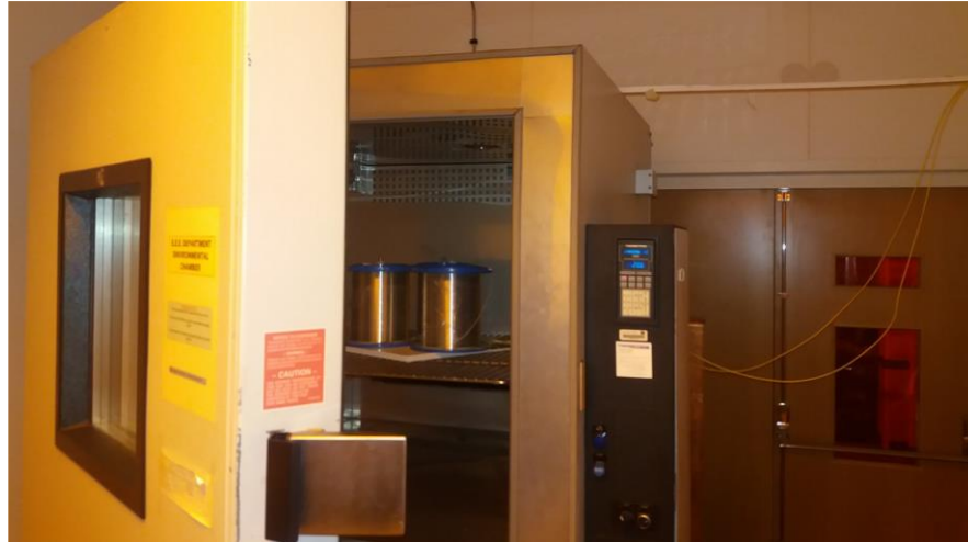
Fig. 5.3: Fibre spools placed in the temperature control chamber.
