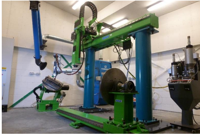
Figure 35 LMD processing cell.
