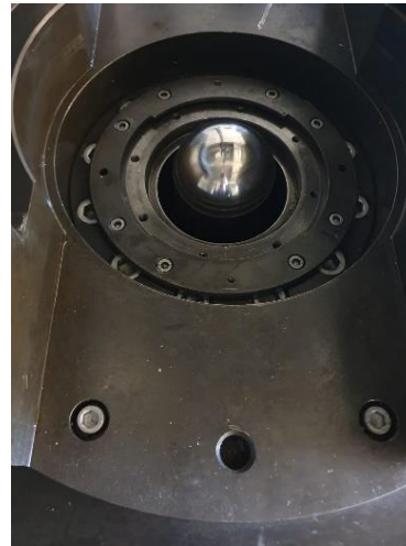
Figure 119 Nakajima test setup: (a) BUP machine; (b) Hemispherical punch.
