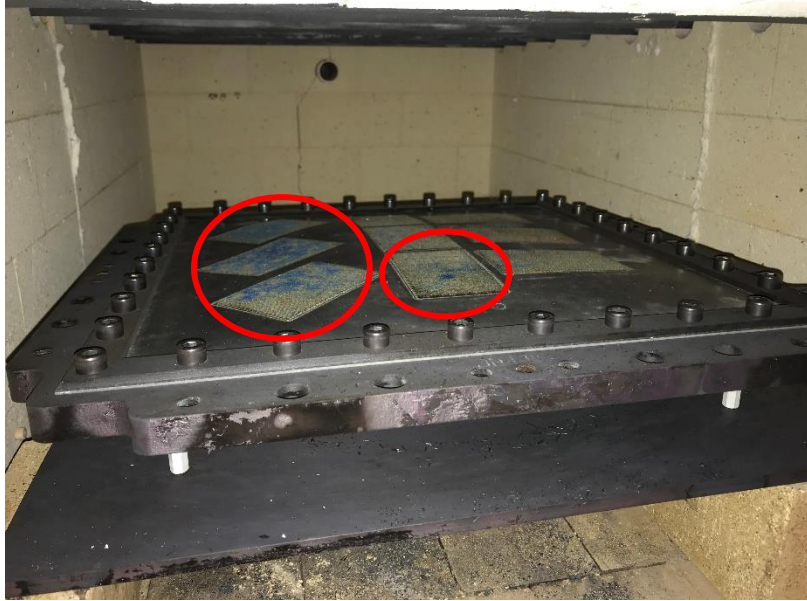
Figure 59 Blue oxide surface following heat treatment.
