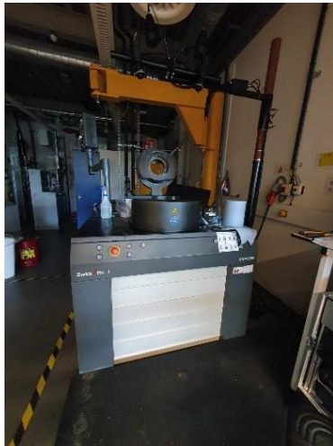
Figure 119 Nakajima test setup: (a) BUP machine; (b) Hemispherical punch.
