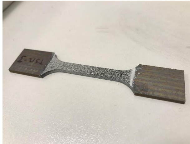
Figure 40 Stochastic (speckle) pattern on tensile specimen for DIC.
