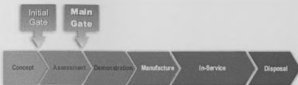
Figure 1.1: The CADMID Cycle Source: MOD, The Acquisition Handbook, 2002
