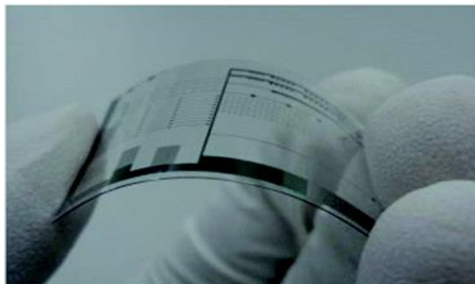
Figure 1.1: Flexible AMOLED display on PEN substrate [1].
