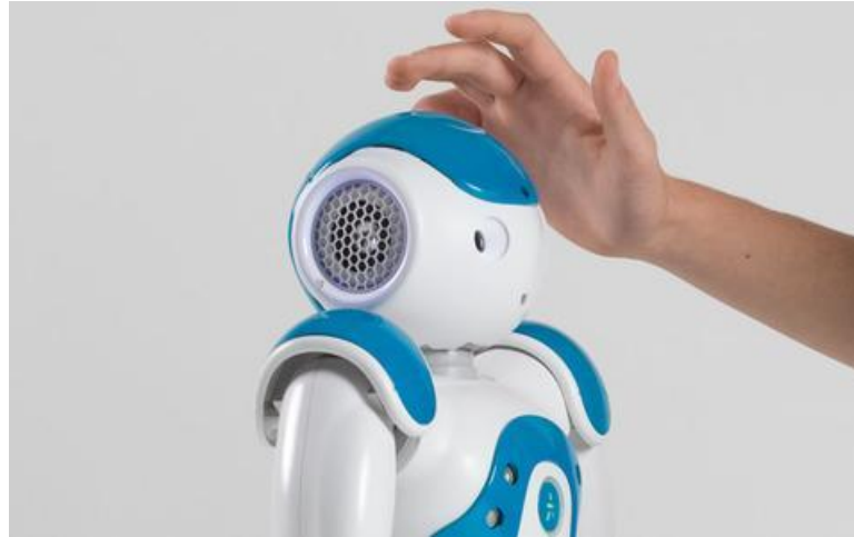
Figure 1.4: Humanoid robot fitted with capacitive tactile sensors for touch detection [10].
