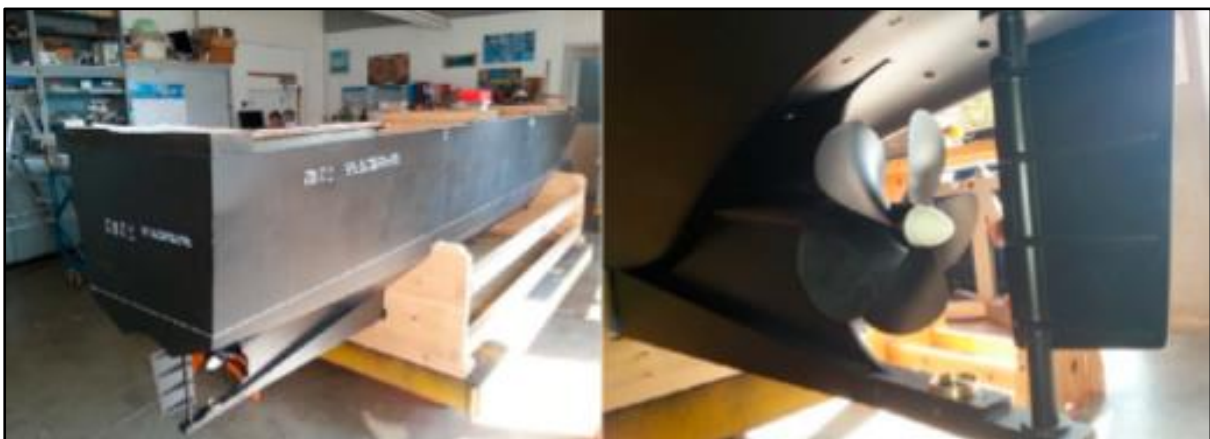
Figure 6.31. Model scale vessel tested in the cavitation tunnel (Felli et al., 2014).
