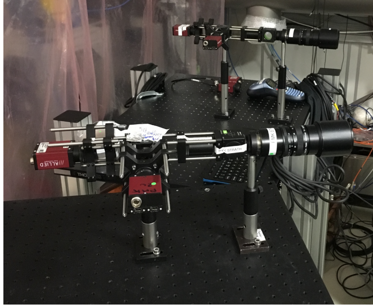
Figure 4.5: Photograph of the dual-wavelength imaging system employed to measure the light signal incident on the scatter screens.
