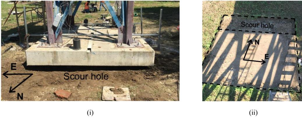
Figure 5-5: (i) Excavation of the soil under the foundation, (ii) Scour hole shape at the end of the final test.
