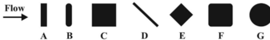
Figure 2-4: Cylinders differing in cross-sections shape, but having the same projected width to the flow [37],[38].
