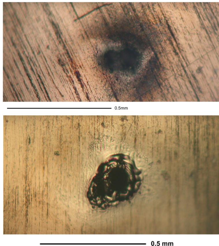
**Figure 7.11.** Damaged areas in the molybdenum foil used in the scintillator experiments.
