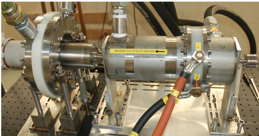
**Figure 6.13.** Photo of the constructed solenoids with water hoses, power connections and 3-axis mounting system.
