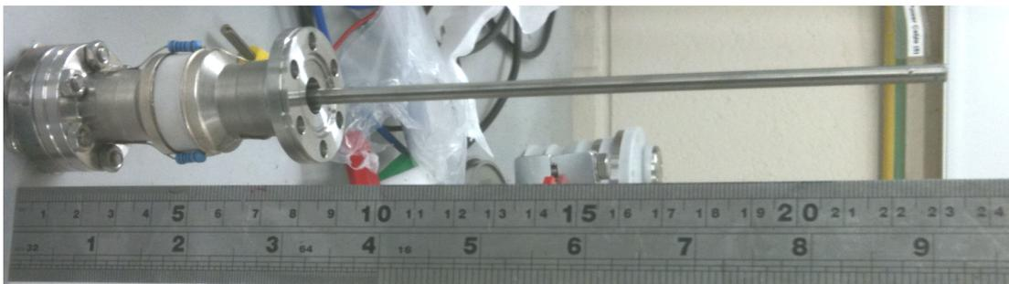
**Figure 6.42.** Photo of the Faraday cup connected to a ceramic insulator which has two 100Ω resistors connecting the two sides of the ceramic insulator.
