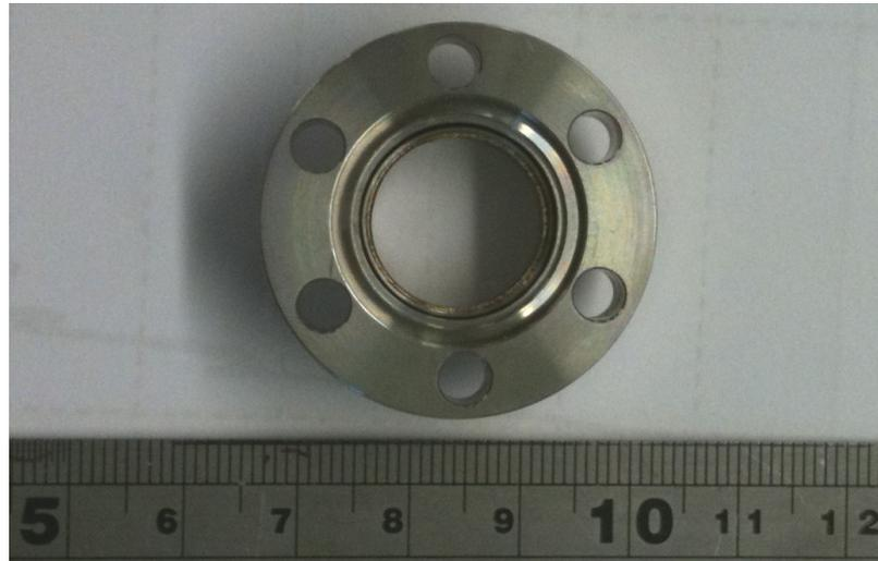
**Figure 6.20.** Photo of the microwave window used in the W-band gyrotron backward wave oscillator system.
