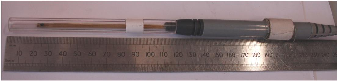
**Figure 6.16.** Axial hall probe used to measure the cavity and reverse coil's magnetic field profile.
