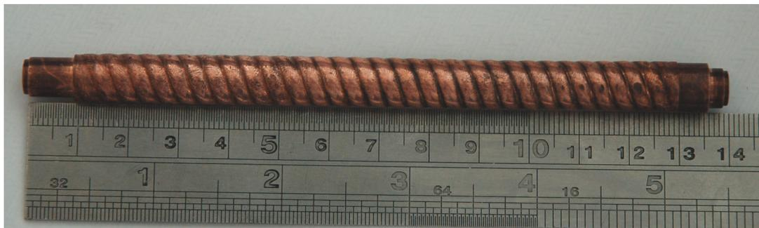
**Figure 3.19.** Photo of the constructed 34-period helically corrugated waveguide.
