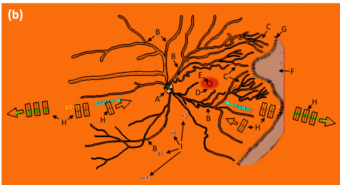
Figure 89 - A flat retinal target with 3 dimensional features (b) was created by tracing appropriate 3D shapes over a reference image taken from Gole et al. that is used as a reference for stage 2 ROP (a) (359). Certain features guided painting of the retina, such as an extrusion of the optic disc (A), and embossed features representing major blood vessels (B) and neovascularisation (C). Others sought to emulate three-dimensional features of a preterm ocular fundus such as the foveal pit (E) within the macula (D) and the retinal ridge (G) at the edge of a region of detached retina (H). Finally, extrusions were also added to mark the various retinal zones (H) and subtended angles between 30^\circ and 75^\circ in 15^\circ increments.
