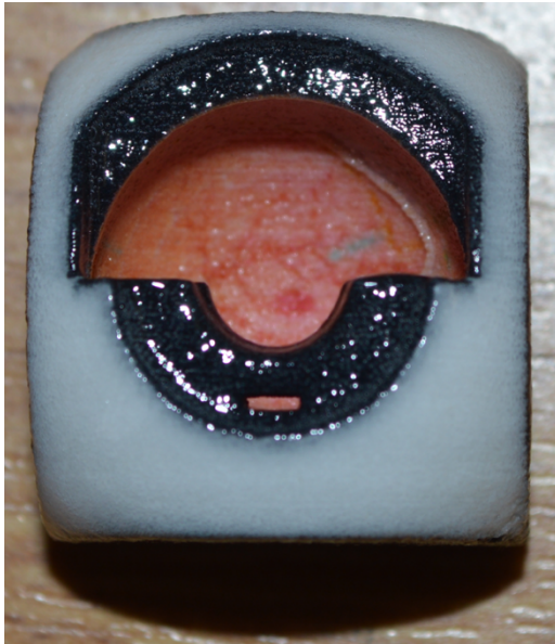
Figure 90 - A rejected prototype of the eye phantom using coloured sandstone.
