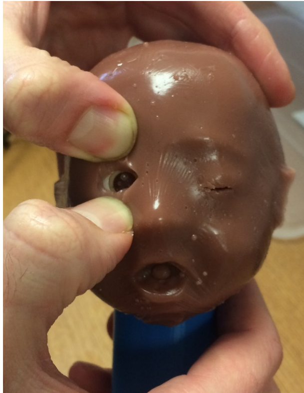
Figure 100 - Fully assembled preterm infant phantom. Eye phantom is inserted in the position of the right eye with a 3D printed 'blank' being inserted in place of the left eye.
