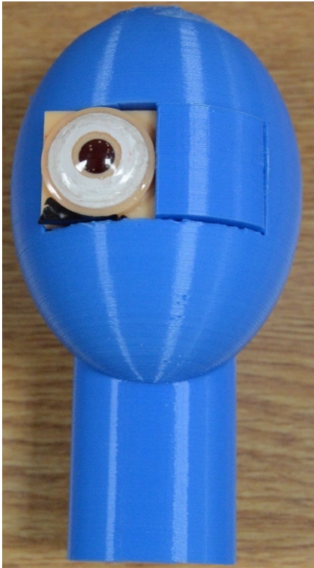
Figure 97 - Skull phantom with eye phantom inserted in the position of the right eye and a blank inserted in the position of the left.
