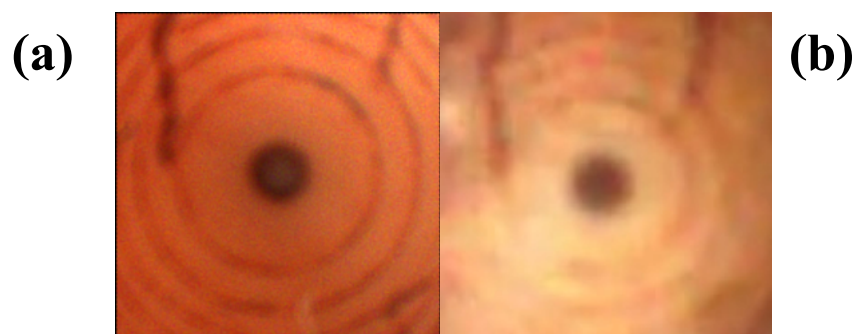
Figure 131 - Region of interest containing the foveal pit and three radial steps resulting from the additive 3D printing process acquired using (a) the RetCam (b) the prototype.
