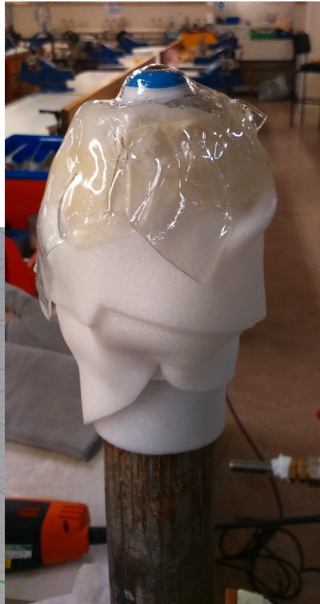
Figure 94 – Left: A CAD rendering of the vacuum mould, consisting of a 3D printed part, in blue, and a 12mm diameter steel ball bearing in grey. Right: The PMMA meniscus lens representing the cornea in the eye phantom was formed by heating the PMMA sheet in an oven and then pulling over the mould that was sealed on top of a vacuum pipe.
