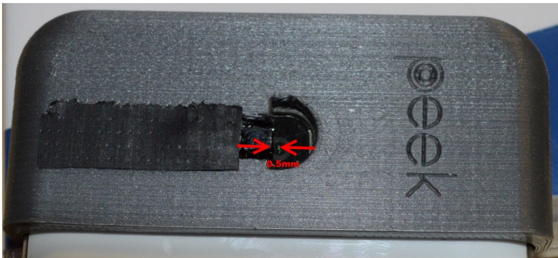
Figure 42 - The prism was fixed so that there was an approximately 0.5mm lateral separation from the camera aperture.
