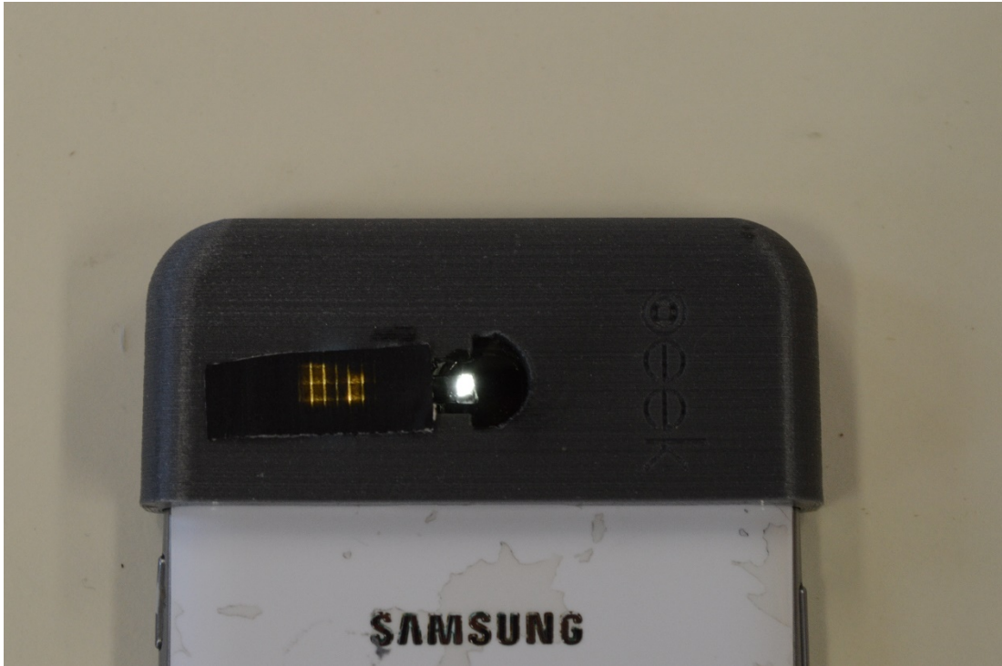
Figure 43 - A length of black duct-tape was fixed over the prism channel to prevent light not entering the prism from causing unpolarised specular reflections and therefore image artefacts.
