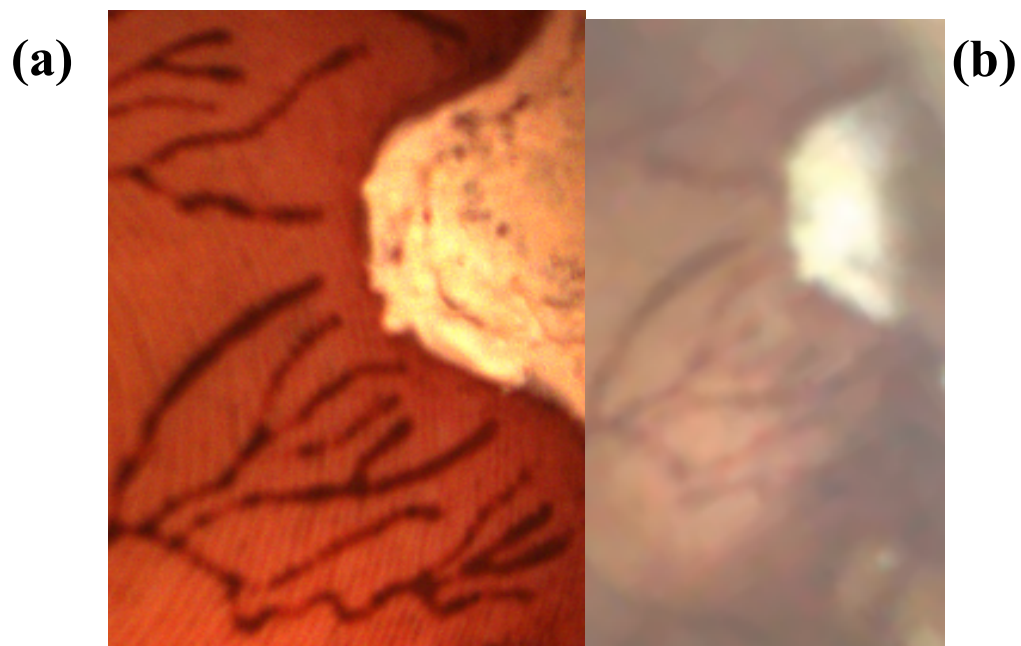
Figure 130 - Comparison of the resolution of finer details on the preterm eye phantom as acquired by a RetCam 3 (a) and the technology demonstrator (b)
