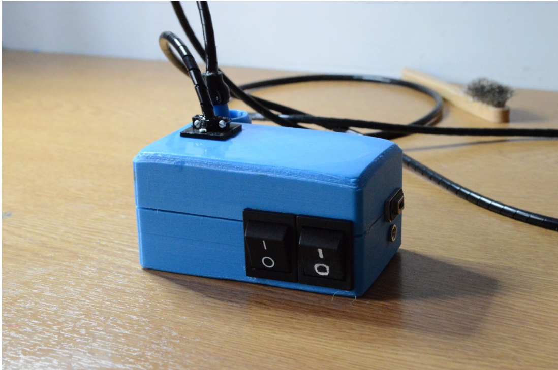
Figure 115 – The fully assembled base unit. The rocker switch to the left of the front face controls the illumination source. The camera grip is stored in the receptacle to the right and rear of the unit.
