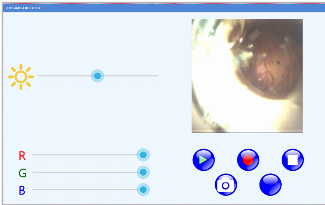
Figure 119 - Screenshot of the system GUI. The GUI also allows control of the image sensor's exposure (top left) and the setting of the gain of each colour individually (bottom left). Every other image sensor setting is set automatically in software.
