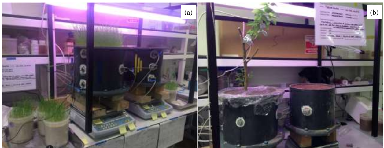
Figure 5.1: Infiltration column, vegetated and bare soil; (a) Herbaceous species: Lolium Perenne ; (b) Shrub: Salix Cinerea
