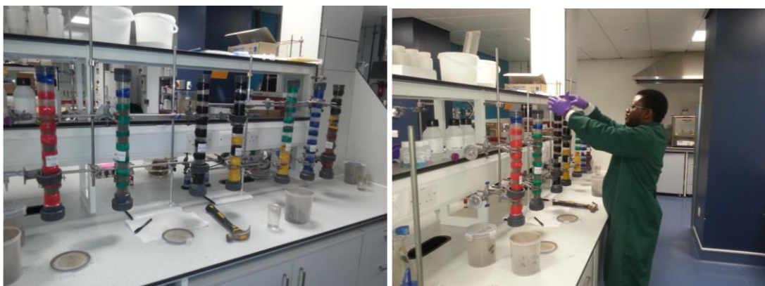
Figure 5.2 Columns used and addition of amended soil into the columns
