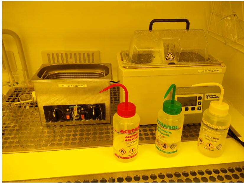
**Figure 2.2:** The ultrasonic cleaner and solvent bench.
