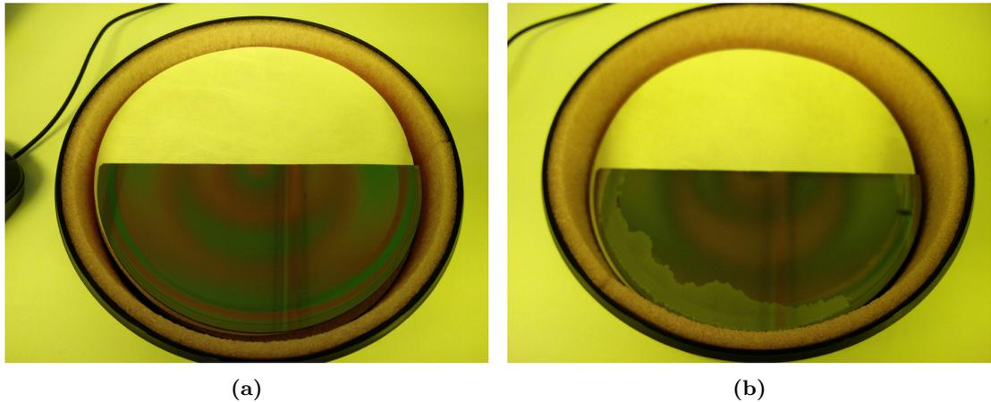
**Figure 5.1:** (a) The 5 layer DBR wafer material and (b) the 10 layer DBR wafer material as received from the Cambridge collaborators. The 10 layer structure showing clear delamination and flaking due to the stresses of growth shattering the GaN DBR layers. The wafers are each 150 mm in diameter.
