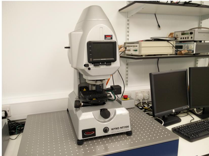
**Figure 2.35:** The Wyko NT1100 optical profiling system.
