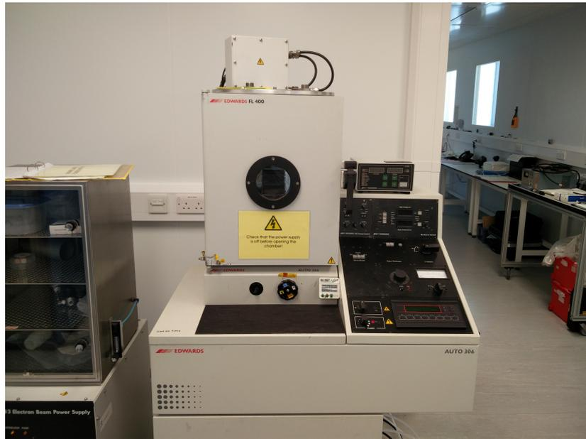
**Figure 2.23:** The E-beam evaporator used for thin metal film deposition.
