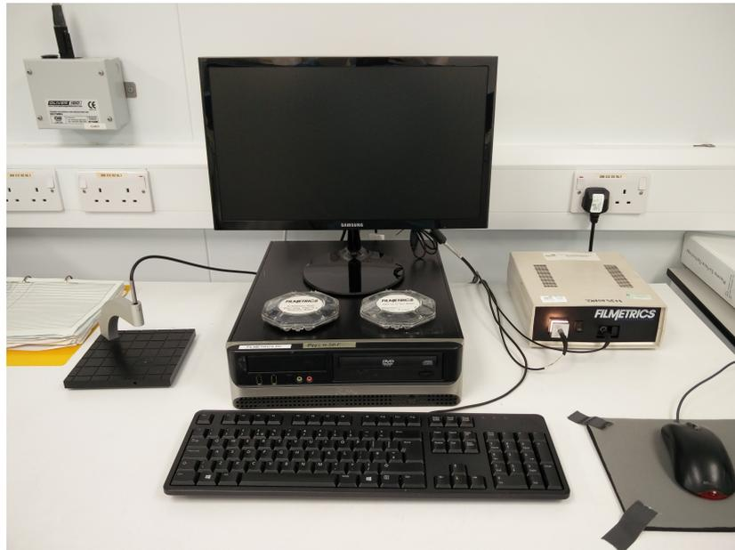
**Figure 2.33:** The Filmetrics F20 thin film measurement device.
