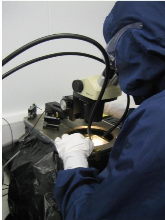
**Figure 2.38:** The probe station tool.
