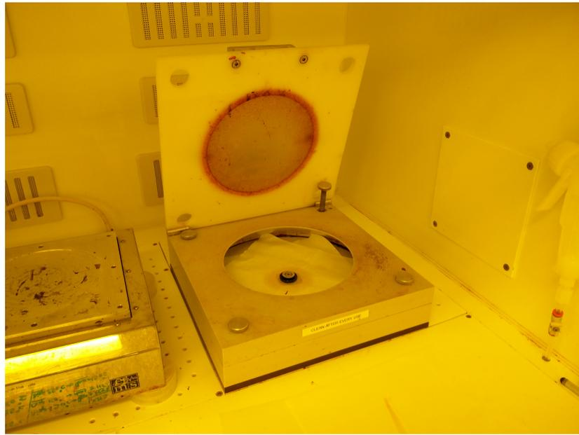
**Figure 2.9:** The photoresist spinner lined with cleanroom wipes ready to spin a sample.
