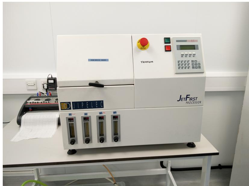
**Figure 2.24:** The rapid thermal annealing tool.
