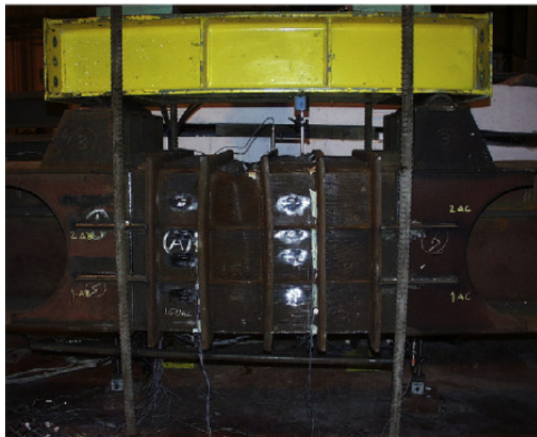
Figure 2-7: General deformation of box girder of high tensile steel after the collapse load, Gordo and Soares (2009)
