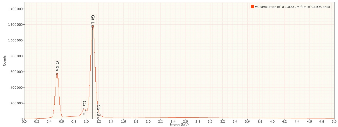
Figure 3.15: EDX X-ray spectra produced by a DTSA-II simulation on 1 \mu\text{m} \text{Ga}_2\text{O}_3/\text{Si} thin film using an electron beam energy of 10 keV and probe dose of 4000As
