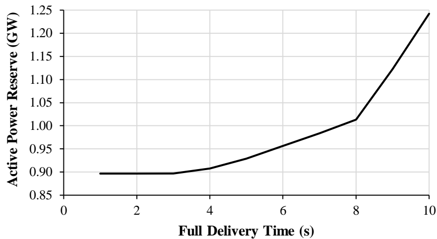
Figure 4.9: Plot of the change in active power reserve held with change in full delivery time of response under the assumed system conditions.
