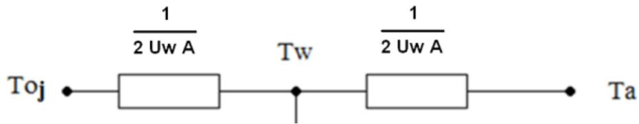
**Figure 63 Steady state resistance circuit of the wall**
