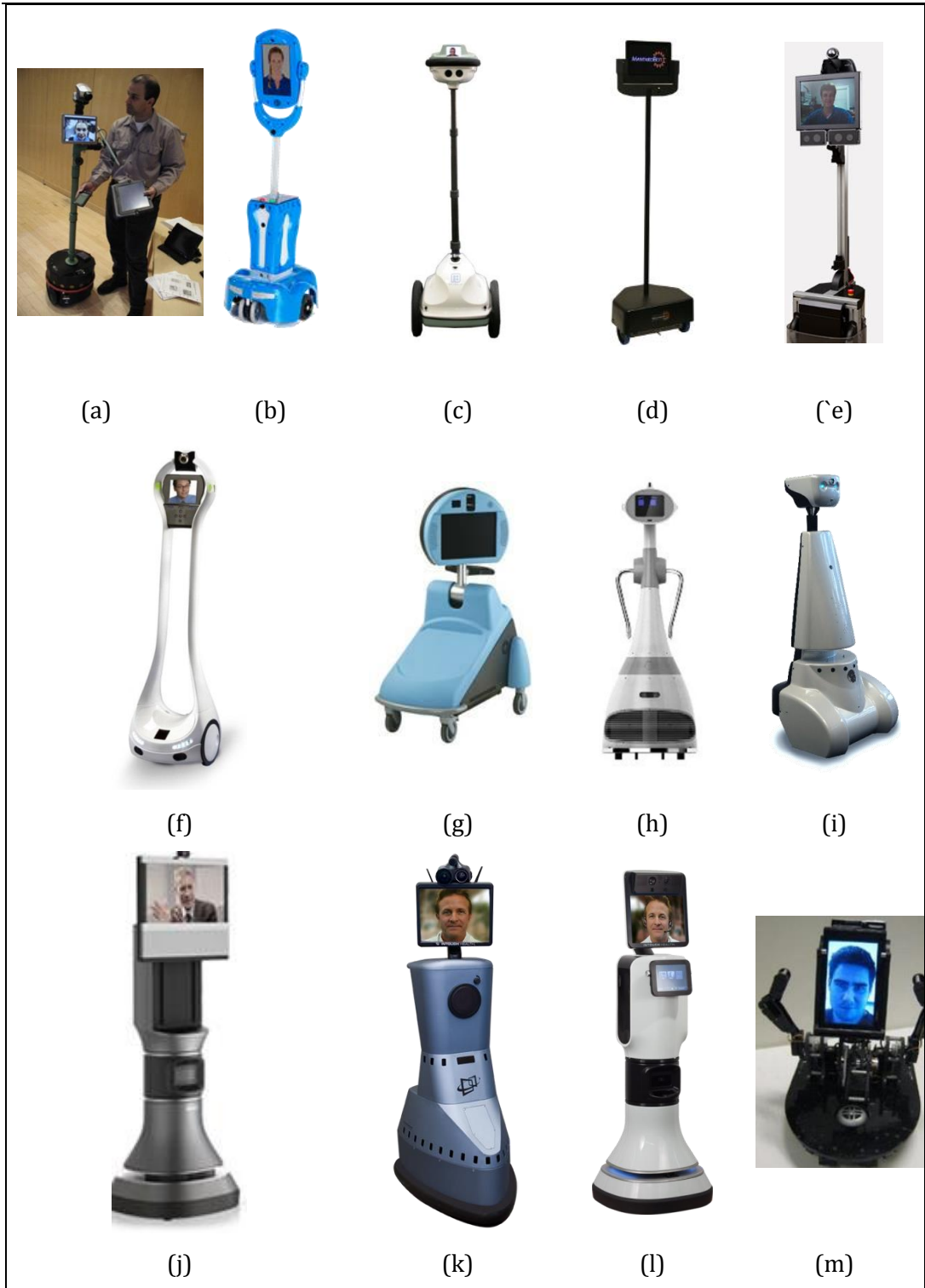
Figure 2.1. (a) PRoP, (b) Giraff, (c) QB, (d) MantaroBot, (e) Texai, (f) VGo, (g) PEBBLES, (h) Luna, (i) Jazz connect, (j) iRobot Ava, (k) RP-7, (l) RP-VITA, (m) MeBot
