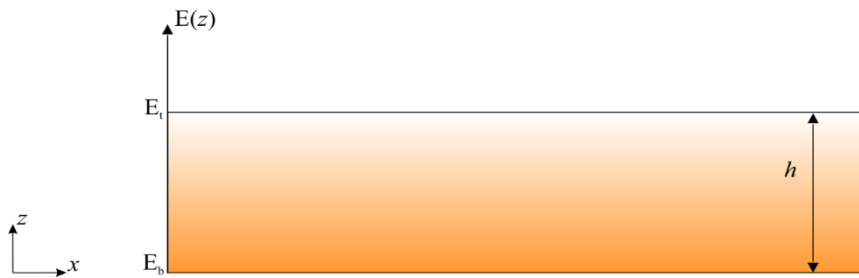
Figure 4.29 Material variation along the thickness direction for the functionally graded material
