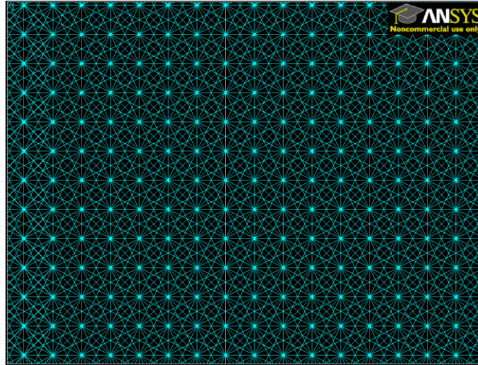
Figure 6.5 Network of beam elements to represent interactions between PD points.
