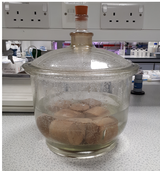
Figure 3.2: Vacuum saturation in progress
