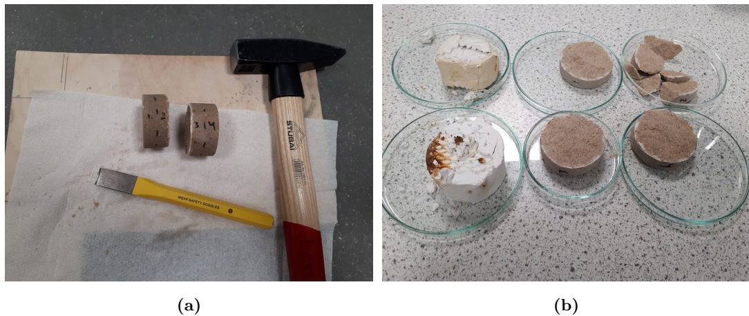
Figure 7.3: Preparation of samples for analysis. (a) Using hammer and chisel to segment samples. (b) Measuring water content on stone slices and poultice.
