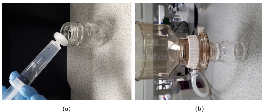
Figure 3.8: Filtering systems (a) by hand (b) using vacuum
