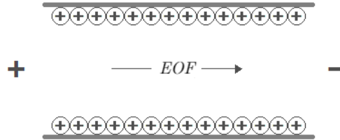
Figure 2.5: Positively charged electrical double layer on the inner surface of a negatively charged capillary, resulting in an electroosmotic flow (EOF) towards the cathode, after Dziubakiewicz and Busewski [2013].
