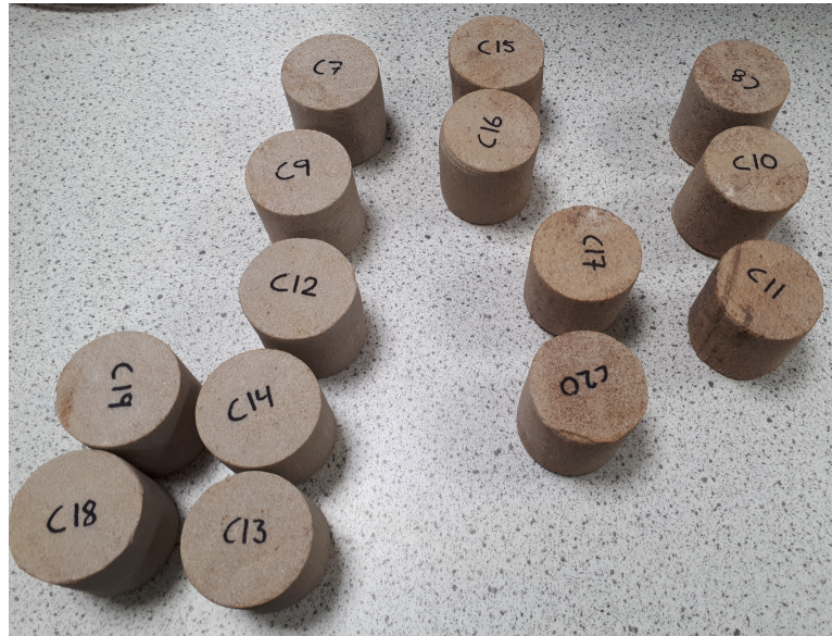
Figure 6.1: Clashach samples divided into sub-groups based on their visual assessment of the amount of iron-stained bands
