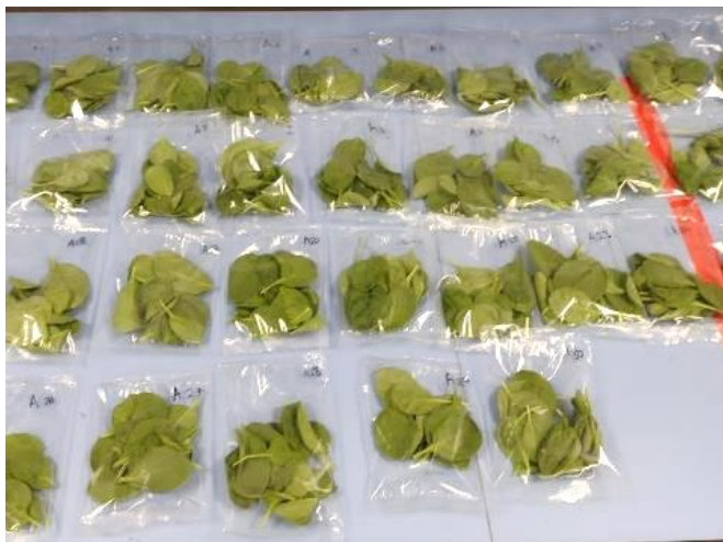
Figure 5.2: Image of packed salad bags. 10 cm x 20 cm bags were produced using BOPP sheets and filled with 10 g of spinach leaves obtained from a local supplier.
