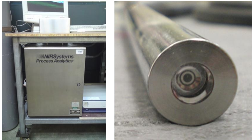
Figure 3.7 – The trolley mounted FOSS on-line 6500 (left) and the reflectance probe head (right).
