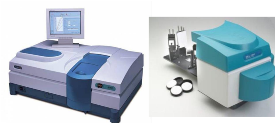
Figure 3.12 – Cary 5000 UV-Visible-NIR (left) spectrometer and external diffuse reflectance accessory DRA 2500 (right) 4 .
