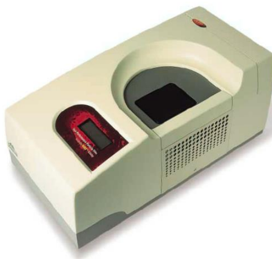
Figure 3.17 – Malvern HPPS 5001 non invasive back scatter particle sizer. 7
