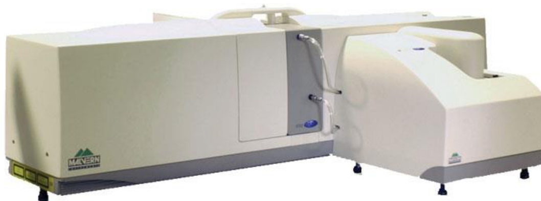
Figure 3.19 – Malvern Mastersizer 2000 with HydroG sample dispersing unit. 9
