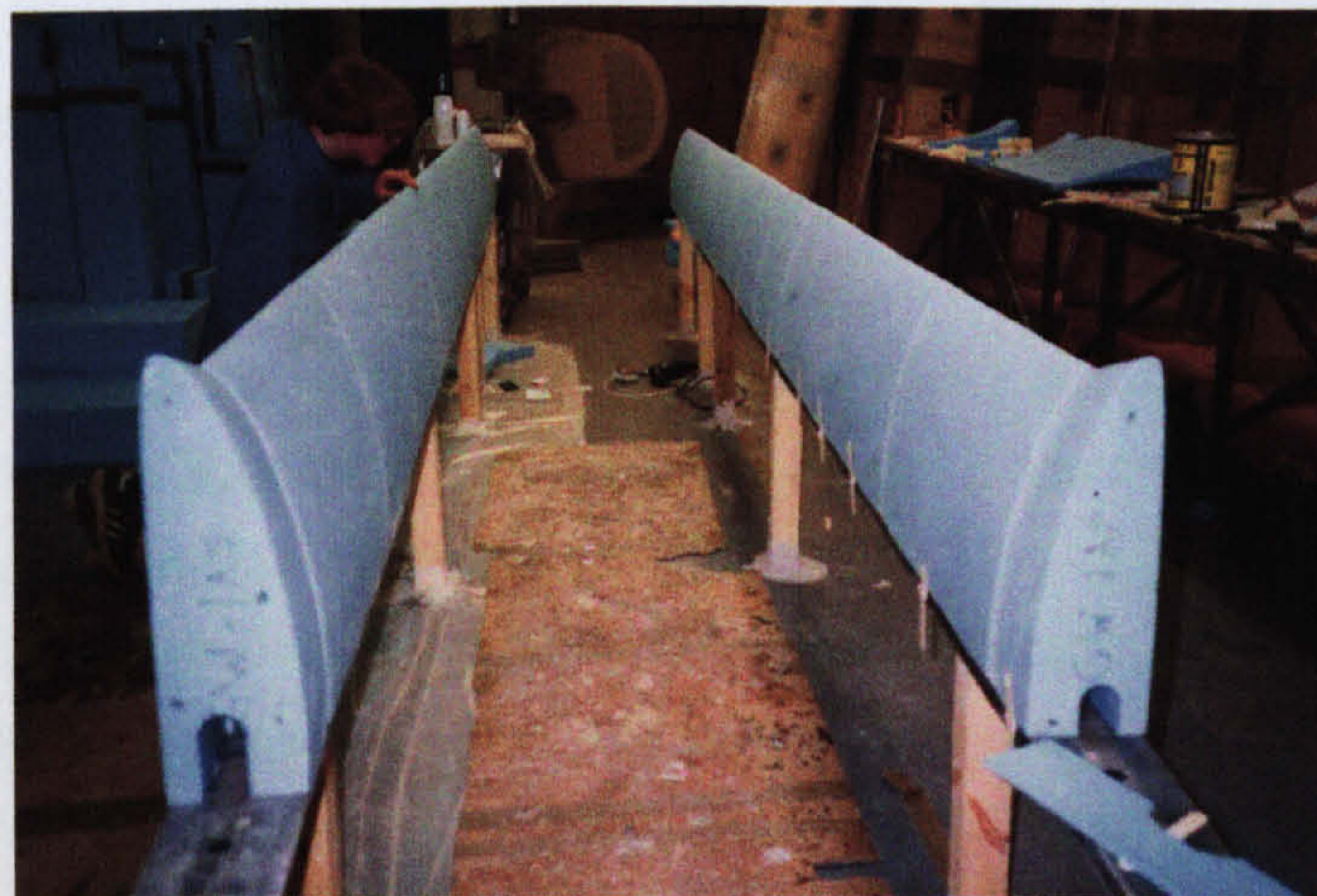
Fig 24: Construction of the Prototype Glider Wing Leading Edge structure
