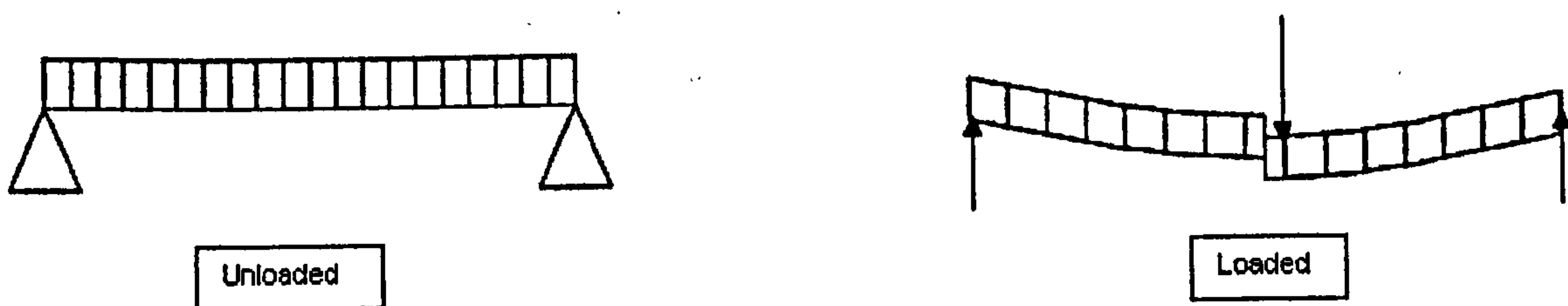
Fig 29: Core Shear failure
