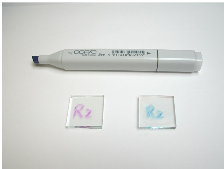
Figure 6-11 – a picture showing the resazuring ink on Activ Glass and plain glass after irradiation with UV light, alongside the pen used to put down the ink.
