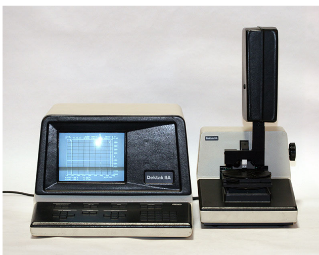
Figure 2-1 – the dektak profilometer used for measuring the thickness of thin polymer films.
