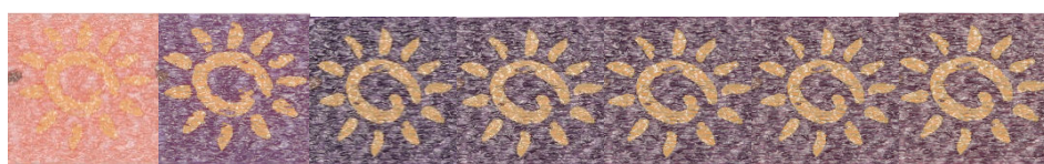
Figure 1-11 – Pictures of the centre of the SolarSafe wristband after irradiation with UVI 5 solar light. The pictures show, in order, the wristband after it has received 0, 1, 2, 3, 4, 5, 6 and 7 MED equivalents for skin type II.
