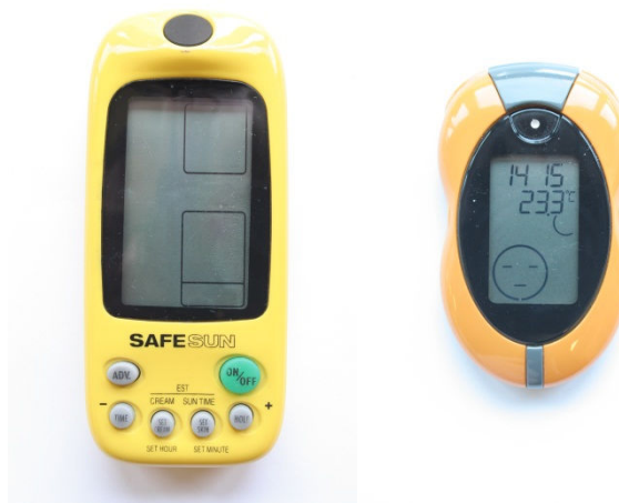
Figure 1-5 – Two example electronic devices for monitoring the levels of solar UV. On the left is the Optix Safe Sun Precision UV Meter, and the right hand instrument is the UV Messgerät of Ideen Welt.
