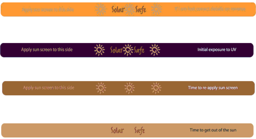
Figure 1-9 – The proposed colour changing scheme of the Solar Safe wristband. The stages are, from top to bottom, pre-exposure to UV, initial exposure to UV, time to re-apply sun screen , and time to get out of the sun .
