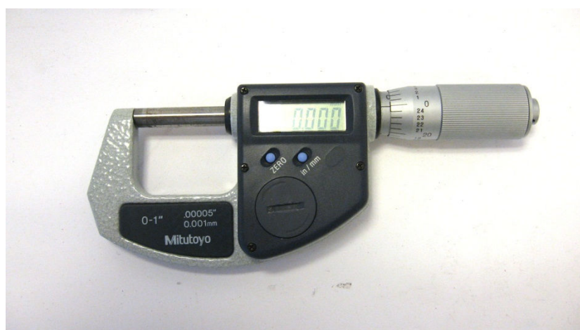
Figure 2-3 – A mitutoyo micrometer, used for measuring the thickness of some polymer films.
