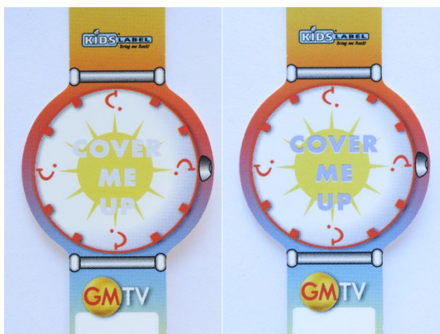
Figure 1-8 – The Kids Label wristband provided to holiday makers by Thomson. These images show the band before and after exposure to UV light. The phrase “cover me up” turns blue upon exposure to high intensity UV.
