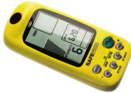
Figure 2-11 – SafeSun Solar Meter used for measuring the UVI index and Erythemal Dose.
