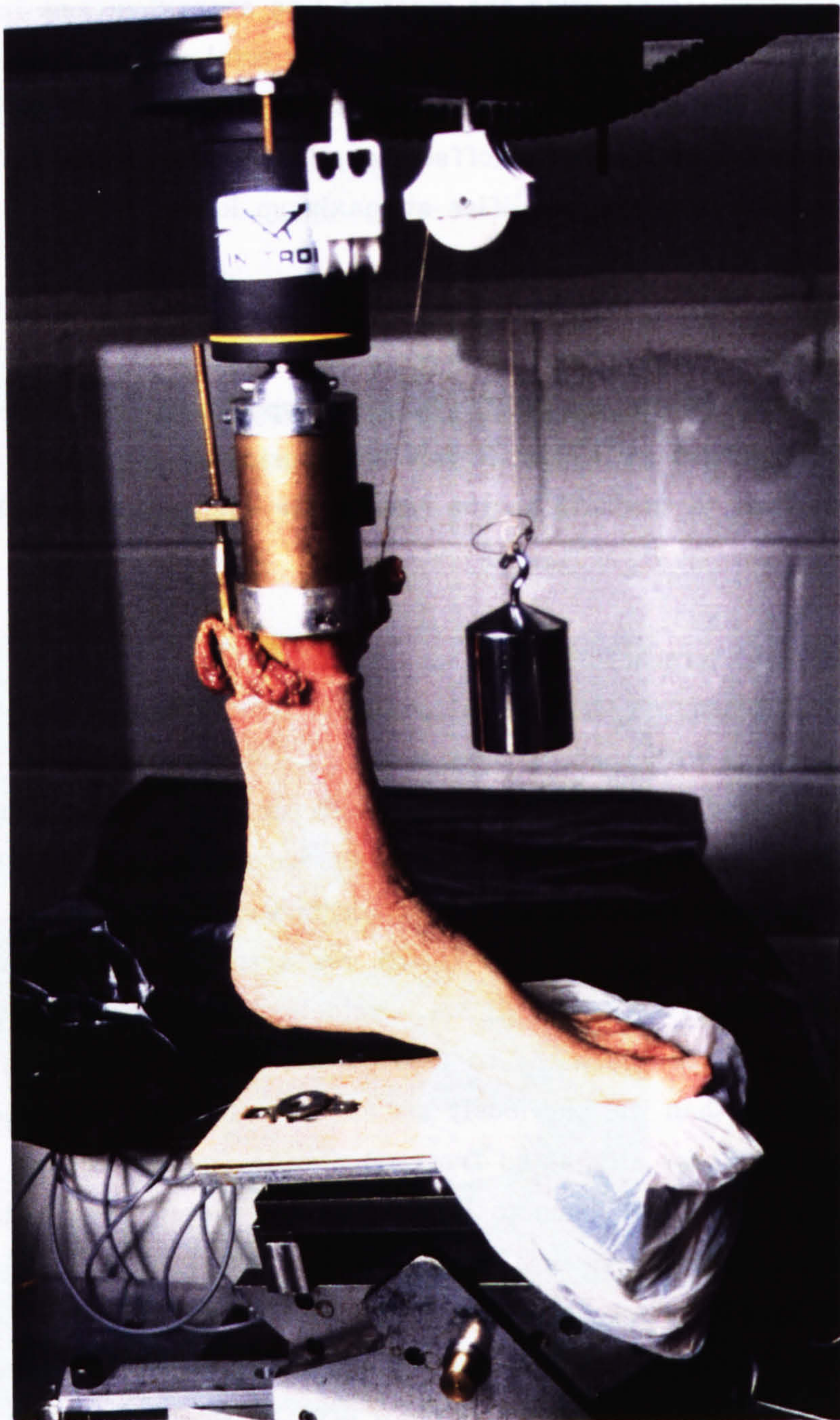
Figure 5.5 A foot specimen mounted in the testing system. The tibia and fibula are fixed in the support collar and the base of the foot rests on the load cells on the support platform. In this case tendo achilles is tensioned to produce plantarflexion and a weight has been added to produce tension in one of the extrinsic muscle tendons. (The plastic cover is removed for the illustration)
