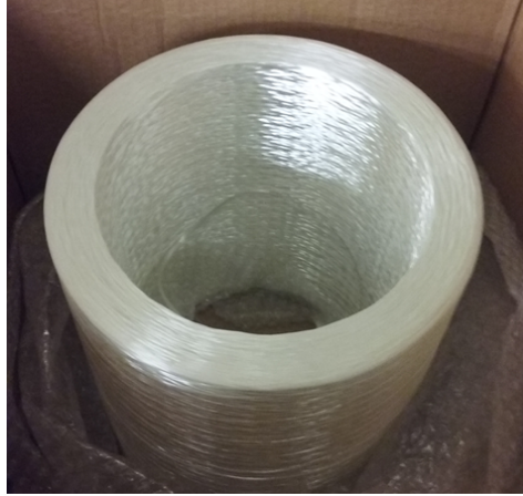
Figure 3.11 – Image of an OC APS-sized E-glass fibre roving
