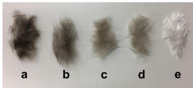
Figure 5.6 - Glass fibres recycled in the fluidised bed at a temperature of a) 400 °C, b) 450 °C, c) 500 °C, d) 550 °C and e) 500 °C + thermal cleaning. Reproduced from [66]
