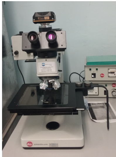
Figure 3.14 – Image of the Leitz Ergolux optical microscope used for measuring fibre diameters before tensile testing
