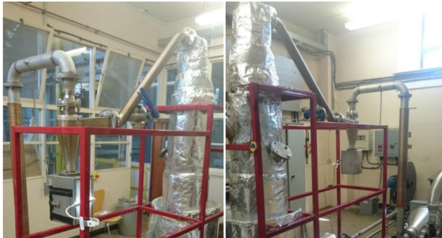
Figure 5.5 – Images of the in-house developed fluidised bed. Reproduced from [66]
