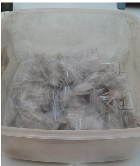
Figure 5.17 – Image of glass fibres thermally recycled from wind turbine blade in the fluidised bed
