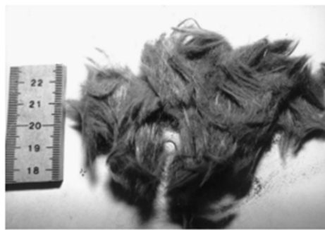
Figure 5.3 – Image of glass fibres recovered from SMC feed using the fluidised bed. Reproduced from [141]
