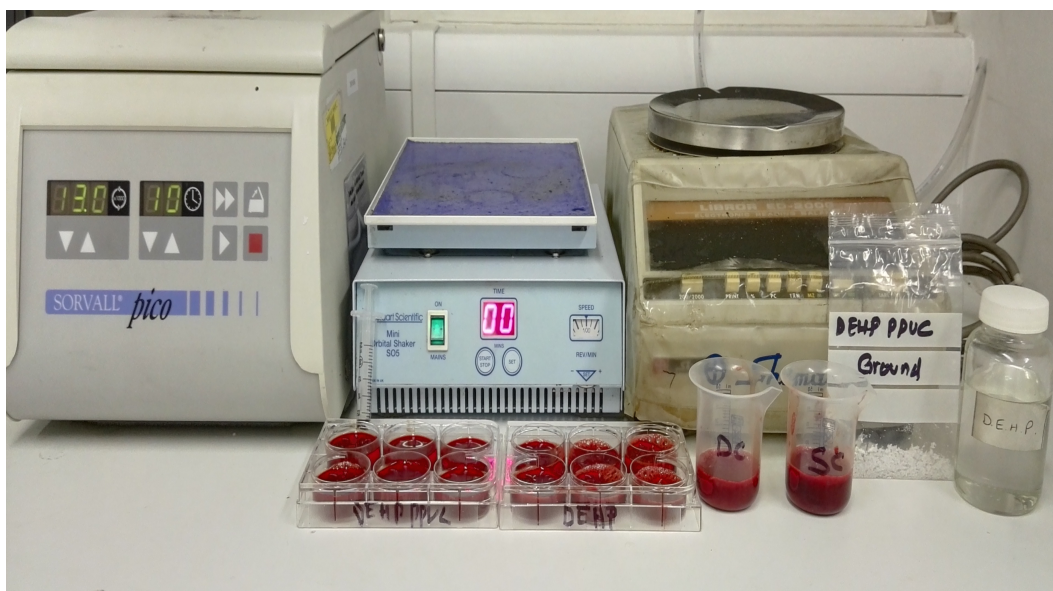
Figure 28: Bovine blood experiment set up from left to right (Centrifuge, orbital shaker, weight balance, liquid DEHP, ground DEHP plasticised PVC and blood samples).
