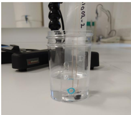
Figure 3.11. pHEMA-adapted electrode submerged in KCl test solution during OCP measurement procedure
