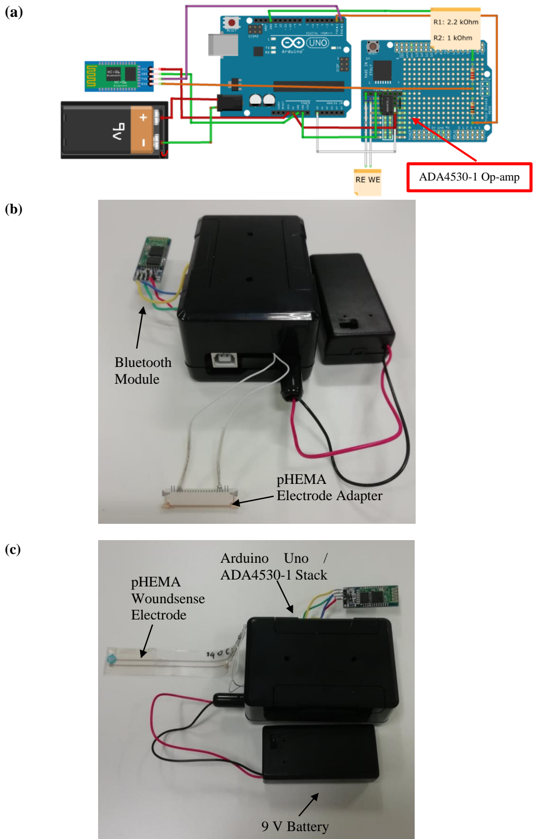
Figure B.2. (a) Schematic of wiring between ADA4530-1, Arduino Uno and HC-06. (b)-(c) Experimental configuration of ADA4530-1, Arduino Uno and HC-06.
