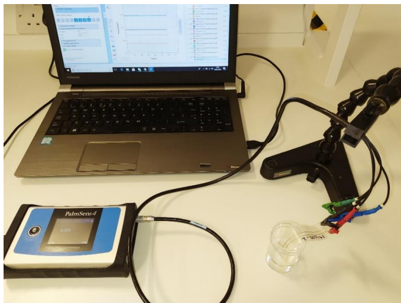
Figure 3.12. Experimental setup utilised for OCP measurement procedure.
