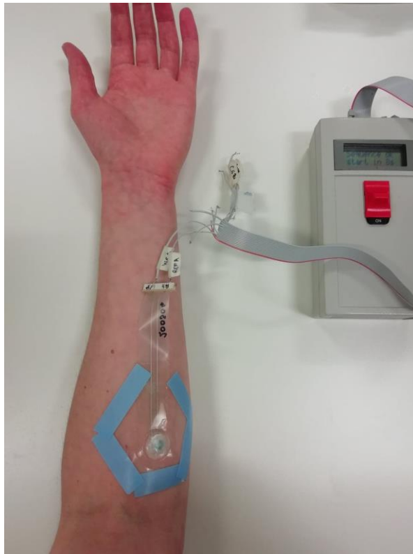
Figure 3.21 Example of how pHEMA electrode with foam is positioned and attached to forearm of participant. The plastic covering was secured over electrode using medium grade toupee tape around its rim. The PEA is shown connected to the electrode.
