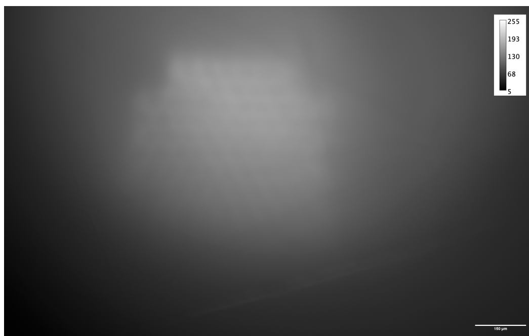
FIGURE 3.10: Inhomogeneity of illumination across a fluorescent slide when using epifluorescence illumination with a reflective objective.
