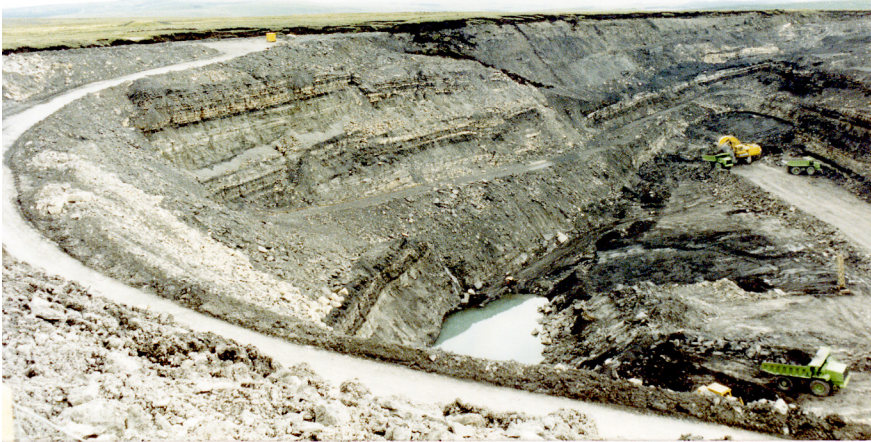
95: Benbain open cast site, 1987 (just north of Dalmellington) showing the digger excavating the coal and dump trucks transporting it away. This image gives a good sense of the relatively few workers that were employed, compared to deep mining.
