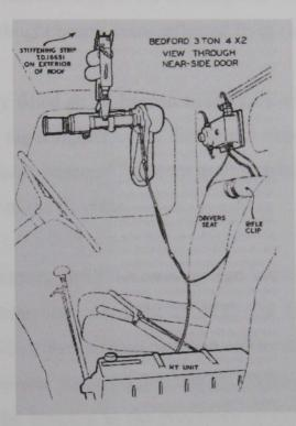
Fig. 4.11 Infra-red binocular installation for British truck Source: Windscreen, spring 2001.
