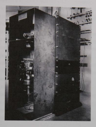
Fig. 6.15 Baird Television Ltd High Speed Facsimile Transmitter, probably from 1937.<sup>4</sup> Source: D. Brown
