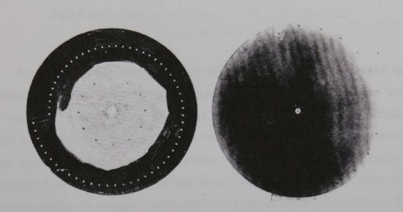
Fig. 3.7 Baird Television LtdFig 3.8 Signals Experimental EstablishmentSource: Television, September 1932.Source: PRO AVIA 23/553Nipkow discs used for sending images of text
