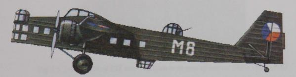
Fig. 6.4 Marcel Bloch 200 aircraft. Unlike the aircraft used by BTL, this aircraft has Czechoslovakian national markings and is fitted with a dorsal and ventral turret.
