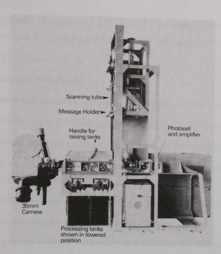
Fig 6.6 The equipment fitted by Baird Television Ltd to Bloch aircraft.
