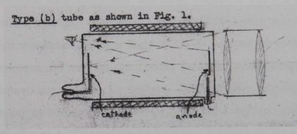
Fig. 4.8 Cassegrain type image converter tube. Source: ADM 204/1432
