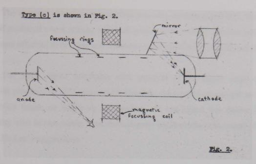
Fig. 4.9 Development of image converter. Note mirror above anode installed to overcome problem of occlusion of image by anode.
