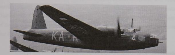
Fig. 6.26 Wellington Mk I fitted with Vickers Turrets Source: Author's collection.
