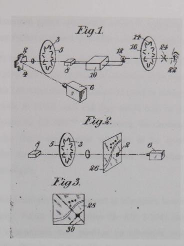
Fig. 3.2. Remote spotting apparatus defined by J.L.Baird's patent GB 295 210 Source: Patent GB 295 210
