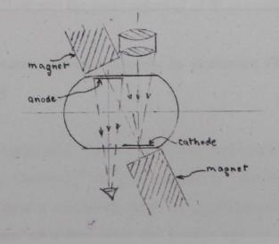
Fig. 4.10 Dr Lee's suggestion for an image converter tube. Source: ADM 204/1432
