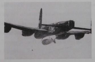
Fig. 7.22 A Grand Slam bomb being dropped from an Avro Lancaster aircraft. Source: J. R. Hills
