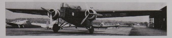
Fig. 6.8 *The MB 200 at Hendon aerodrome*. Note the absence of the ventral turret and single bladed generator fitted below fuselage.
